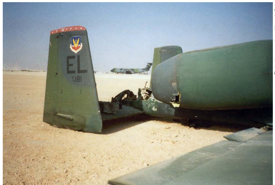
An A-10 shows heavy damage caused by an Iraqi surface-to-air missile during Desert Storm.
