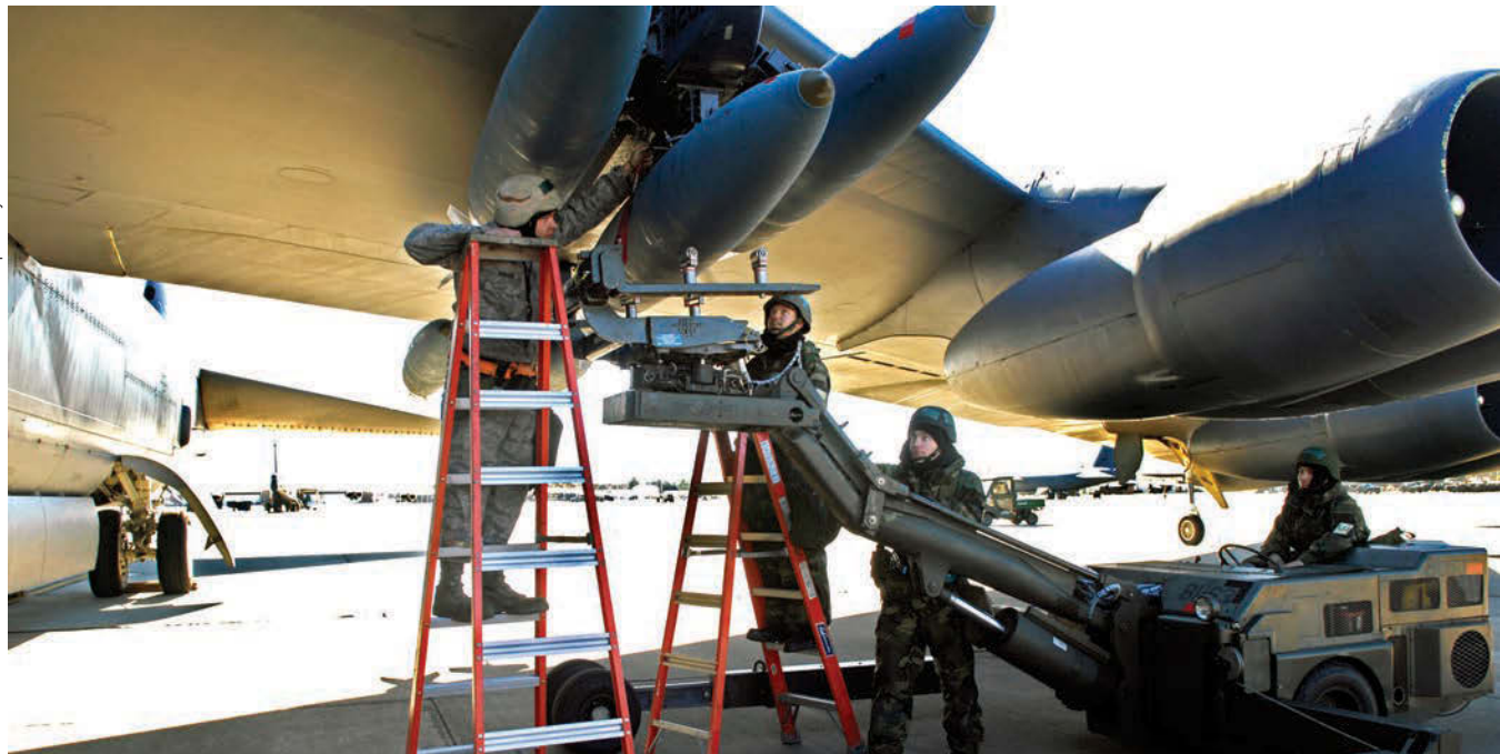
A weapons load team moves JDAMs onto a B-52 at Barksdale AFB, La. One upgrade for the bomber will allow for retargeting of weapons during flight.
