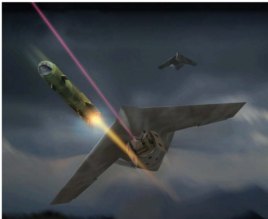
An artist's concept of the Lockheed Martin unmanned aircraft called "Various," which can take off and land vertically, using lift fans in the wings.
