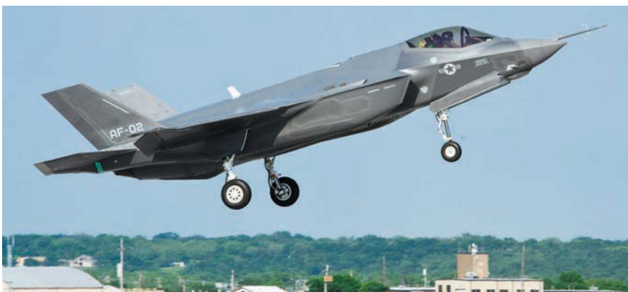
Lucky Seven: The seventh F-35 flight test aircraft takes off on its first flight from NAS Fort Worth JRB, Tex. The aircraft, known as AF-2, is configured to test multiple weapons loads and will be used to test the F-35's ability to carry both internal and external weapons.
