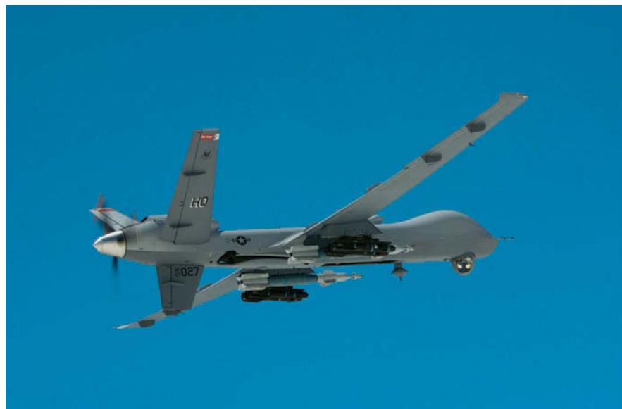
An MQ-9 Reaper armed with laser guided bombs and missiles. The Reaper can carry a payload roughly equivalent to an F-16 fighter.
