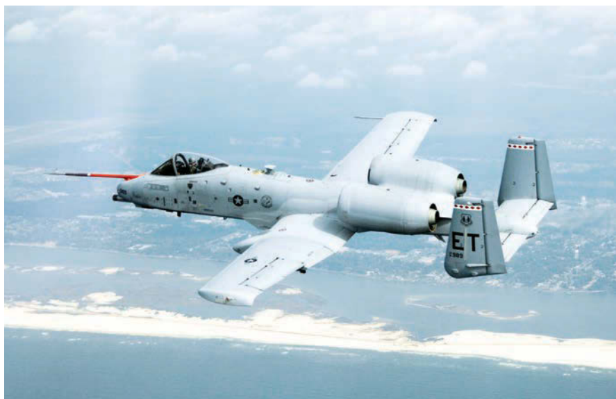
Getting Greener: An A-10C Thunderbolt II from Eglin AFB, Fla., powered by a biomass-derived jet fuel blend of 50 percent Hydrotreated Renewable Jet fuel and 50 percent JP-8, follows the Florida coast on March 25. This was the first flight of an aircraft powered solely with such a blend.
