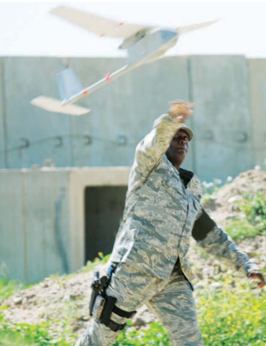
Little Wing: Right, members of the 506th Expeditionary Security Forces Squadron perform an operations check on a Raven unmanned aerial vehicle in Iraq. The UAV carries cameras, sensors, and communications tools and performs a host of ISR duties. Above, MSgt. Bryon Griffin launches the Raven.
