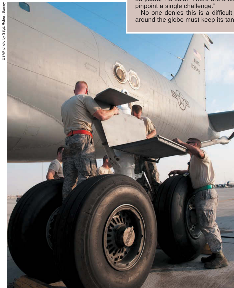
Airmen with the 379th Expeditionary Maintenance Squadron replace a landing strut on a KC-135 tanker in Southwest Asia.
