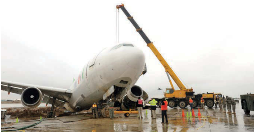
That's One Heavy Lift: USAF crash and recovery teams acted as first responders on March 1 when an Airbus A300 civilian cargo airplane skidded off the runway at Bagram Airfield, Afghanistan. The aircraft's main landing gear collapsed on touchdown. Airmen and soldiers used a 120-ton crane to help clear the runway.
