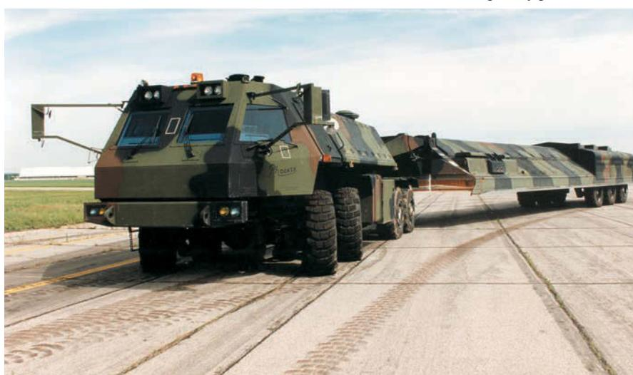
**STRAT-X considered a truck-based transporter system. It presaged the Midgetman system, whose mobile launcher is shown here.**
