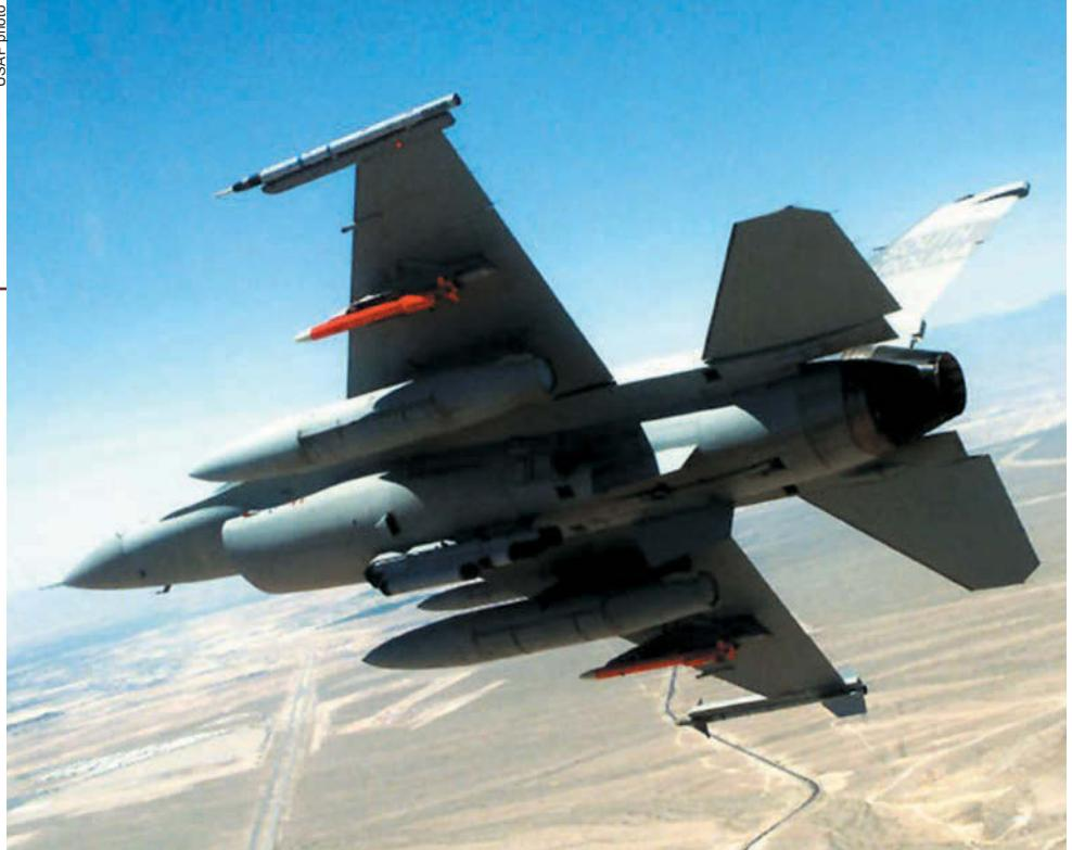
An F-16C Block 52 aircraft equipped with Miniature Air Launched Decoys (in red) joins an exercise over Nellis AFB, Nev.
