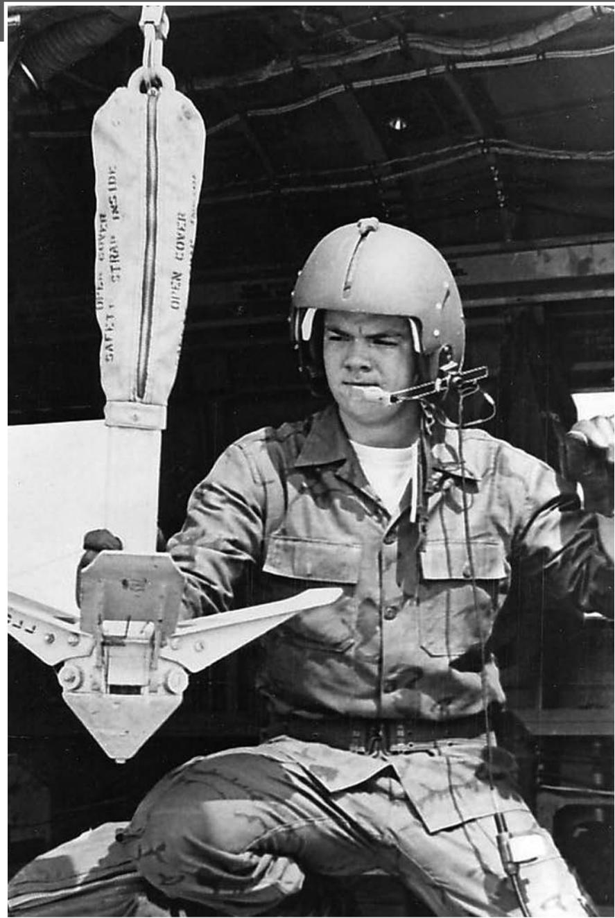
*Air Force pararescue jumper Duane Hackney on duty in Southeast Asia, checking the jungle penetrator on his HH-3 helicopter.*
