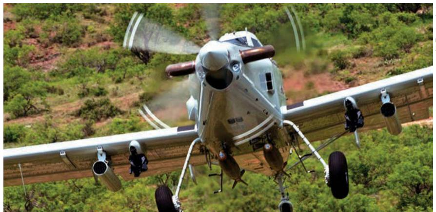
**Air Tractor, of Texas, has entered the light attack aircraft field as well. Shown here is its AT-802U prototype.**
