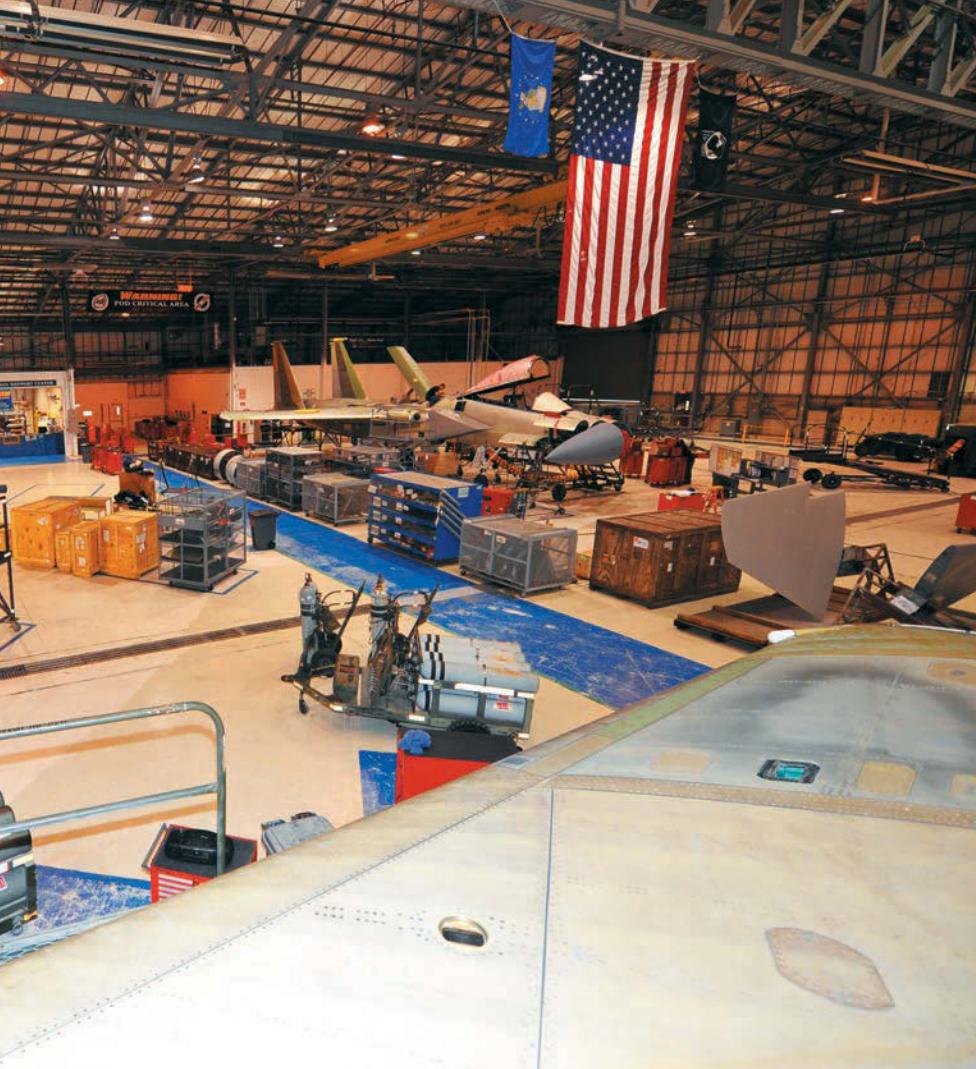
cations take place. Around the building, wings are being disassembled, while stabilizers and tail assemblies are being inspected by technicians looking for signs of trouble.
