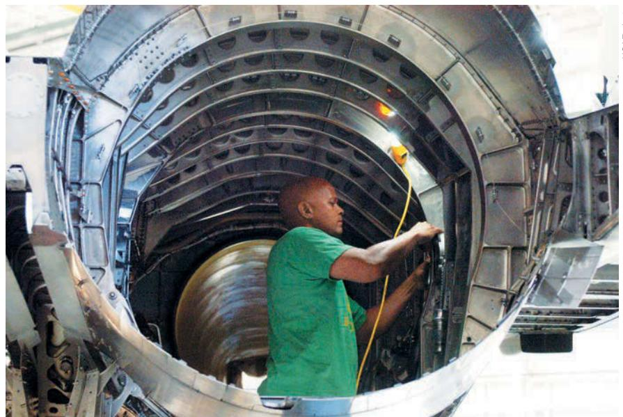
**A sheet metal mechanic with the 561st Aircraft Maintenance Squadron repairs damaged components in an F-15 engine compartment.**
