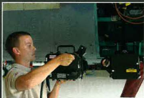
ABE is the perfect solution for sensor and system alignment on F-15 Eagles and F-16 Fighting Falcons.
