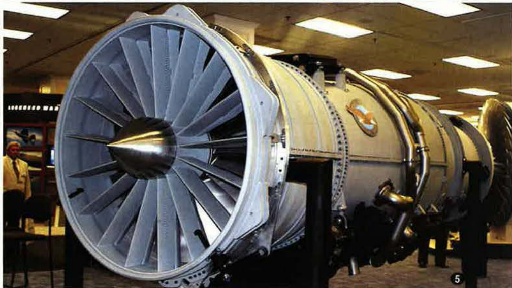
151 A full-scale mock-up of the F135 engine that will power the F-35 fighter dominated the Pratt & Whitney booth. 161 Boeing displayed a cutaway of the
