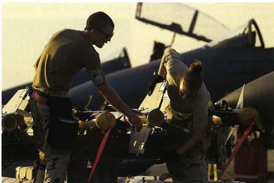
SSgt. Kevin Harvey and A1C Amanda Hicks, weapons loaders with the 494th Aircraft Maintenance Unit, load AMRAAM and Sidewinder missiles onto an F-15E.
