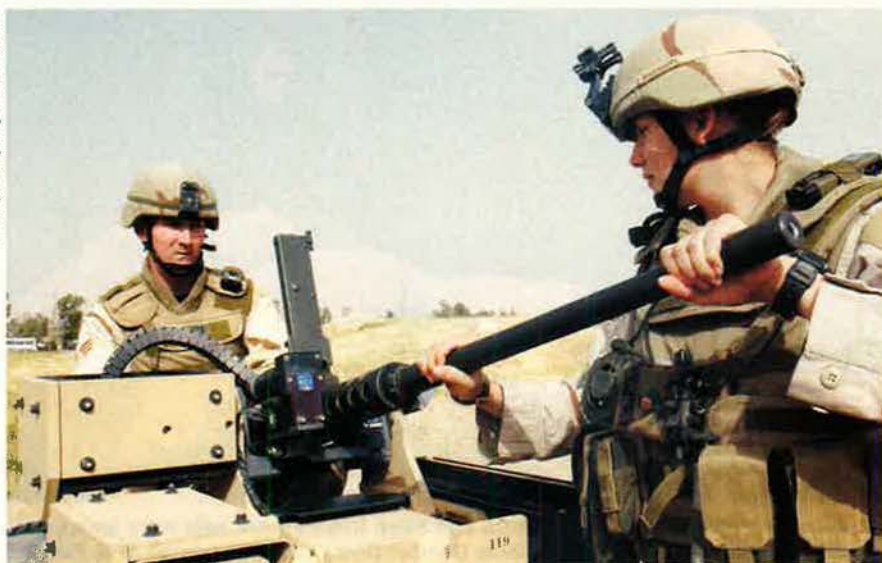
SrA. Jeffrey Oats and SrA. Kesha Snedecker fit a gun to a Humvee at Kirkuk AB, Iraq, in April. The new Common Remote Operated Weapon Station, or CROWS, allows gunners to fire from inside the vehicle, rather than from the vulnerable turret.
