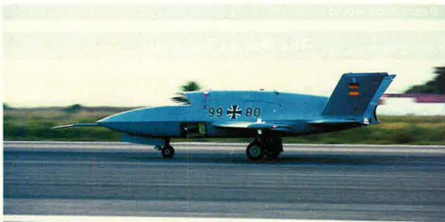
A German "Barracuda" unmanned aircraft test bed takes off on a completely autonomous mission in May. Developed by European Aeronautic Defence and Space Co., the UAV will explore technologies for use in future scout or combat missions.
