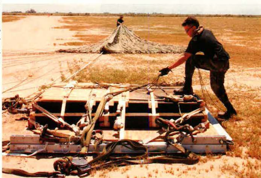
ANG SrA. Mark Richwine disconnects the parachute from a pallet at Edwards AFB, Calif., after a test drop from a C-130J. Active duty, Guard, and Reserve aircrews conducted this airdrop certification test together.
