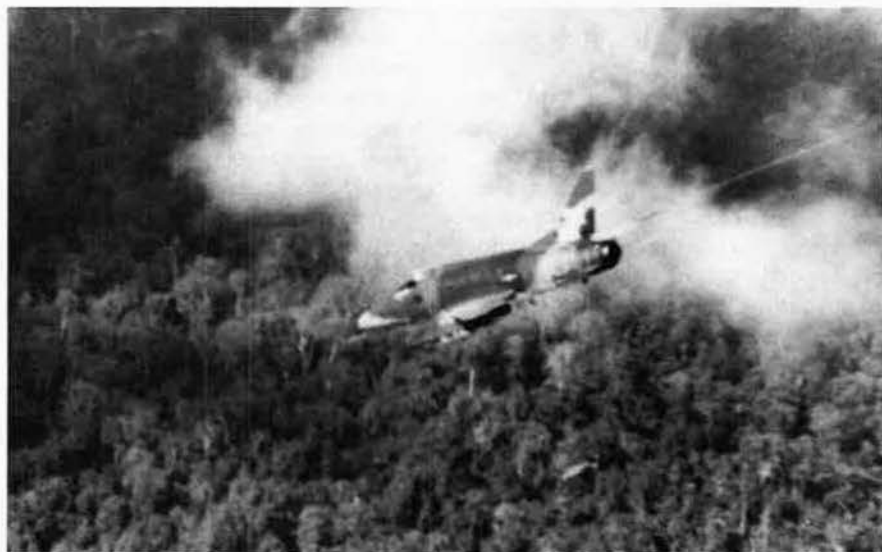
In Vietnam, new radar systems allowed fighters without ground target acquisition radars, such as this F-100, to accurately provide air support. Sky Spot would track the attack aircraft's position relative to a desired release point.
