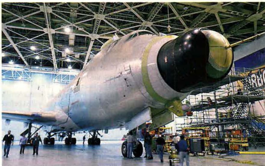
Shown here in preparation for flight testing in Wichita, Kan., the ABL may take its first realistic test shot in 2008. The 747-type aircraft is equipped with a powerful chemical laser weapon for shooting down ballistic missiles in their boost phase.
