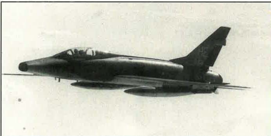
Visible beneath the wings of this F-100F aircraft are rocket pods, each of which carry seven phosphorous rockets. The phosphorous smoke was used by Misty crews to mark targets over enemy territory.
