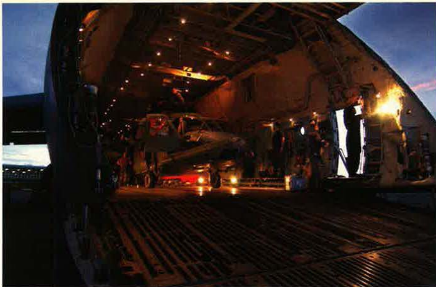
This HH-60G Pave Hawk looks tiny in the cavernous cargo bay of the C-5; up to six of these helicopters will fit inside. The C-5 is unrivaled for its outsize/over-size cargo-carrying capacity.
