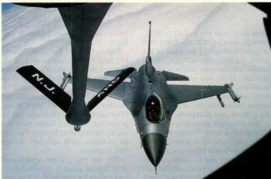
The fighter force patrolling homeland skies works closely with numerous support aircraft. Here, a New Jersey Air National Guard KC-135 tanker refuels a New Jersey Guard F-16.
