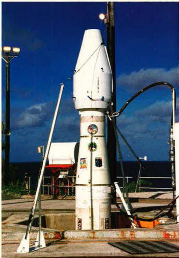
The EKV. The system features 10 silo-based interceptor missiles, each tipped with an Exoatmospheric Kill Vehicle. Some 140 miles in space, the EKV will detach, locate the missile, and smash it.
