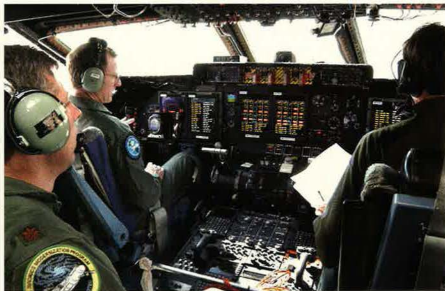
The Avionics Modernization Program brings the C-5 into the 21st century, with glass cockpit avionics, digital systems, and the ability to comply with new international air traffic regulations.
