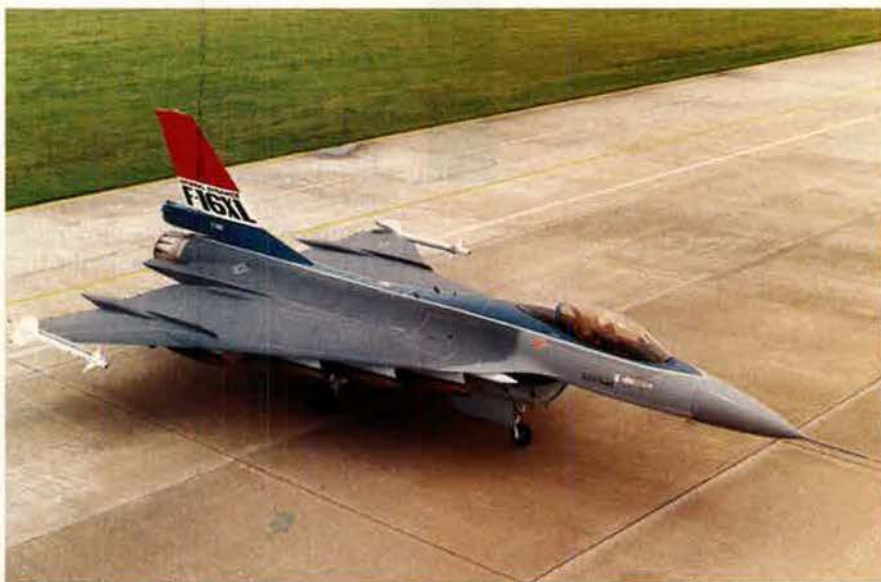
Among the many F-16 variants was the delta-wing F-16XL. Compared to the standard F-16, it could carry more fuel and ordnance, but USAF went with the F-15E Strike Eagle for the deep interdiction role.
