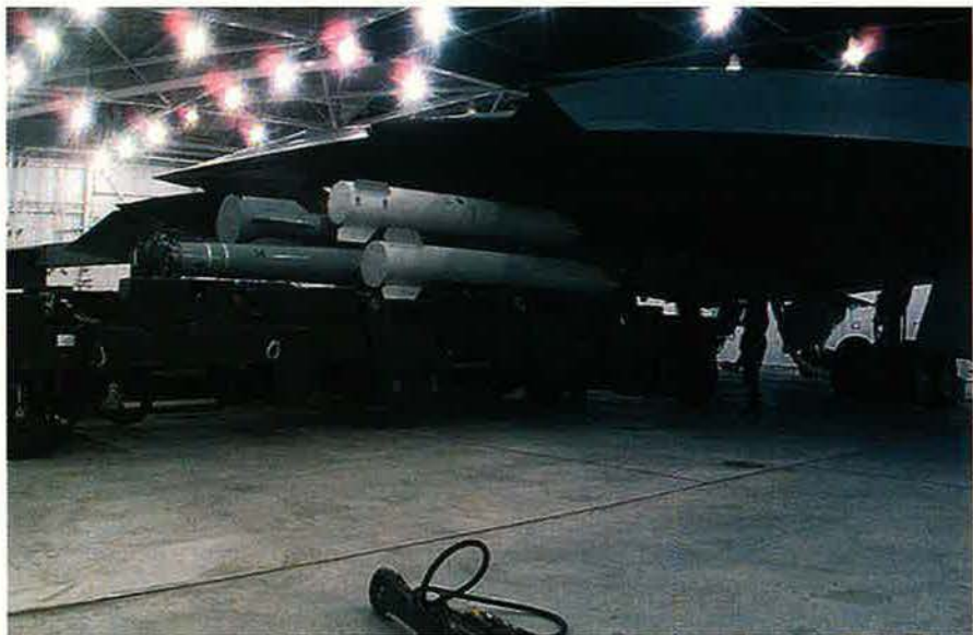
SIOP Bomber. The B-2 retains a nuclear attack mission. In this photo, munitions specialists at Whiteman operate a rotary launcher erector, one of two that would contain nuclear weapons.
