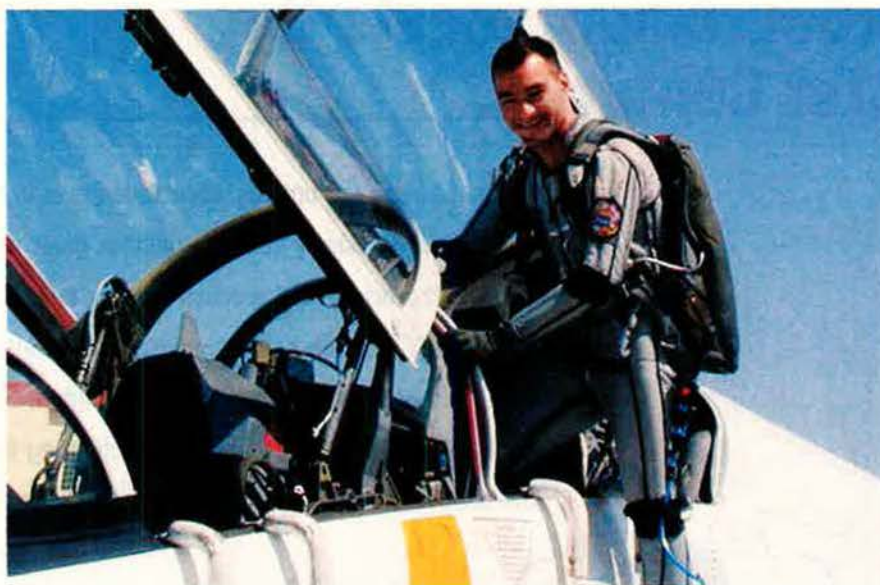
At the USAF Test Pilot School, Edwards AFB, Calif., Capt. Aaron George climbs out of a T-38 after testing a Swiss-made, liquid-filled, full-body anti-gravity suit. The new aircrew protection concept uses hydrostatic force to regulate suit pressure—a possible improvement over current compressed-air anti-g suits.
