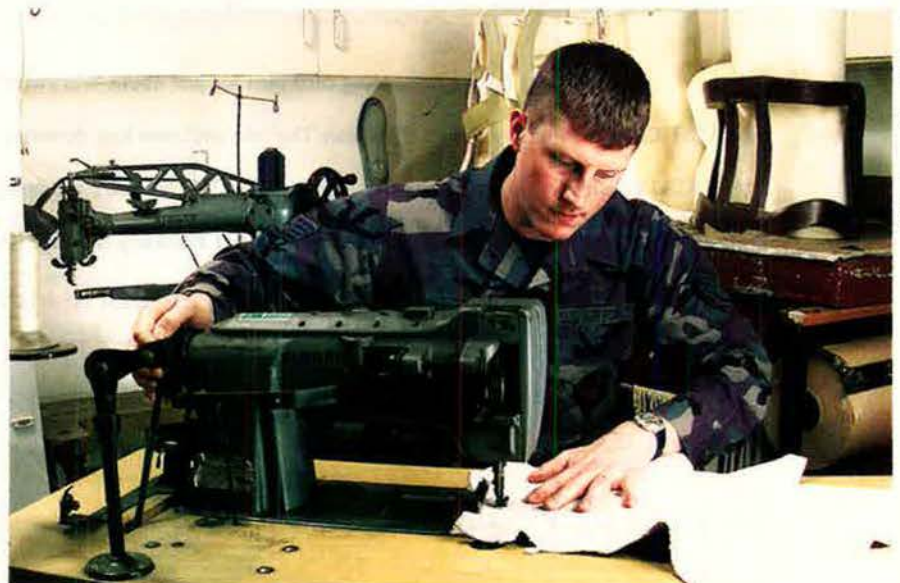
SSgt. Nathaniel L. Raney, an orthotic laboratory technician, 374th Medical Operations Sq., Yokota AB, Japan, uses a sewing machine to fabricate leather cuffs for custom-made leg braces. The lab, which makes wrist splints, cervical collars, ankle supports, and other braces for people with compression-type problems, is the only one of its kind in the Pacific theater.
