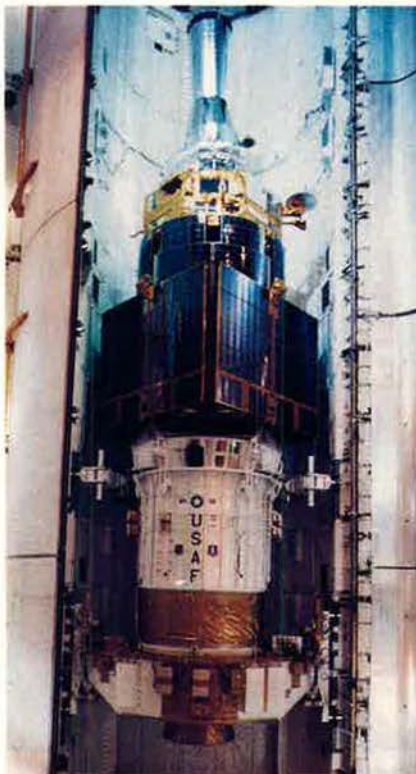
Defense Support Program satellite mounted atop an Inertial Upper Stage booster.
