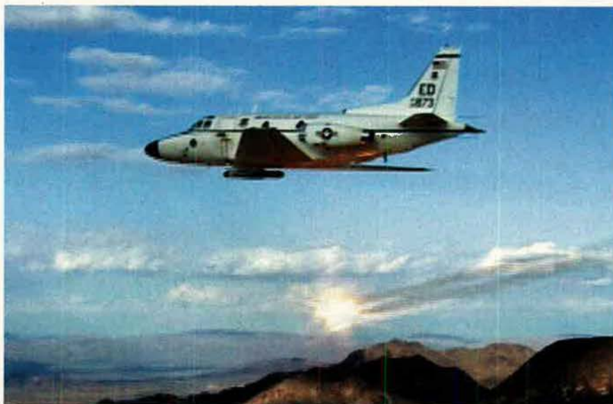
A T-39B ejects a flare during recent testing by the 418th Flight Test Sq., Edwards AFB, Calif. The T-39 can now serve as a low-cost chaff and flare dispenser to support various users, including the Army in testing its ground-based radar systems.
