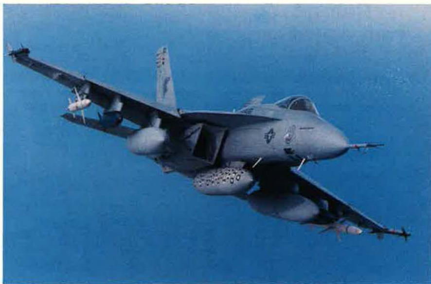
The F/A-18E/F, the "cornerstone of 21st century Navy TACAIR," has front-aspect-only signature reduction. Lack of all-aspect stealth will confine carrier air to the low end of the threat spectrum.
