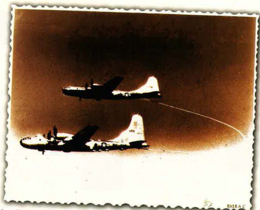
A KB-29 refuels Lucky Lady II during a training mission for the B-50's historic flight. On the actual around-the-world journey, the Superfortress was refueled four times using the drogue system.
