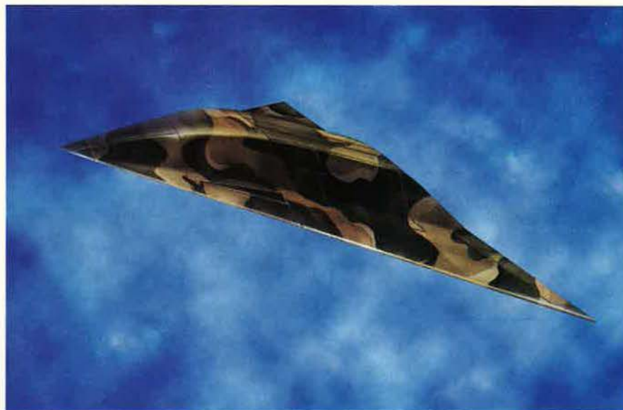
An artist's conception of the Raytheon craft. UCAVs show much potential for SEAD, being smaller, sleeker, and stealthier than a typical fighter and with a loiter time well beyond the duration of a human pilot.
