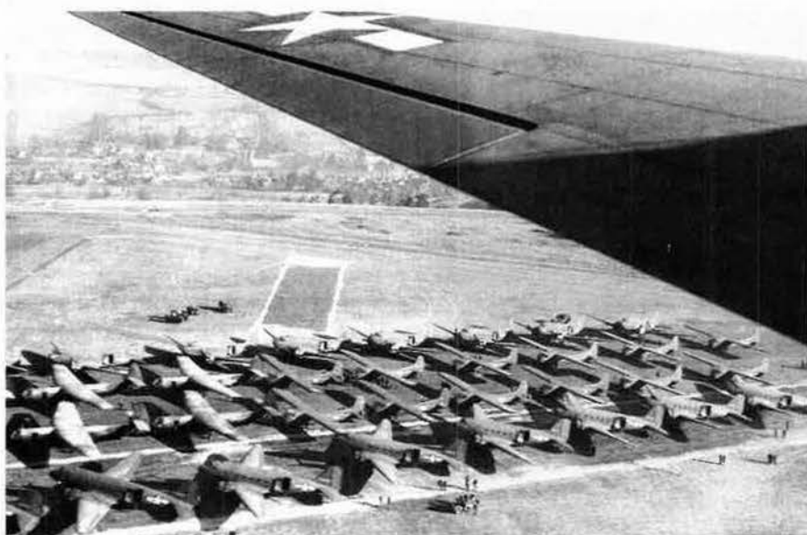
The C-47 Skytrain was the primary troop carrier aircraft. Here, C-47s line an English flightline, with an array of gliders on the inner rows, in preparation for an airborne invasion in Europe.
