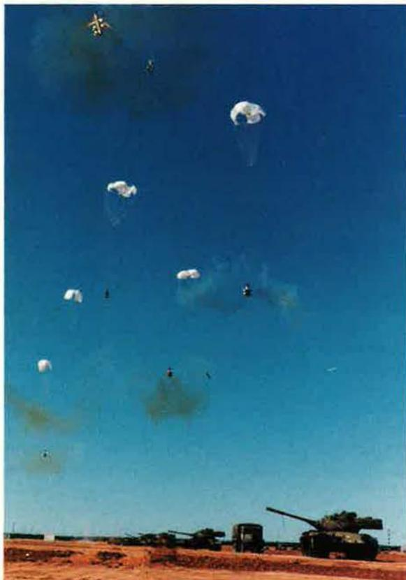
*Once an SFW's tactical munitions dispenser throws out its 10 submunitions, the submunitions hang on a parachute, spinning up their projectiles as they descend. At about 100 feet, the submunitions eject their four projectiles. Each hockey puck-shaped projectile then uses an infrared sensor to locate a hot target.*
