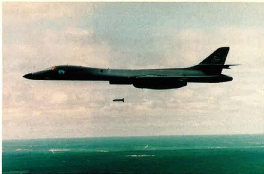
*At left, a Sensor Fuzed Weapon, USAF's newest wide-area cluster munition, 10 times more effective than earlier cluster bombs, takes out a tank during testing. Above, a B-1B bomber releases a CBU-97/B SFW.*
