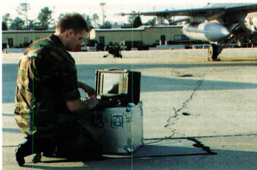
SSgt. Randy Trotter, a 20th Fighter Wing Gold Flag technician at Shaw AFB, S. C., uses the fault test isolation system to detect the source of a problem with an F-16's radar warning receiver. The program's success led USAF to buy the isolation system for every F-16 squadron. (See story below.)
