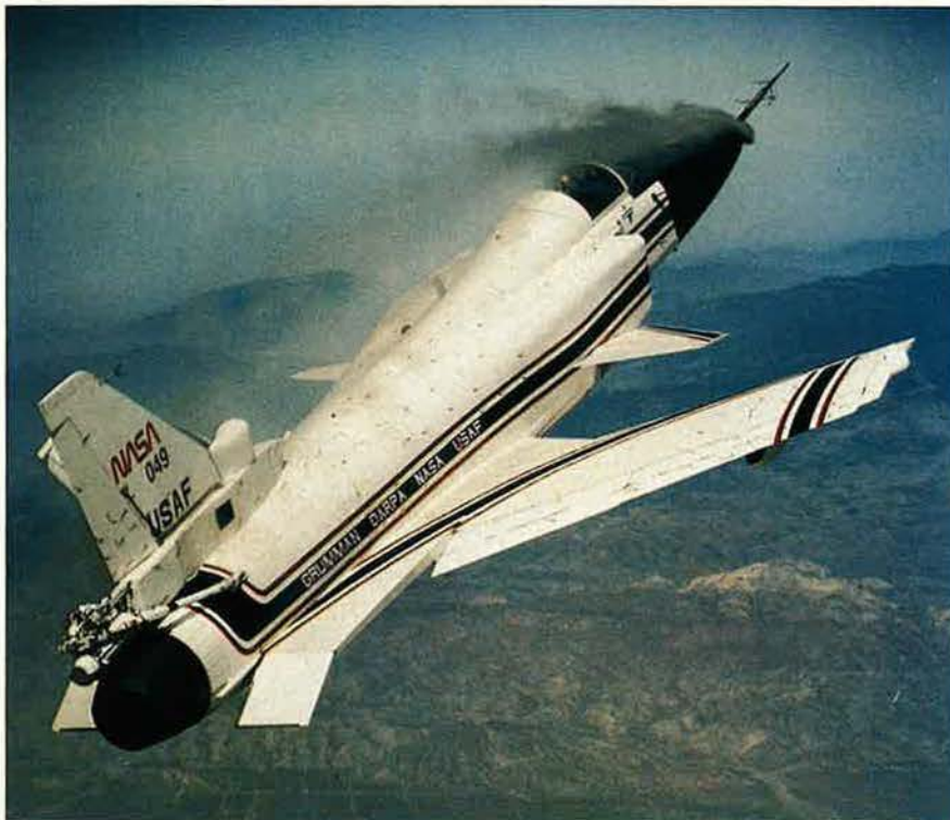
A stream of smoke is released from ports on the nose of the X-29 Advanced Technology Demonstrator to provide information on forebody vortex flows at high angles of attack. The aircraft completed its first phase of high-angle-of-attack military utility flight testing in late September at Edwards AFB, Calif. The X-29 program is a joint effort of USAF and NASA.
