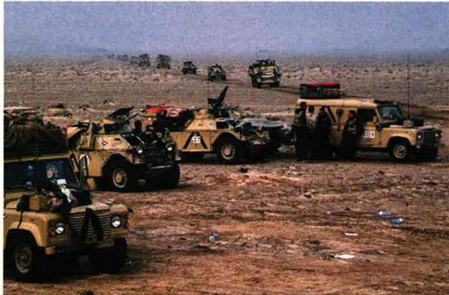
Allied soldiers helped protect themselves from friendly fire by distinguishing their vehicles with inverted "V"s, seen here on the A-1 echelon of the Royal Scots Dragoon Guard advancing into Kuwait. Also visible on some of these vehicles are fluorescent orange air recognition panels.
