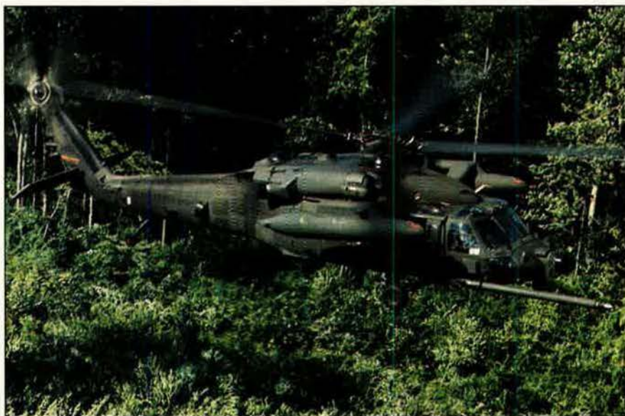
Sikorsky Aircraft delivered its prototype MH-60K special operations helicopter to the Army on August 20. The MH-60K is a modified UH-60 Black Hawk equipped with terrain-avoidance radar and forward-looking infrared systems that allow for low-level flying missions at night and in adverse weather.
