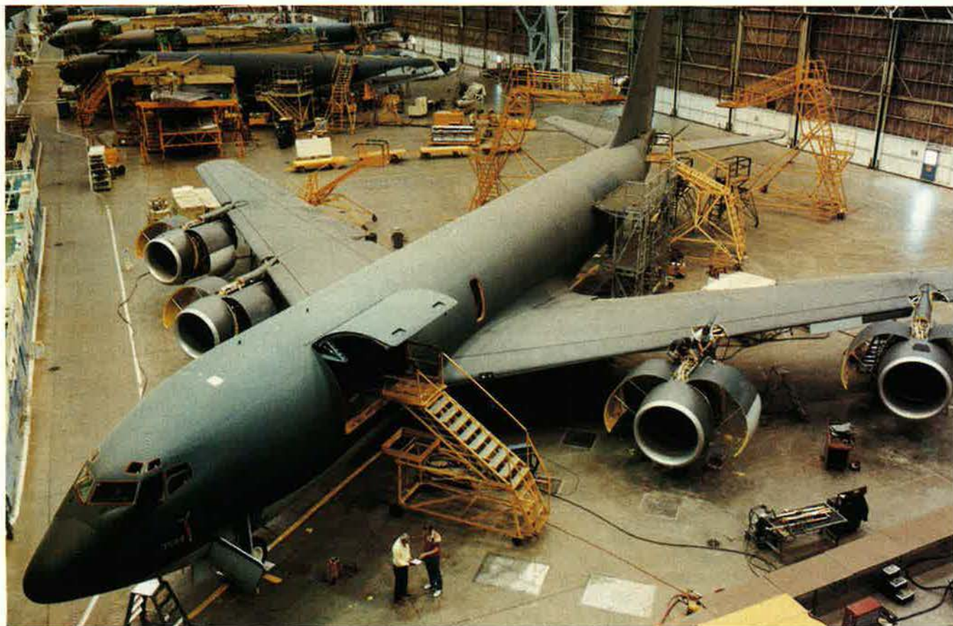
At a Boeing plant in Wichita, Kan., a KC-135 receives a new engine. The KC-135R modification made the tanker quieter, less smoky, and more efficient; some 250 aircraft have been converted since the early 1980s. Despite such successes, thousands of contractors, subcontractors, and suppliers have left the defense business, partly as a result of federal defense budget cuts.
