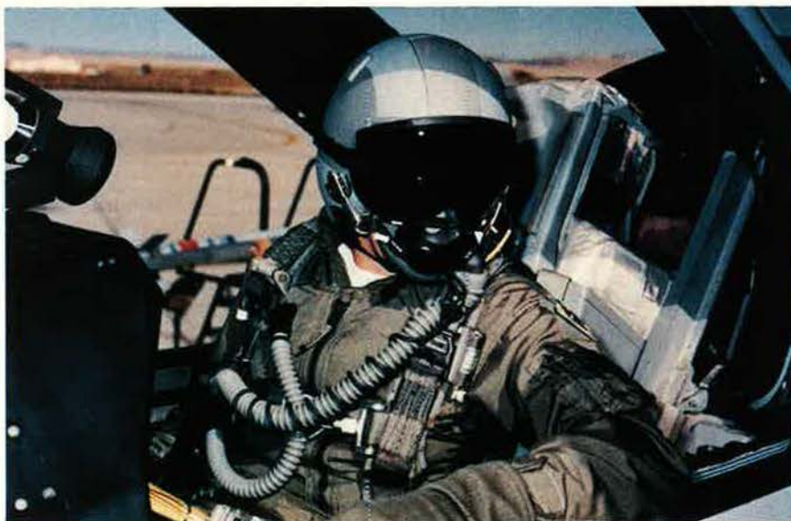
A pilot's first line of defense against GLOC is the anti-G suit. As the G level rises, a valve inflates bladders over the abdomen, thighs, and calves to exert counter-pressure against pooling of blood in the lower body. Another bladder keeps the oxygen mask sealed to the pilot's face. The suit provides up to two Gs of protection.
