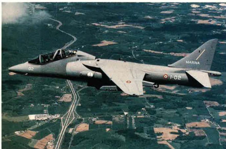
A TAV-8B Harrier II with Italian Navy markings flies over Missouri during a test by McDonnell Aircraft. It is one of two going to the carrier Giuseppe Garibaldi to train Italian Navy pilots for the Harrier II Plus, whose radar integration and production is a collaborative program by the US, Spain, and Italy.
