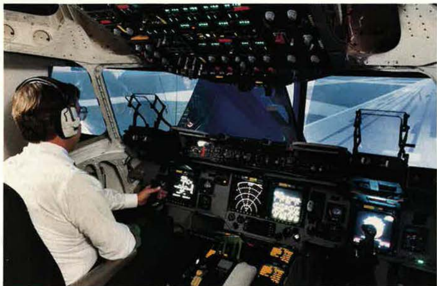
Avionics Integration General Manager Ed Bailey of Douglas Aircraft Co. works the controls of the C-17 airlifter's flight-hardware simulator, which is used to verify the integration of all C-17 flight control and avionics hardware and software. The cockpit features stick instead of yoke controls and a head-up display similar to those in fighter aircraft. The C-17 is scheduled for its first flight this summer.
