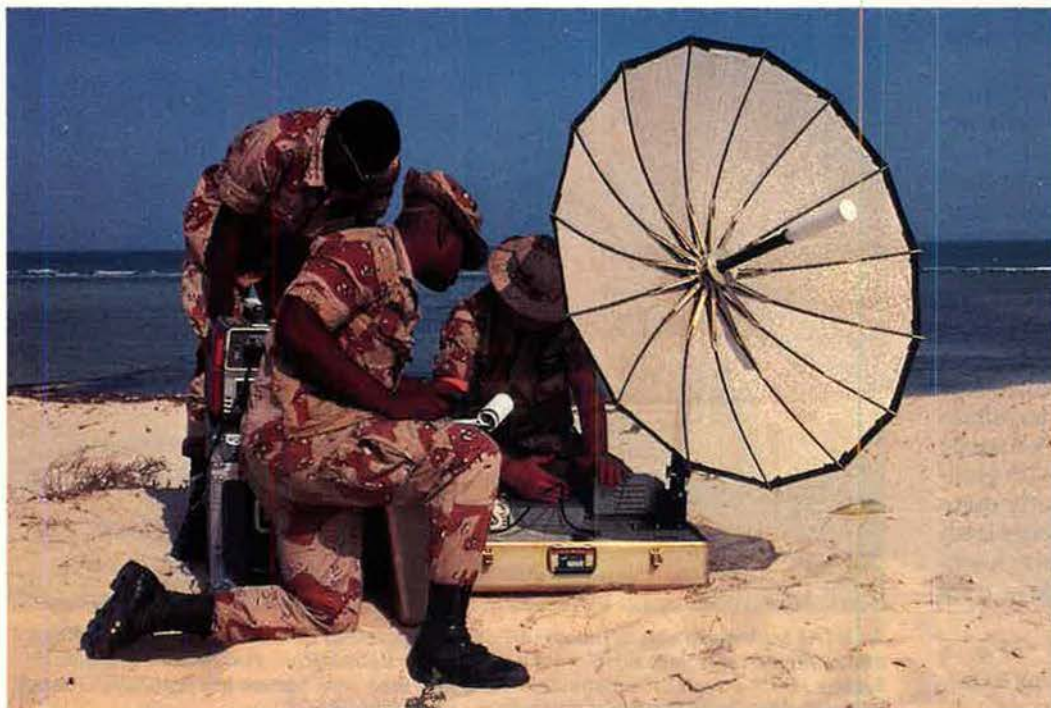
Crew of a joint combat camera section set up a station for transmitting still video images from a forward-deployed position to the Pentagon. All sorts of ground stations were Gulf War staples, and US forces learned a lot about the nature, uses, and availability of space resources.
