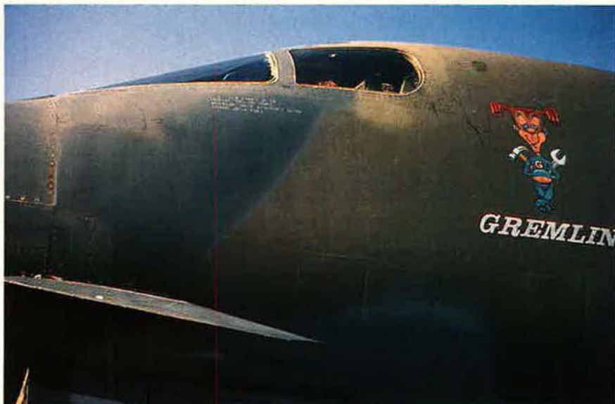
The military aircraft designation block is normally stenciled on the left side of the fuselage just below the canopy window, as on this B-1B bomber. Designations are based on missions, designs, and vehicle types.
