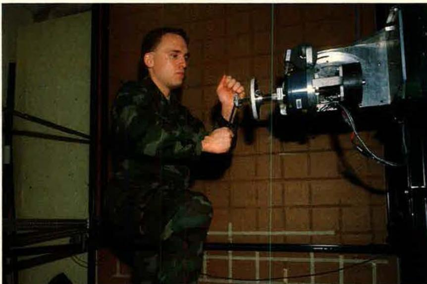
As test subject SSgt. Arch Currid tightens a bolt while kneeling, all of the forces and moments he employs to move the wrench are measured to become a part of the database for CREW CHIEF, a computer modeling system for maintainers. With these parameters, a designer can change a design still on the drawing boards.
