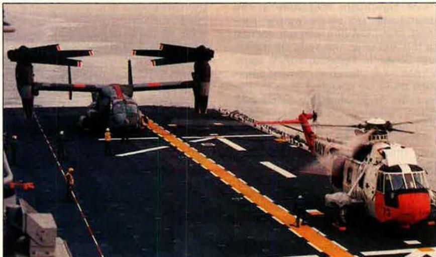
*The number four V-22 Osprey flight test aircraft prepares for takeoff from the deck of USS Wasp (LHD-1). The V-22's wing has been rotated into position, and the rotor blades are about to be unfolded. Completion of initial shipboard compatibility trials last December was an important milestone in the aircraft's development.*
