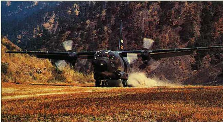
The C-27A intratheater airlifter for Southern Command will be a modified version of the Aeritalia G.222 STOL transport (here, coming in for a landing on a dirt strip). The C-27s will fill the airlift gap between CH-47s and C-130s in Central America.
