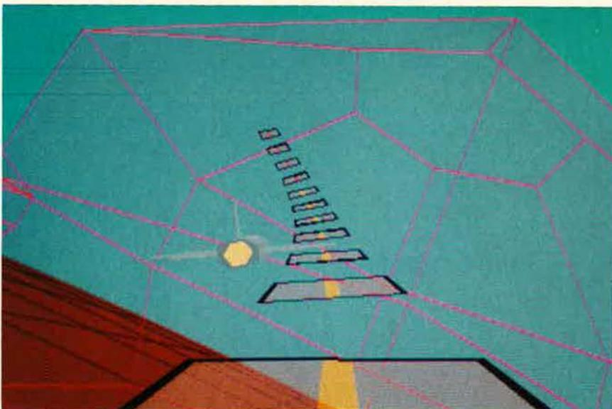
*In this prototype virtual cockpit display, the "follow-me" airplane gives the pilot a visual "rabbit" to follow. The pavement sections show the pilot the best pathway to fly. The amber lines indicate danger, and the red framework shows the pilot he is in a threat area. The rust-colored area represents the ground.*
