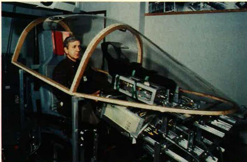
*The rapidly configurable cockpit simulator is a key element of the CAT (cockpit automation technology) program. If a new display or control works here, it may eventually move to flight test. The simulator, here "flown" by Joe Hendrix, a contractor employee, will be delivered to Wright-Patterson this year.*
