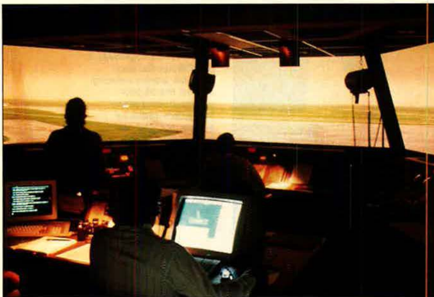
Logicon delivered the Federal Aviation Administration's new computerized, voice-controlled air traffic control tower simulator on January 25. The $10 million simulator will be used to train air traffic control students at the FAA Academy in Oklahoma City, Okla. Students will talk to aircraft images through microphones, and the images will respond through a voice recognition system.
