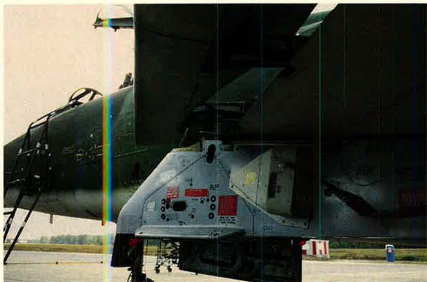
The wing pylons on the QF-100 above have been modified with a chaff-and-flare dispenser to imitate enemy aircraft more realistically for test missiles. Drone pilots find the cockpit (below) Spartan at best. Anything unrelated to flight safety and unneeded for testing is removed. Notice the lead weights where a gunsight once was.
