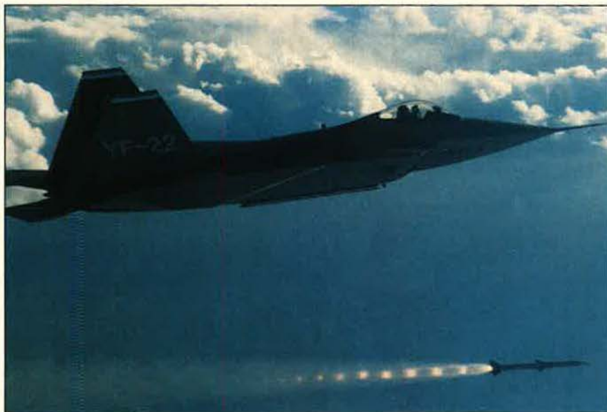
An AIM-120A Advanced Medium-Range Air-to-Air Missile was launched from the number two Lockheed/Boeing/General Dynamics YF-22 prototype (powered by P&W engines) on December 20. The missile, not aimed at a target, ignited well clear of the plane's internal weapons bays. All four prototype aircraft are now in flyable storage at Edwards AFB, Calif., awaiting the Air Force's decision.
