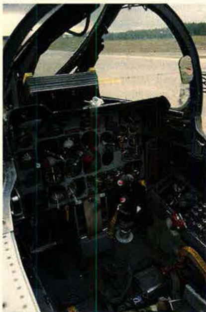
The wing pylons on the QF-100 above have been modified with a chaff-and-flare dispenser to imitate enemy aircraft more realistically for test missiles. Drone pilots find the cockpit (below) Spartan at best. Anything unrelated to flight safety and unneeded for testing is removed. Notice the lead weights where a gunsight once was.
