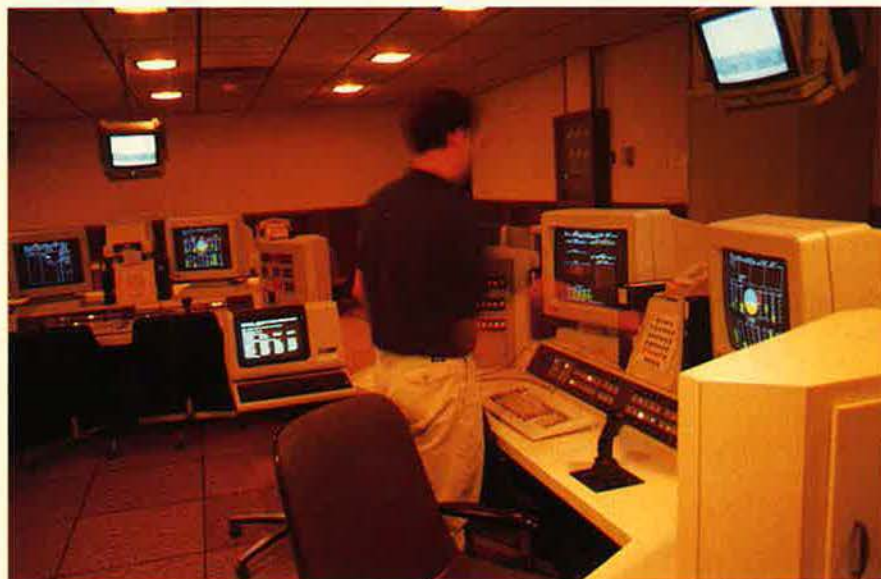
The Gulf Range Drone Control Upgrade System (GRDCUS), a state-of-the-art computer system, can control up to four full-scale drones at one time. Above, Marty Walker, a contract software analyst, works a GRDCUS station. The control stick on the desktop is used to fly the drone.
