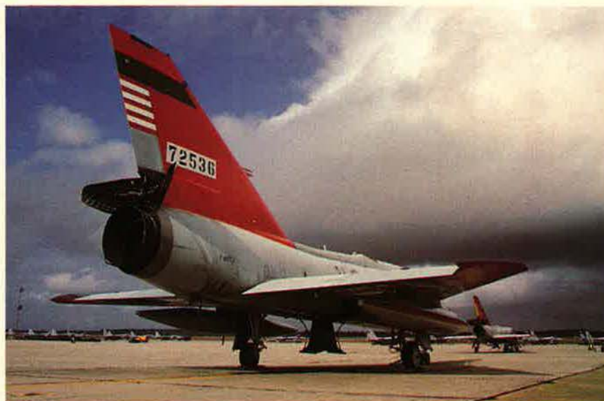
The Convair F-106 Delta Dart interceptor, phased out of ANG service three years ago, is starting its second life as a full-scale target drone. All full-scale drones' wingtips and vertical stabilizers are painted orange, but QF-106s' rudders retain the fin flash insignia of their last unit, mainly for rudder balance.
