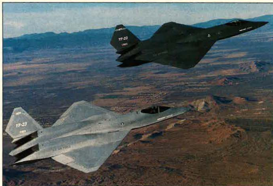
The demonstration/validation phase of the Air Force's Advanced Tactical Fighter program was concluded on December 31. The Northrop/McDonnell Douglas design, the YF-23, was the first to fly and the first to finish. The first YF-23 (top) is powered by two Pratt & Whitney YF119-PW-100 engines; the number two aircraft (bottom) is powered by a pair of General Electric YF120-GE-100 engines.
