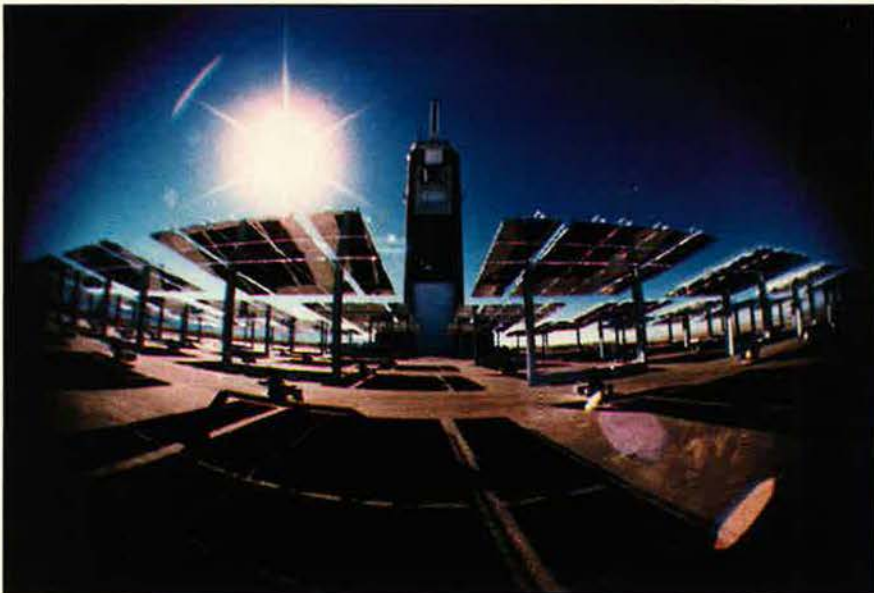
A new wind tunnel, sponsored by the Air Force, has been installed at the Sandia National Laboratory at Kirtland AFB, N. M. Using the 220 sun-tracking heliostats of the National Solar Thermal Test Facility (shown here) and airflows of up to 240 miles per hour, the tunnel (in the tower, center) can simulate the irradiating effects of nuclear thermal flash on aircraft materials.
