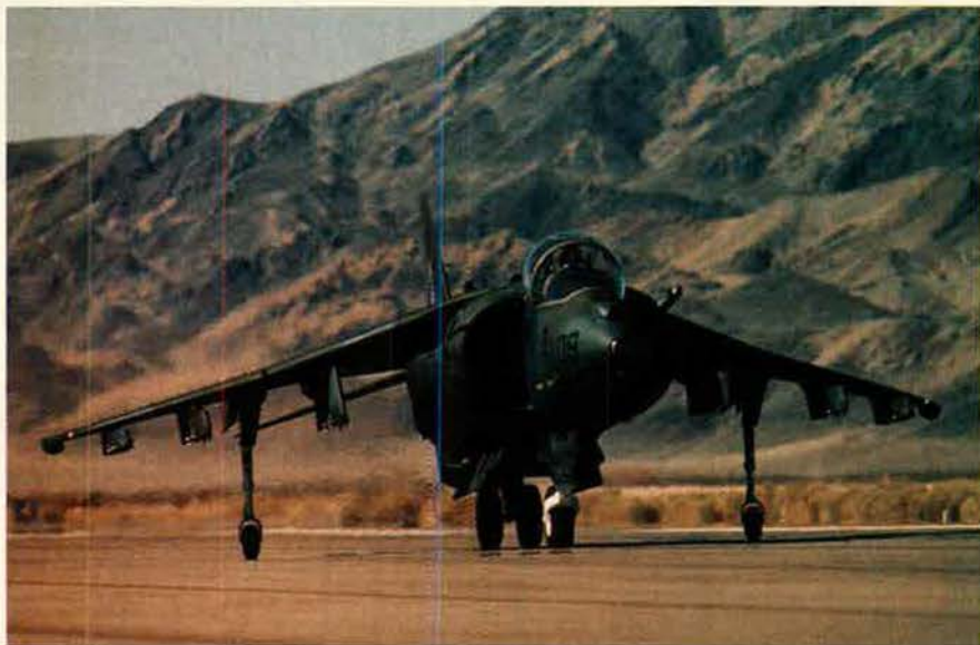
The first vertical takeoff aircraft to enter squadron service was the Harrier. Its remarkable capabilities come from a Rolls-Royce Pegasus engine using vectored thrust directed through four nozzles mounted on the fuselage. Above, a Marine AV-8B Harrier II returns to Indian Springs, Nev., during an exercise.
