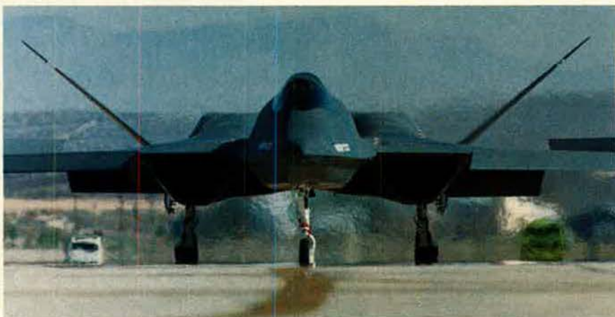
The heat haze behind this Northrop/McDonnell Douglas YF-23 prototype demonstrates the difficulty of hiding the hot efflux of even a stealth fighter from enemy infrared search and track systems.
