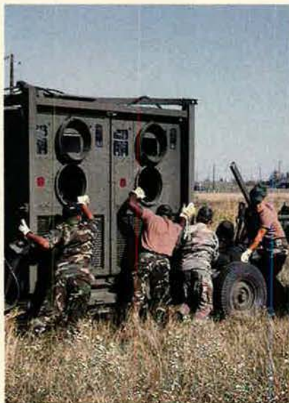
Four persons can set up a shelter unit in fifteen minutes. It used to take forty workers and twenty-four hours. TACS operators can assemble an entire TACC and its equipment in six hours.
