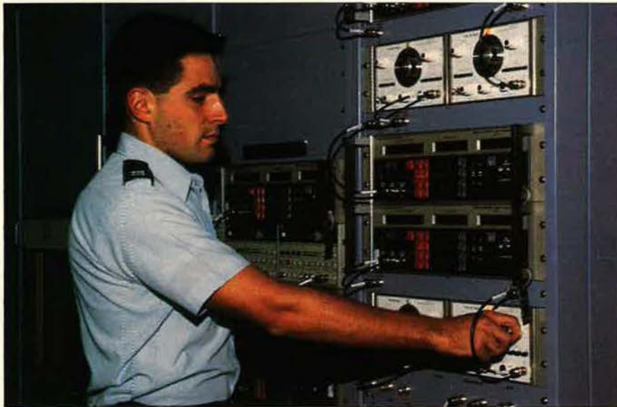
The avionics laboratory's "avionics wind tunnel"—the Electromagnetic System Simulator—can create an entire flight environment, complete with electronic warfare, communications, and sensor inputs. This allows the laboratory engineers to test equipment in a "real" situation before actual flight tests are performed.
