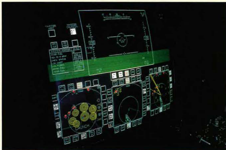
Research into flat panel displays for the cockpit has been under way for nearly eighteen years. This laboratory test article shows a "glass cockpit" display. While active-matrix, color liquid crystal multifunction displays are being introduced and promise great benefits, they can't be produced in large sizes, they sometimes need a warm-up period, and they will require a large investment in production facilities.
