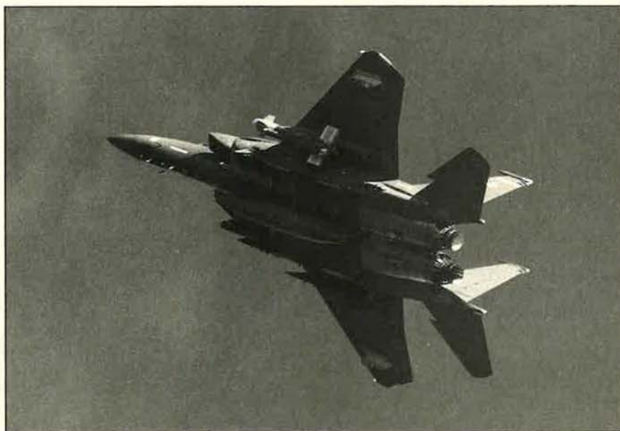
The Rockwell AGM-130A, the rocket-propelled version of the GBU-15 glide bomb (shown here on an F-15E), was recently cleared for production. Failures in early tests nearly led to termination of the standoff weapon program. The Air Force is seeking funding for 960 TV-guided and 3,088 infrared-guided AGM-130s. Air Force Systems Command's Munitions System Division (now the Air Force Development Test Center) at Eglin AFB, Fla., oversaw AGM-130 development.
