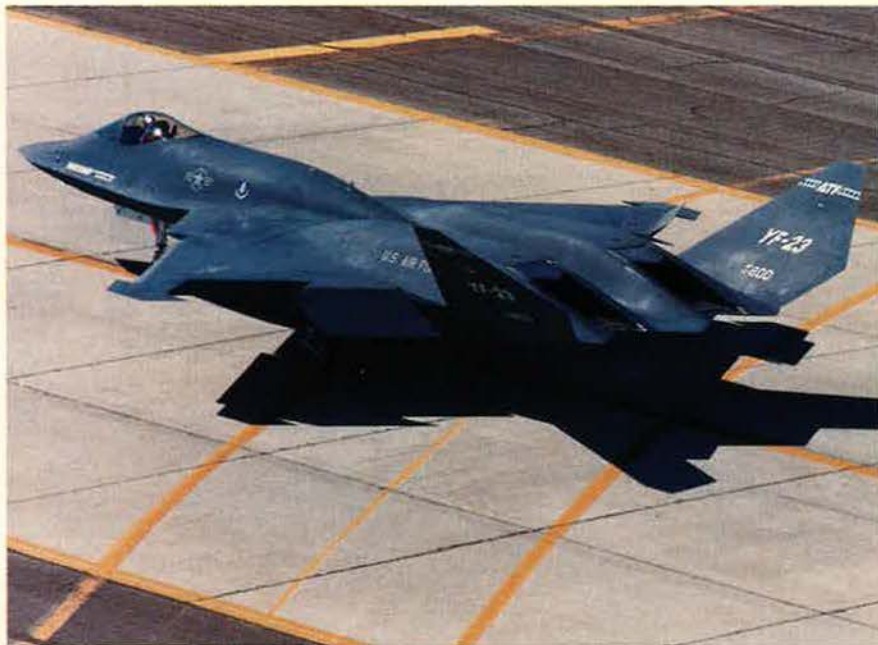
This photo shows the YF-23's fixed, rectangular exhausts, similar to those on the B-2. The exhausts appear to be surrounded by heat-absorbing material similar to that on the space shuttle and are also masked by the ruddervators. Video footage reveals that all of the YF-23's control surfaces (except the leading edge slats) can be operated independently. This will greatly increase maneuverability.
