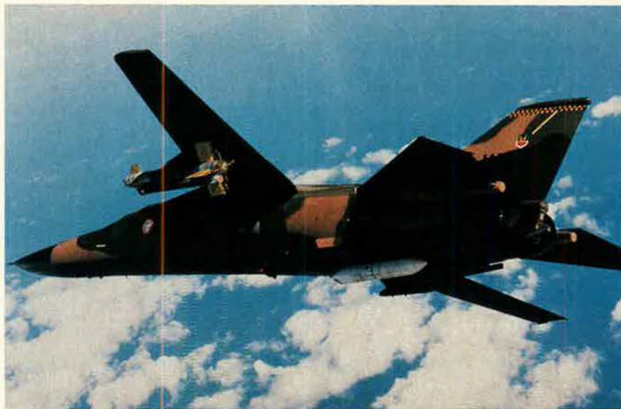
An AGM-130 goes aloft on an F-111 for a flight test. AGM-130s can be launched by F-111s, F-15Es, and F-4s, and they can be adapted to F-16s. Each missile can carry a 2,000-pound warhead more than twenty miles, something that no other nonnuclear missile in the US arsenal can do.
