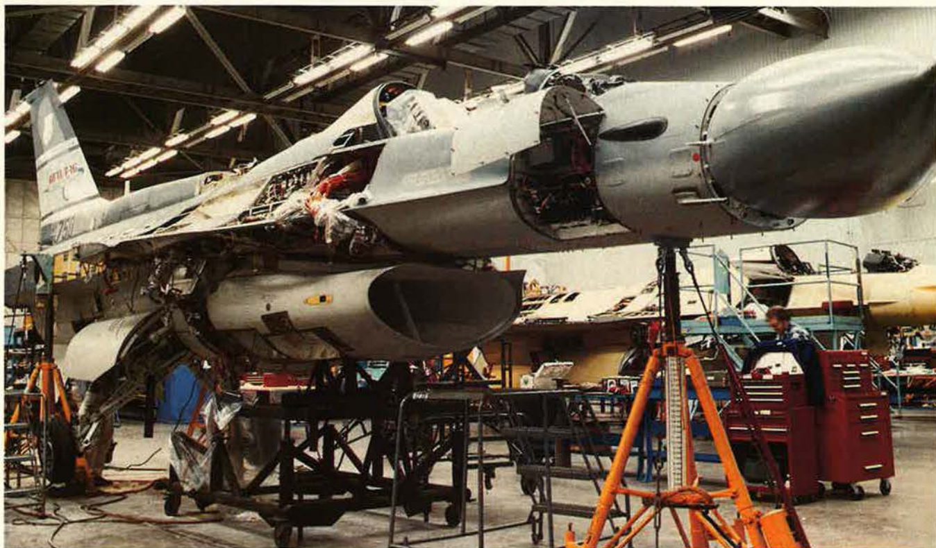
When the AFTI/F-16 emerges from its refit later this year, the aircraft will have the APG-68 radar that is fitted in current production F-16s, and the avionics will be brought up to the Block 40 production standards. The AFTI/F-16 will also get a head-steerable, forward-looking infrared sensor, but its trademark canards will not be replaced.
