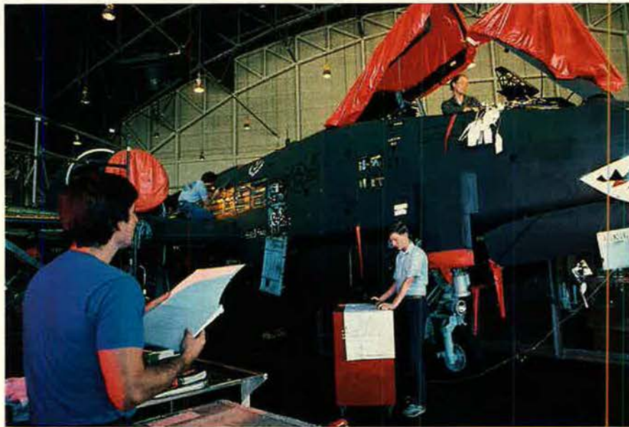
A-10s are among the aircraft given new strength and longer life through the use of composite materials developed at Sacramento ALC. As part of programmed A-10 maintenance, as shown here, the wings' leading edges are removed and replaced with ones made of advanced composites to prevent damage from birdstrikes.
