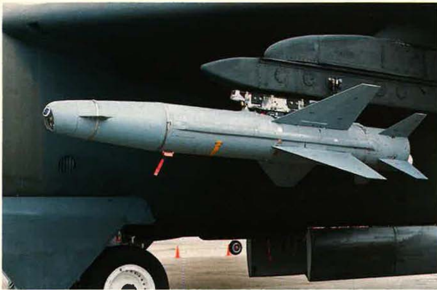
Strategic Air Command has turned to the Israel-made AGM-142A Have Nap missile, shown here, to give B-52 bombers potent, nonnuclear, standoff capability. USAF now believes that standoff weapons are here to stay.
