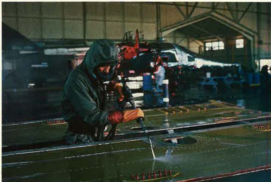
Workers in the aircraft wash rack wear protective gear and air supply equipment while using high-pressure water guns to desal F-111 fuel tanks. Fuel leaks are a common problem in F-111s. A special Process Action Team modified maintenance processes to significantly reduce maintenance delays caused by fuel leaks.
