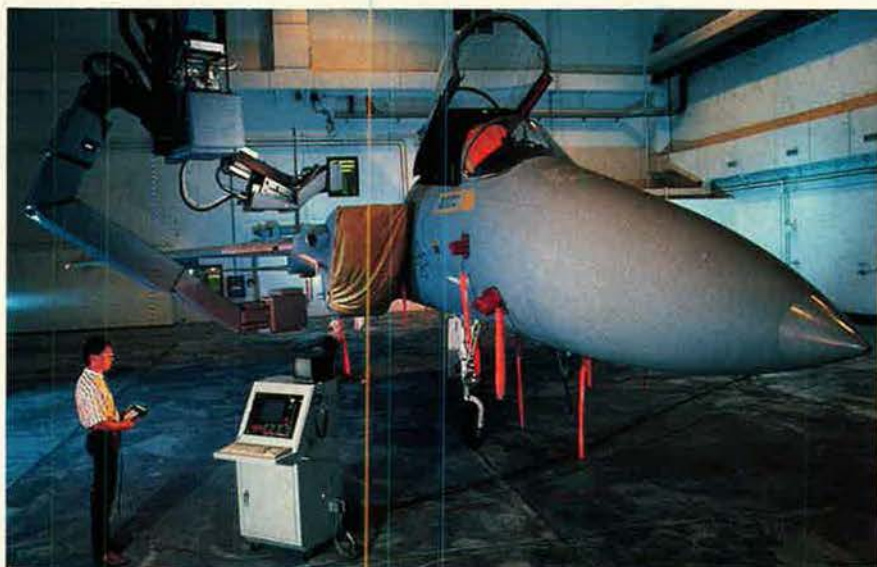
Nondestructive inspection technician Gerald Abah programs the world's largest robot to inspect an entire F-15 for cracks and corrosion. McClellan's new facility, the only one of its kind, allows the internal inspection of intact aircraft using X-ray and neutron radiography.
