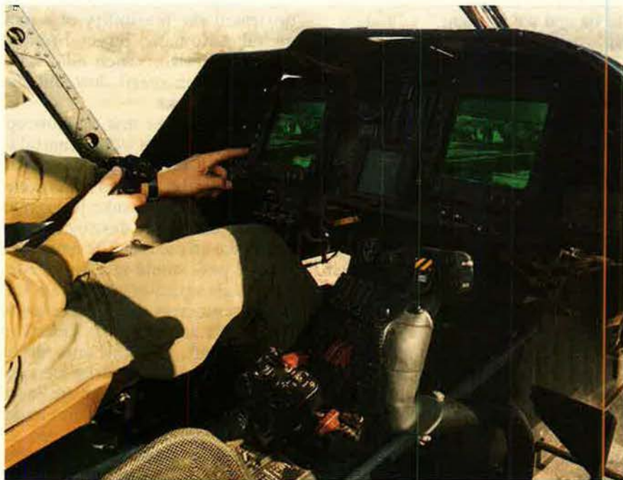
In the successful first phase of the technology demonstration effort (CAS I), an Army pilot used the McDonnell Douglas-built, mast-mounted sight on the OH-58D's rotor hub to generate images (as seen on the two multifunction displays on the panel at left) that conveyed targeting information to the AFTI/F-16's pilot (above).
