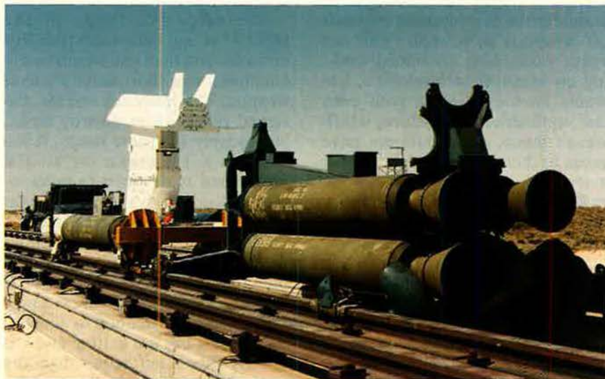
An advanced aircraft munitions dispenser, painted white, is moved into position for a sled test, prior to flight testing at Holloman AFB, N. M. Such dispensers are being developed in standard configurations for a variety of munitions and aircraft as USAF heads full-steam into the standoff-weapons era.
