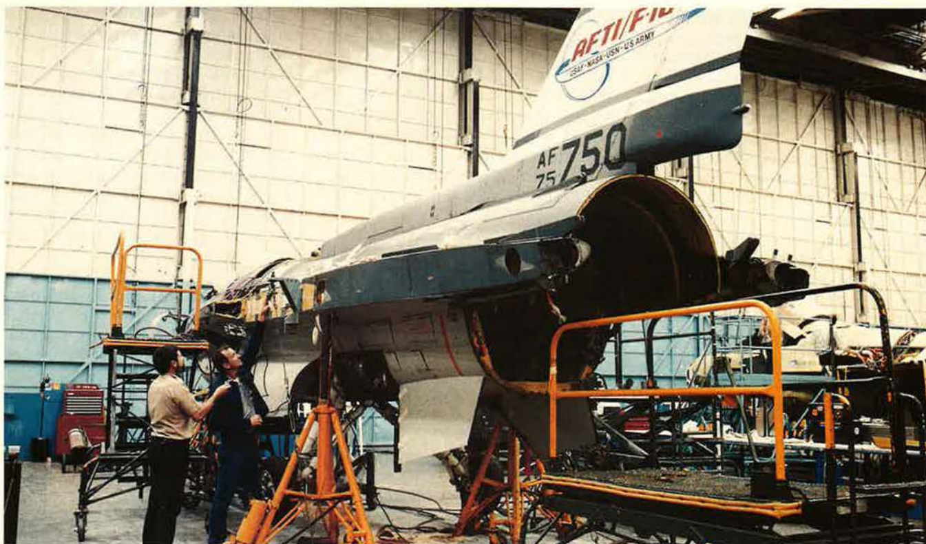
The Advanced Fighter Technology Integration F-16 is now back at the General Dynamics plant in Fort Worth, Tex., being readied for the second half of the second phase (CAS II) of the technology demonstration effort. Once testing resumes, the AFTI/F-16 will demonstrate weapons delivery from low altitude while avoiding collisions, guided by the plane's digital map.
