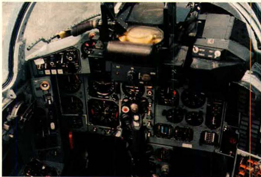
The roomy cockpit of the MiG-29 resembles USAF F-105/F-4-vintage design. The author's cockpit (above) had a few vertical tape instruments and many round analog dials. G-suit, oxygen, and communications leads were on the left. The throttles moved along horizontal bars mounted against the left side wall. The inboard throttle carried a speedbrake switch and an ICS button. There was no radar display, but there was a keypad with digital readouts that may have been part of the INS system.
