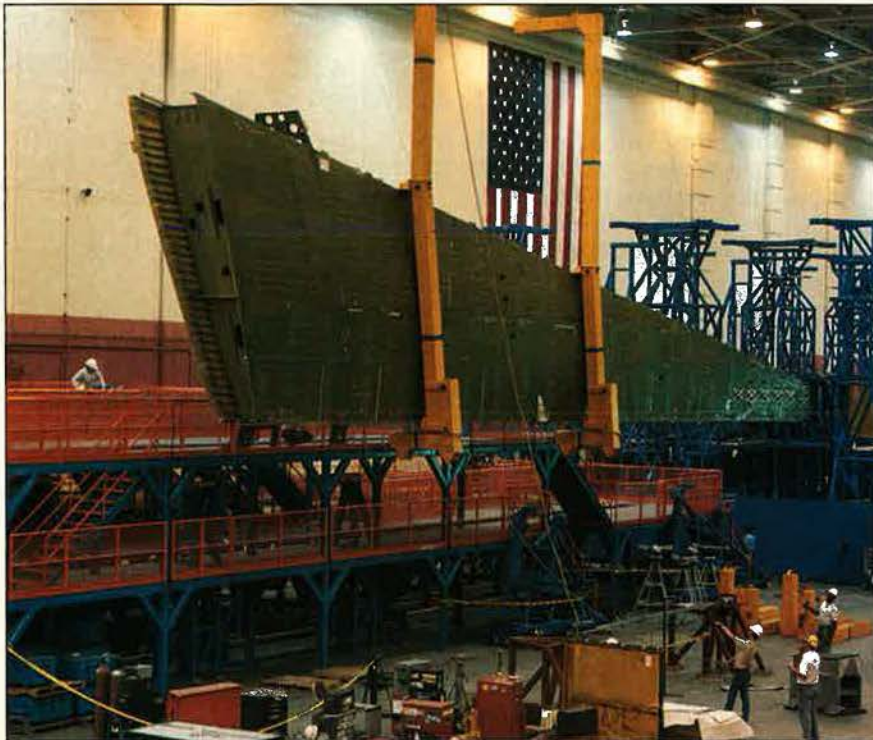
Late last year, several major C-17 components were moved from their assembly jigs at the Douglas Aircraft Co. plant in Long Beach, Calif., in preparation for joining operations. The first section of wing, ninety-two feet long and weighing 28,000 pounds, was placed in an interim jig before being moved to a horizontal fixture where it was joined with the other half of the wing in January.
