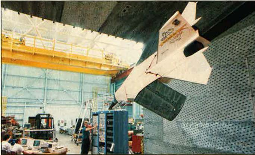
Engineers at Air Force Systems Command's Arnold Engineering Development Center prepare a one-twelfth-scale model of the Advanced Fighter Technology Integration F-111 for wind-tunnel testing. The test provided aerodynamic data on characteristics of configurations of the plane's Mission-Adaptive Wing in different positions.
