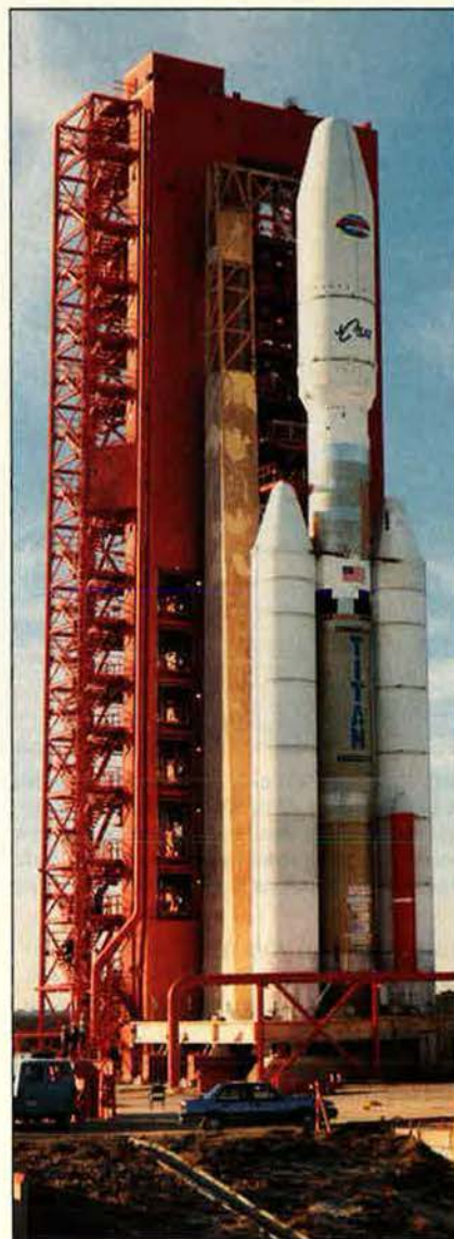
The first commercial Martin Marietta Titan space booster was successfully launched from Cape Canaveral AFS, Fla., on December 31. The commercial Titan III, a derivative of the Titan 34D, is capable of lifting 32,500-lb. payloads to low-Earth orbit.
