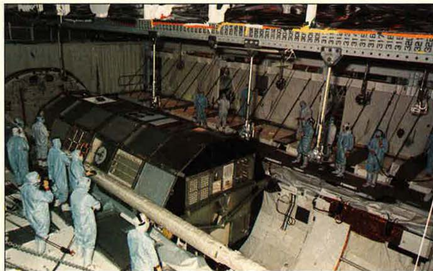
On January 30, technicians at the Orbiter Processing Facility at the Kennedy Space Center got a first look at the Long Duration Exposure Facility (LDEF) after it was retrieved during space shuttle mission STS-32. The long, foil-wrapped object in the foreground is the remote manipulator arm used to grab LDEF.
