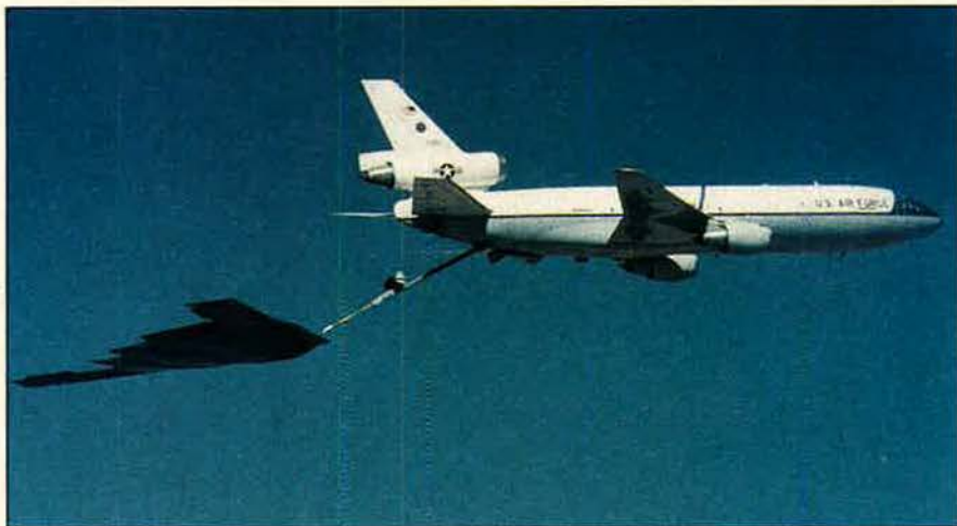
The Northrop B-2A Stealth bomber completed its first series of flight tests on September 23. The five flights were designed to expand the flight envelope, check the function of the aircraft's subsystems, and, as shown here, demonstrate the aircraft's handling qualities while flying in a position to be air refueled. Northrop test pilot Bruce Hinds and Lt. Col. John Small are flying the B-2 underneath a KC-10.
