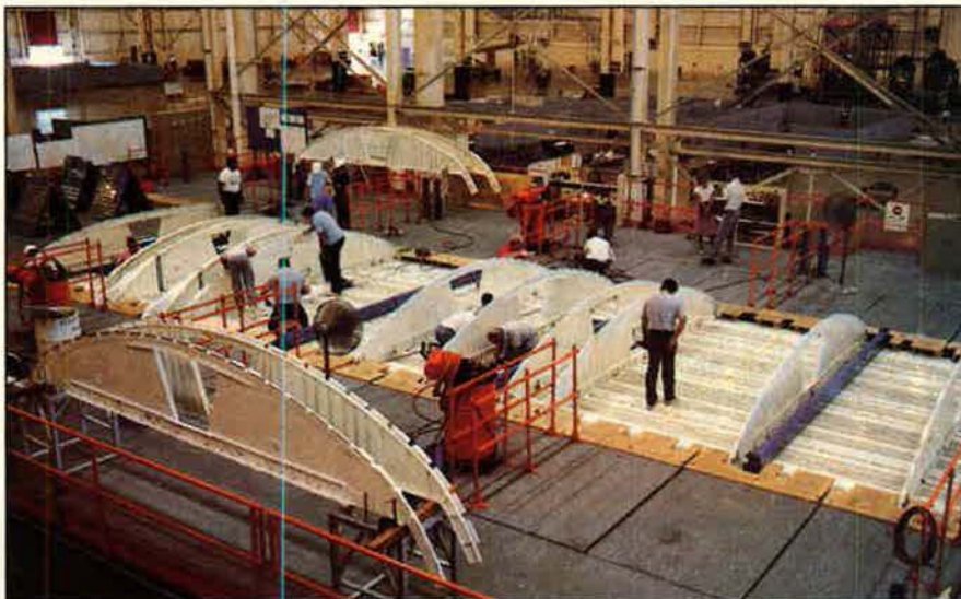
Workers attach underfloor bulkheads to the cargo floor of the first C-17A airlifter, now in production at the Douglas Aircraft plant in Long Beach, Calif. After the ribs and lower skin are attached, the entire assembly will be turned upright to finish the center fuselage. The aircraft is scheduled to roll out next August.
