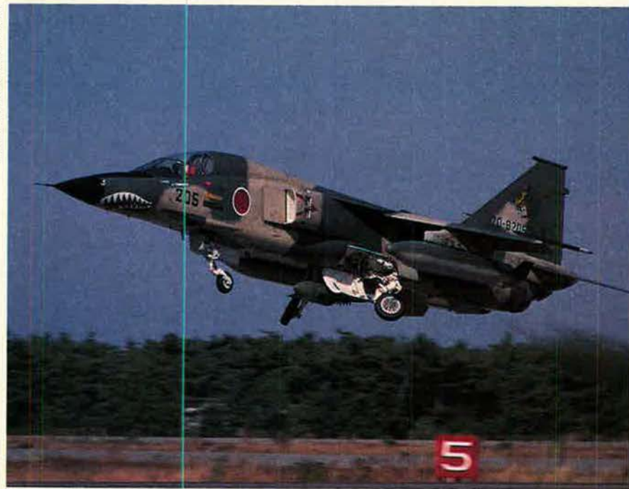
The Mitsubishi F-1, a made-in-Japan support fighter, will be replaced by advanced SX-3s in the 1990s. Deliveries of the single-seat, supersonic F-1s began in 1977. Powered by two Rolls-Royce engines, it can carry two air-to-surface missiles, 750-pound bombs, and four AIM-9 Sidewinder missiles.
