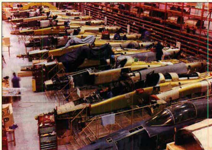
Bristol Aerospace Ltd. rolled out its first overhauled Canadian Forces CF-5 in August 21 ceremonies at its Winnipeg, Manitoba, plant. Canada operates fifty-six CF-5A/D aircraft (officially designated CF-116), a license-built version of the Northrop F-5A, mainly as lead-in trainers for CF-18 (F/A-18) pilots. Bristol will refurbish the CF-5s' wings, install new avionics and wiring, reinforce the dorsal longeron, and provide depot-level support for the planes.
