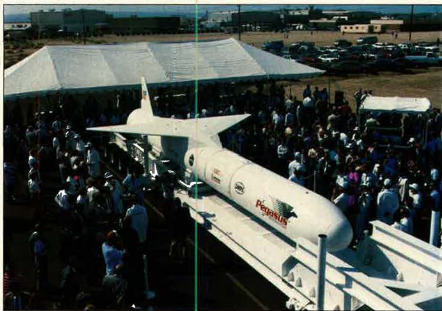
The first Pegasus air-launched unmanned space booster was rolled out at NASA's Ames-Dryden Flight Research Facility at Edwards AFB, Calif., in early August. Pegasus is designed to launch small payloads into a circular polar orbit.
