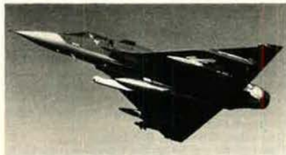
AS 30 L missiles and Atis pod on Mirage 2000
