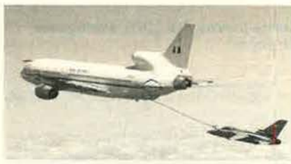
TriStar K. Mk 1 tanker refueling Tornado F. Mk 3
