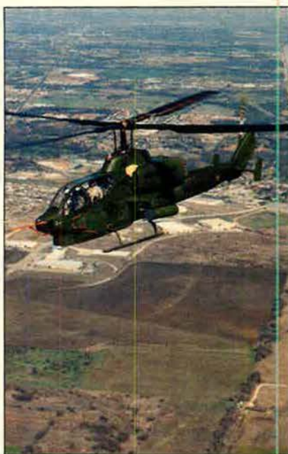
Bell Helicopter Textron's four-bladed AH-1W demonstrator has completed basic stability and safety-of-flight envelope expansion tests. This fall, it will be put through advanced maneuvers and aerobatics.
