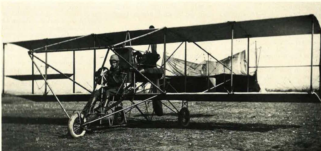
Lt. Harold Geiger in a Curtiss Pusher S. C. #8 airplane at San Diego, Calif., in 1913. Curtiss planes made use of wing-warping but employed independent ailerons for control. The Wrights' patent suits against Glenn Curtiss dragged on for eight years, outlasting their ownership of the Wright Co. and its patents and outlasting Wilbur himself.
