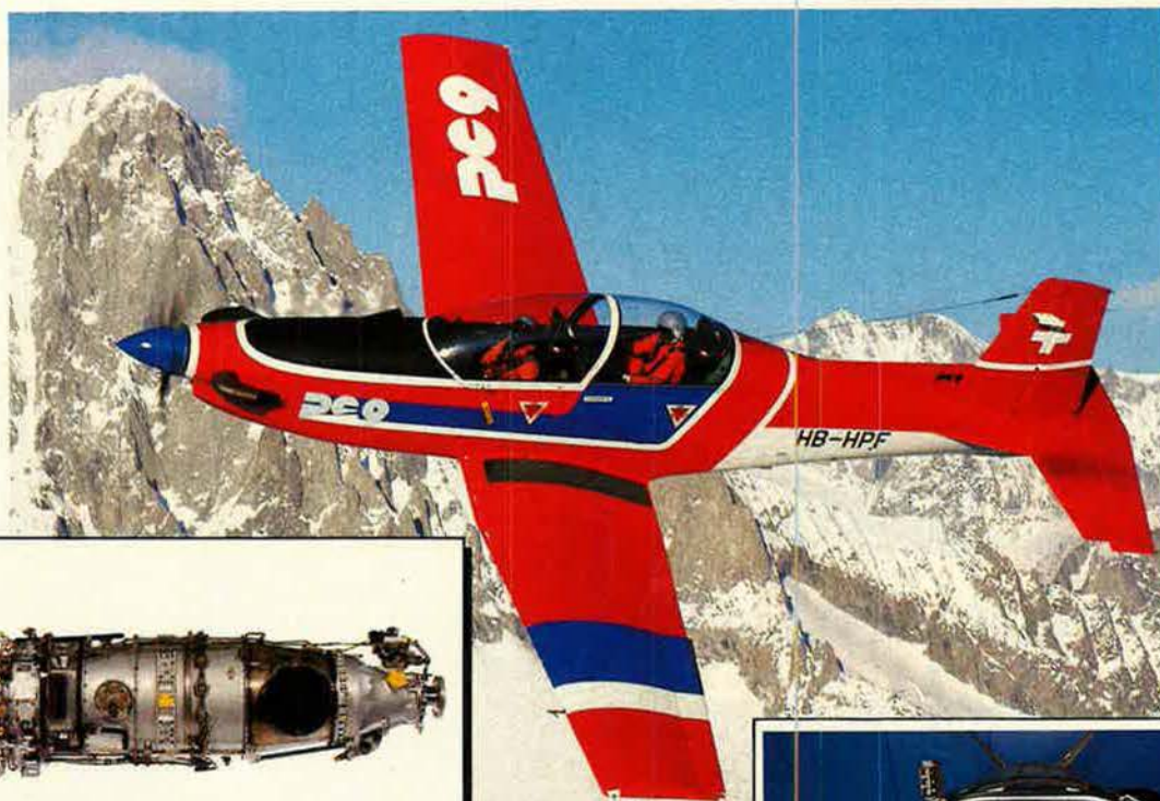
Latest technology 1,150 shp, derated to 950 shp, Pratt & Whitney PT6A-62 engine is fitted with electronic temperature and torque limiter.
