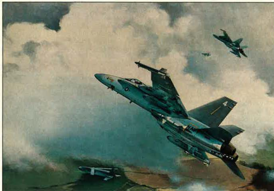
The team of McDonnell Douglas and Hughes was awarded a Navy contract for the demonstration and validation phase of the new Advanced Interdiction Weapon System, shown here being launched from an F/A-18. The baseline AIWS is an aerodynamically efficient, inertially guided glide weapon.
