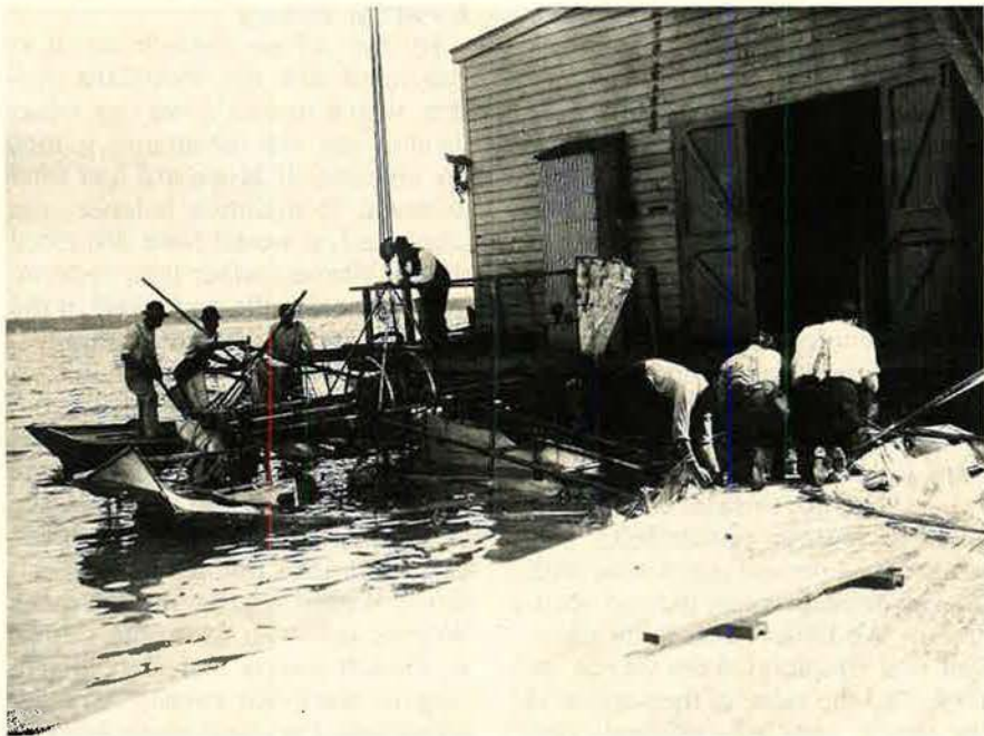
In an attempt to discredit the Wrights' claim by proving that Samuel Langley's aircraft could actually have flown in 1903, Curtiss rebuilt Langley's "aerodrome"—with improvements. Here, Langley's original is fished from the Potomac River after an unsuccessful attempt. In both of its 1903 flight tests, its wings collapsed.
