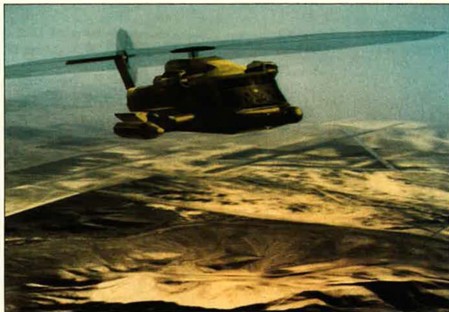
General Electric's Simulation and Control Systems Department will upgrade the Air Force's CH-3 simulator into an MH-53J weapon systems trainer. The MH-53J WST will use GE's Compu-Scene V image-generation system to provide realistic scenes (as shown here) to train pilots, copilots, and flight engineers.
