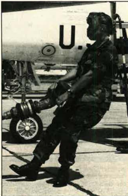
Nobody in the Air Force, neither T-41 pilot nor SR-71 pilot, flies without help from the people in the fuels section. A1C Pam Beaudoin handles the nozzle and hose of an R-9 refueling unit, preparing to fuel one of the T-38s of the 12th Flying Training Wing at Randolph AFB, Tex.
