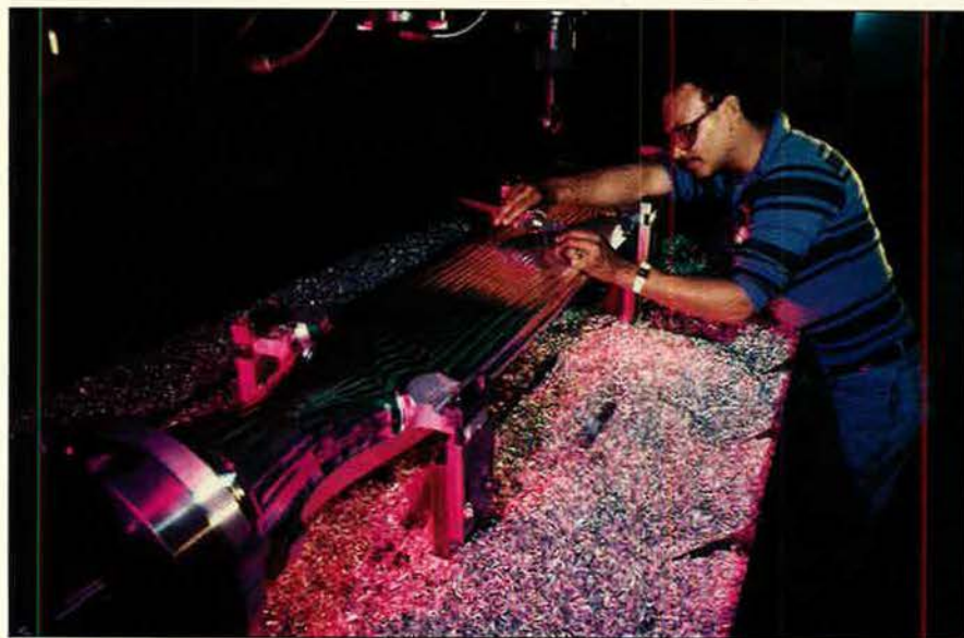
Hamilton Standard machine operator Angel Rodriguez profiles the first spar for the prototype 15WF-5 propeller system, which the company is developing for the Lockheed P-7A antisubmarine warfare aircraft that will replace the P-3 Orion. The five-bladed propeller will be fitted to the General Electric GE38 engine for the P-7A.
