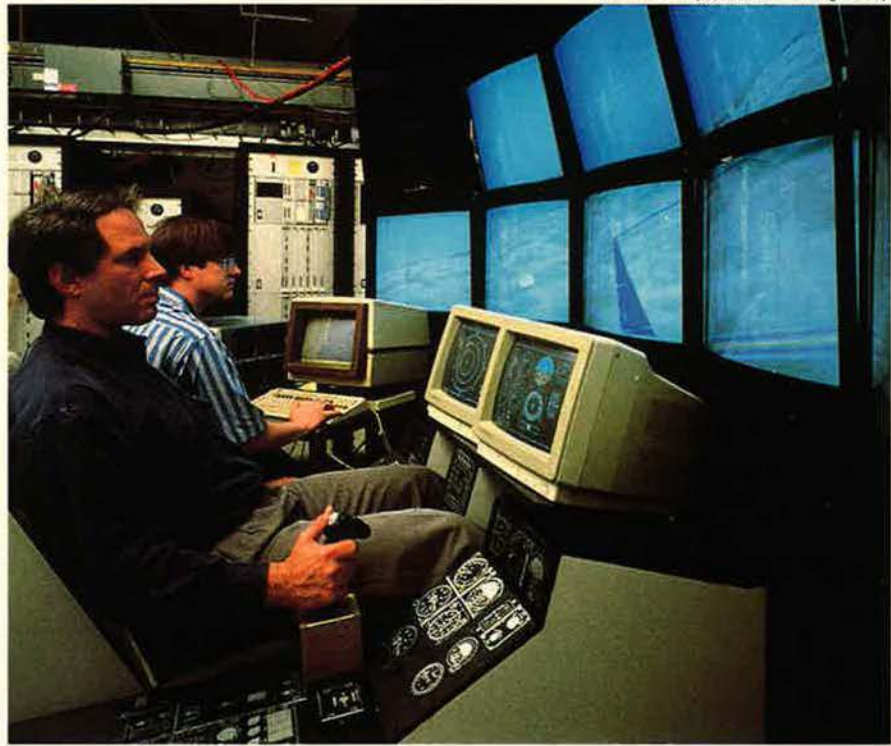
Simnet uses BBN's real-time computer image generation system to simulate the view from many types of vehicles. Using depth buffers, the computer stores data relating to factors such as perspective and speed and adjusts them to produce appropriate visual images. Here, a helicopter simulation is being developed.
