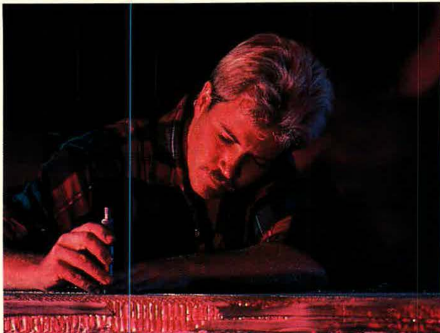
At the Sacramento Air Logistics Center, McClellan AFB, Calif., a quality assurance technician inspects a section of aircraft for structural weaknesses. AFLC "Stress Spectra Surveys" monitor strain on aircraft through a variety of tests.
