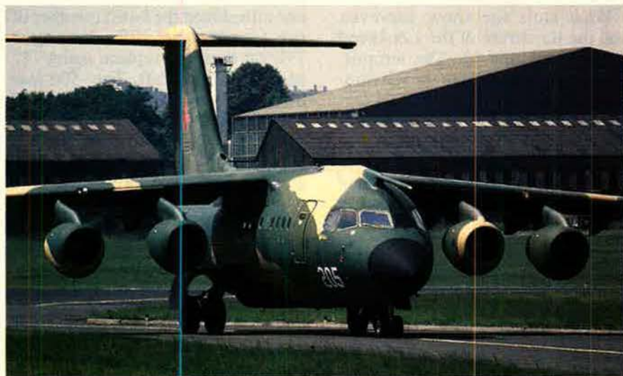
Several companies are producing turboprop commuter transports for the commercial sector and regional jets like this British Aerospace BAe-146 STA (STOL Transport Aircraft) with side-loading cargo door and in-flight refueling probe.
