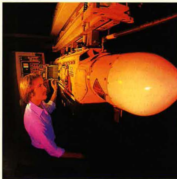
A Westinghouse ALQ-131 ECM pod is checked out by a company technician. The ALQ-131 is the jammer for a variety of combat aircraft and has been upgraded to meet the contemporary threat.
