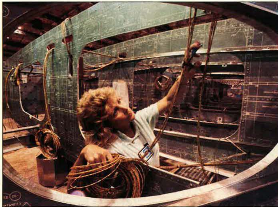
A worker at LTV's plant in Dallas, Tex., installs wire routing on the McDonnell Douglas C-17 airlifter's vertical stabilizer development fixture. The horizontal and vertical stabilizer development fixtures aid in routing all plumbing and wiring for hydraulic, electrical, and flight controls.
