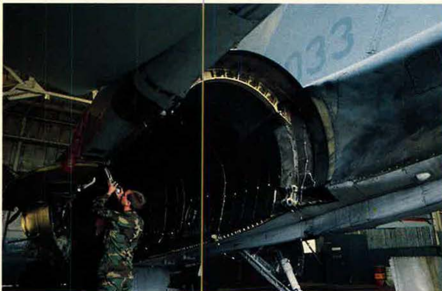
The 390th ECS at Mountain Home AFB, Idaho, represents the nonlethal side of electronic warfare—radar jamming. EF-111A crews can jam transmissions in several ways. Above, A1C John Moore and Sgt. Curtis E. Sargent prepare an EF-111 for one of the updated TF30-P-109 engines now being fitted to the Ravens.
