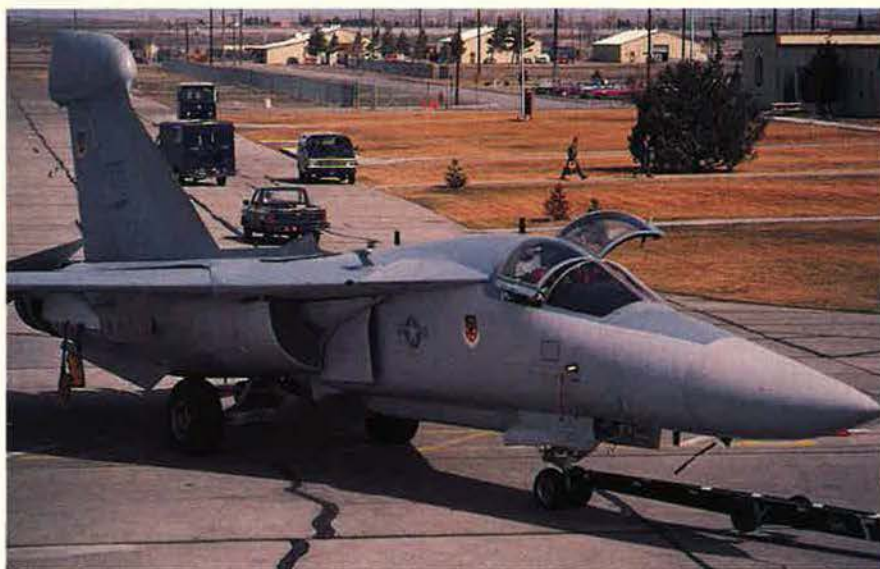
Mountain Home's EF-111s have one of the highest utilization rates in the Air Force. This Raven is being "Euked" (towed) from the maintenance hangars out to the flight line. The "football" on the vertical fin and the "canoe" on the belly house the receivers and transmitters that make the EF-111s so effective.
