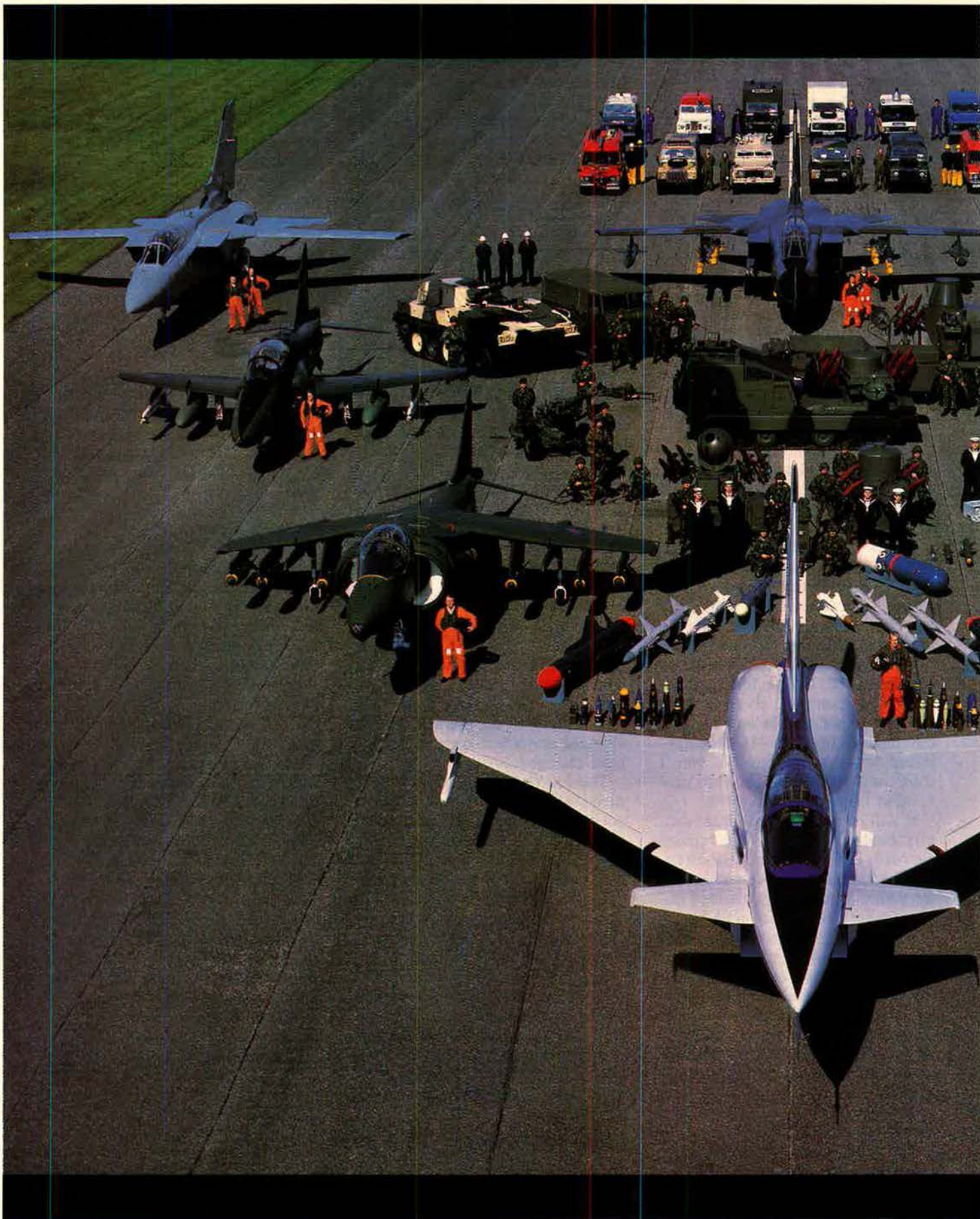
Displayed are: EAP (Experimental Aircraft Programme) – forerunner of the new European Fighter Aircraft, Harrier II GR.5 (advanced V/STOL fighter), Sea Harrier FRS.2, Hawk 100 (advanced jet trainer/strike aircraft), Hawk 200 (single-seat fighter), Torado ADV x 2 (Air Defence Variant), Tornado IDS (Interdictor Strike); Active Sky Flash, Bostead
