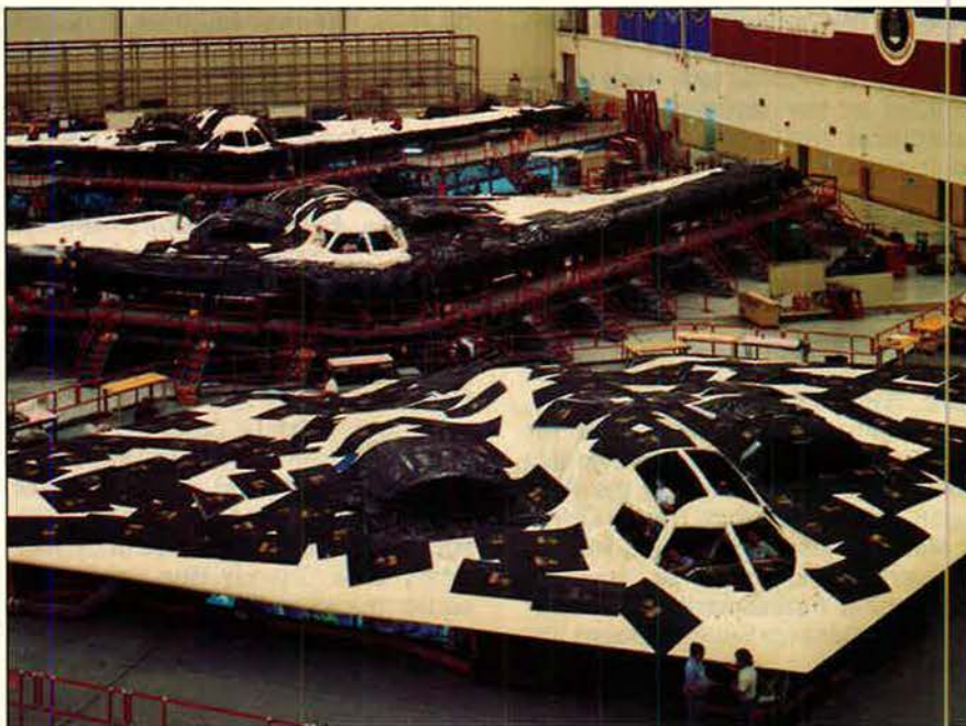
Using a three-dimensional electronic database, Northrop has eliminated "soft" (preproduction) tooling for the B-2 strategic bomber and is building the aircraft on "hard" or production tooling at Air Force Plant 42 in Palmdale, Calif. The mats and plastic wrap protect the B-2's composite skin during production.
