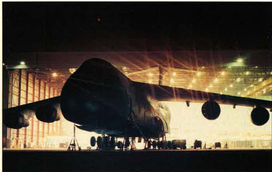
The last of fifty Lockheed C-5B Galaxy transports was delivered to the Air Force on April 17. The new C-5s have been averaging thirty maintenance man-hours per flight hour, well below the specified forty. Program responsibility for the C-5B has shifted from AFSC's Aeronautical Systems Division to AFLC.
