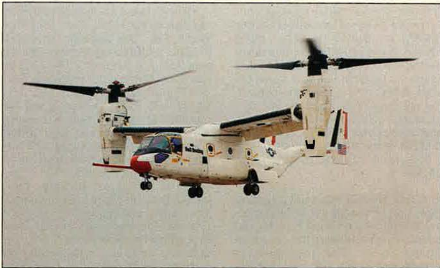
The Bell-Boeing V-22 Osprey tilt-rotor prototype made its first flight on March 19 at Bell Helicopter's Flight Research Facility in Arlington, Tex. The Osprey, which combines the vertical capabilities of the helicopter with the speed of a fixed-wing aircraft, will be used by the Marines, Navy, and the Air Force.
