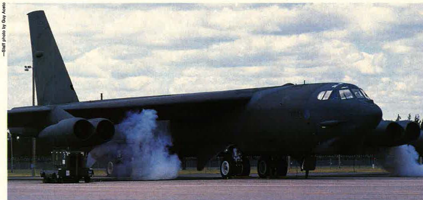
Systems modifications and superb maintenance combine to enable thirty-year-old B-52s to continue to pull twenty-four-hour-a-day alert duty. This B-52H is starting its engines in an alert pad test at K. I. Sawyer AFB, Mich. SAC's 410th Bomb Wing at Sawyer will be the first SAC unit to receive the new AGM-129A Advanced Cruise Missile.
