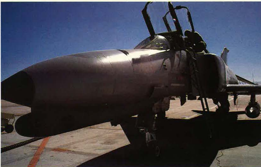
F-4G "Wild Weasel" aircraft like this one from the 561st Tactical Fighter Squadron, George AFB, Calif., are especially designed for radar suppression. The 37th TFW takes part in as many exercises as it can in an effort to maintain TAC's electronic combat capability at a constant peak.
