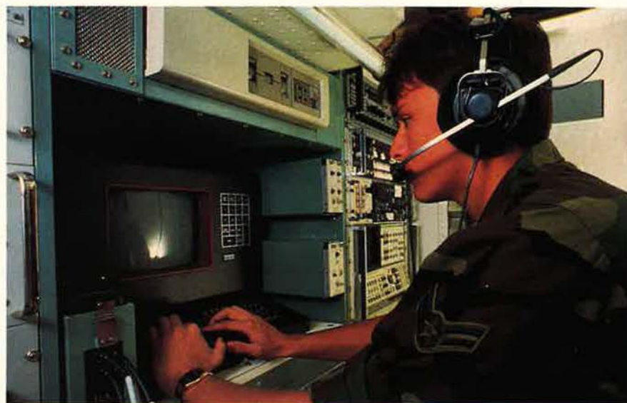
A1C James Coffey of Detachment 3, 695th Electronic Security Wing, Nellis AFB, Nev., manually operates a multiband jammer of the sort used in USAF's "Red Force" program, a training effort to emulate a hostile electronic combat environment for the realistic training of aircrews, weapons controllers, and other communicators.
