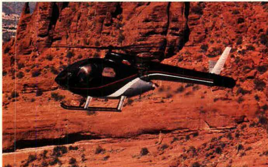
McDonnell Douglas/Bell's LHX will carry a NOTAR ("no tail rotor") system mounted under a conventional tail. The system, proven in a modified OH-6A helicopter (above), forces low-pressure air through a slotted tailboom to a thruster to counter torque and control direction.
