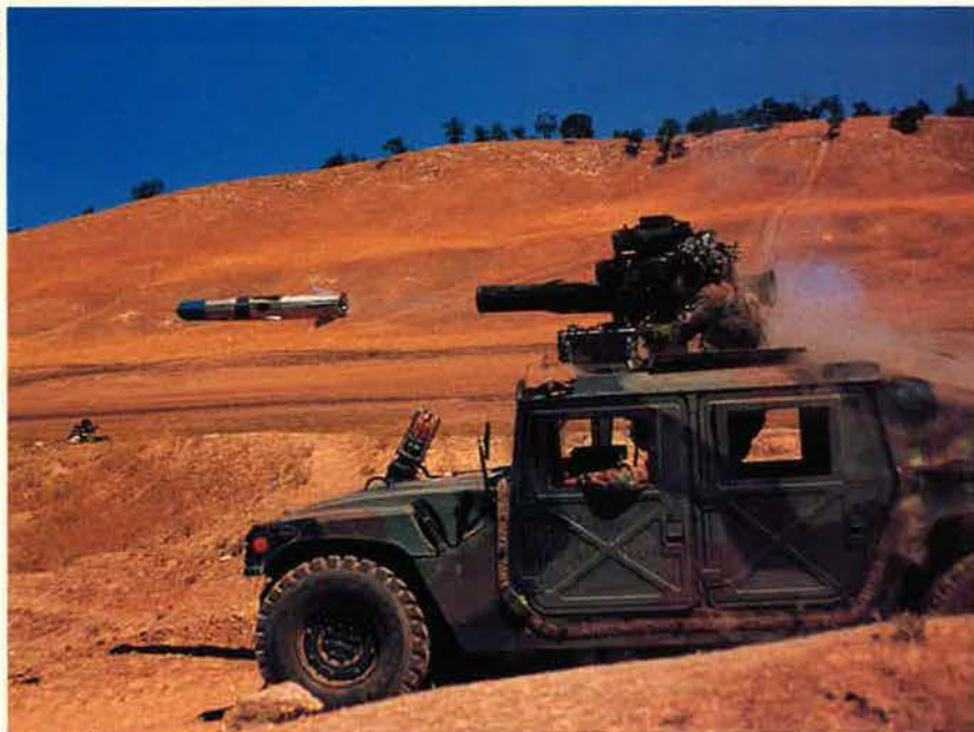
The advent of the TOW (tube-launched, optically tracked, and wire-guided) antitank missile in the 1970s marked the start of something big in land warfare. The venerable TOW missile has been followed into the field by an ever-wider assortment of antitank weapons of increasing sophistication and lethality.
