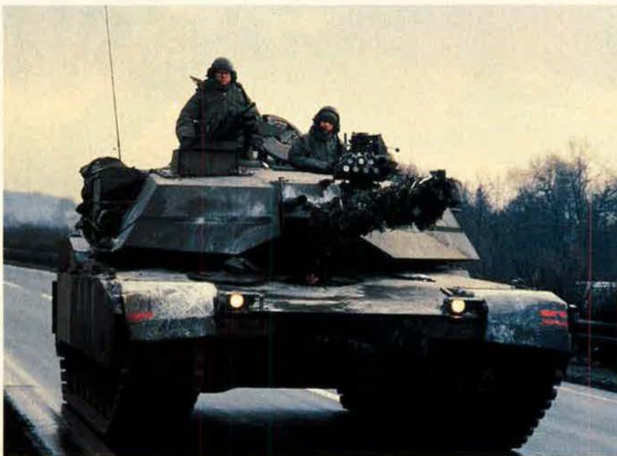
Like tanks everywhere, the US Army M1 main battle tank is most heavily armored on the front and sides. Soviet tanks are now being given the added advantage of reactive armor in these areas. When struck by a shell, reactive armor keeps the shell from penetrating the tank by counterexploding against it.
