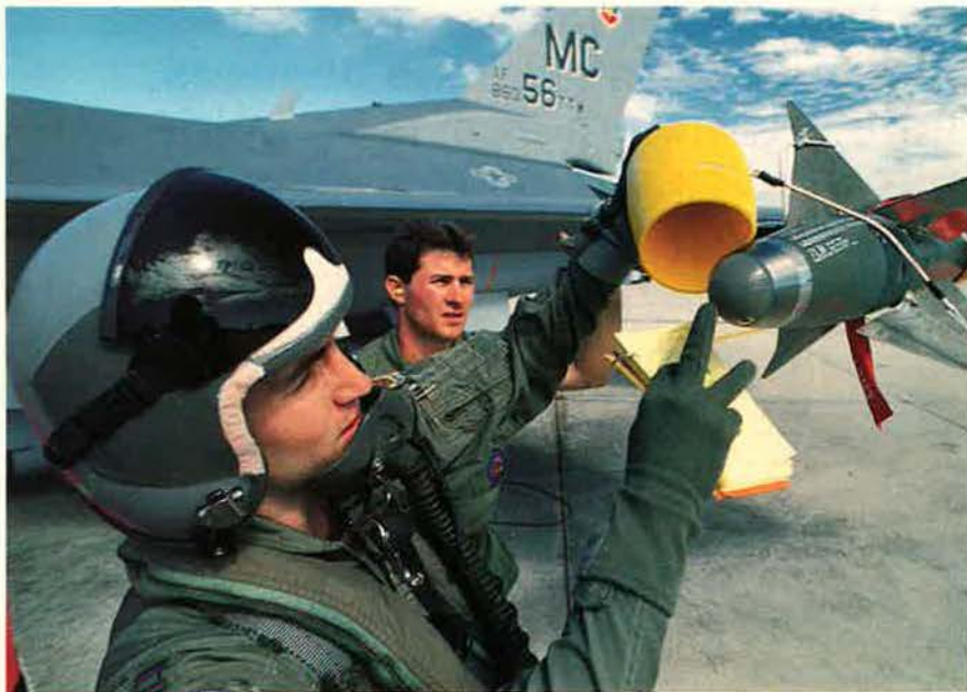
Money spent on modernization through the 1980s has left tactical forces in impressive condition. Most obvious has been a steady phaseout of Vietnam-era F-4s in favor of newer aircraft, such as this F-16 of the 63d Tactical Fighter Training Squadron, MacDill AFB, Fla., armed with an AIM-9 Sidewinder air-to-air missile.
