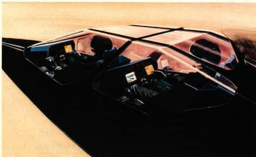
Central to the First Team's LHX concept is a two-pilot cockpit whose flexibility will allow one pilot to accomplish most missions. Both teams' designs will use advanced technology to relay information to multifunction displays rather than to individual cockpit instruments.
