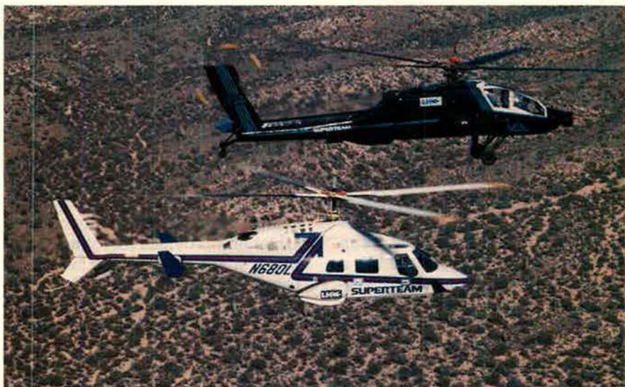
Advanced flight technologies demonstrated in these aircraft will become part of the Superteam's LHX design. That design includes a four-blade, bearingless rotor blade based on the 680 Rotor System of the Bell 222 (foreground) and an advanced flight control system similar to that of the Army's McDonnell Douglas AH-64A Apache prototype, modified for advanced cockpit technology evaluation.
