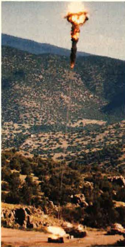
An indirect-fire SADARM weapon descends along a ballistic trajectory to a point above a tank—having found it via radar—and then blasts a self-forging fragment warhead into the top of the target.
