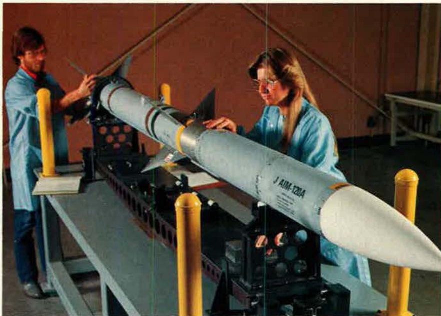
AMRAAM —the Advanced Medium-Range Air-to-Air Missile—is seen as a near-term high priority for air-to-air forces. The missile, shown here at the Hughes facility in Tucson, Ariz., would greatly extend the fighting range of current and future fighters. Raytheon is the second-source manufacturer.
