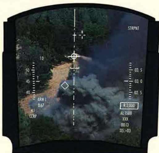
ATHS provides data for such HUD symbols as target I.D., range and steerpoint.
