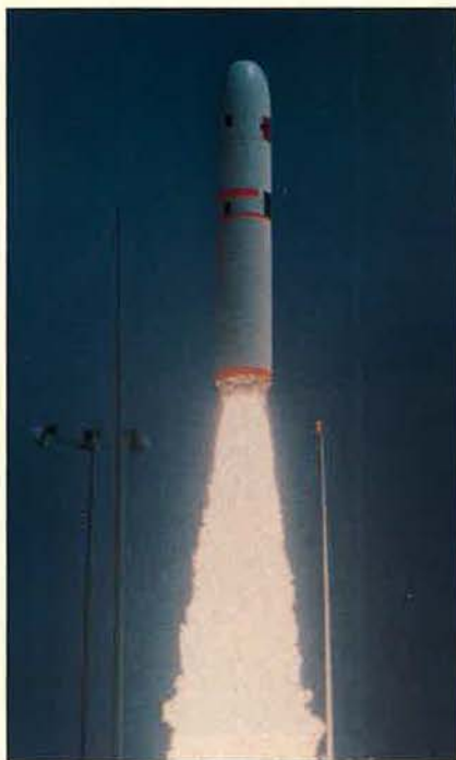
The Navy has nearly completed pad tests of the Lockheed UGM-133A Trident II, or D5, sea-launched missile. Shown is an early test missile being launched from Cape Canaveral AFS, Fla.
