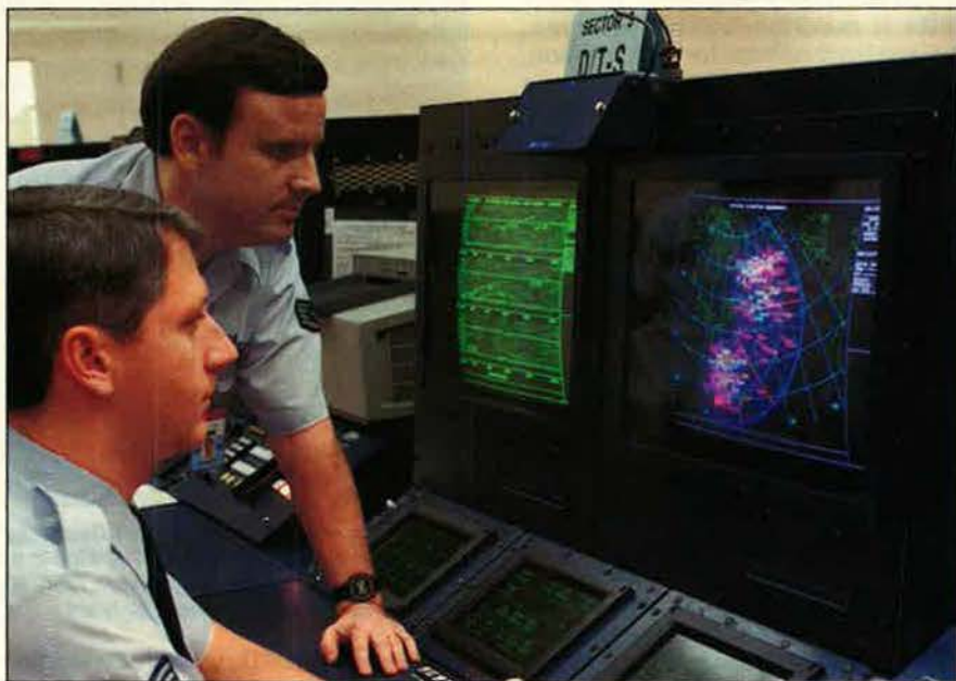
GE's Over-the-Horizon Backscatter (OTH-B) radar enables these two Air Force operators to monitor the entire east coast of North America from the radar's operations center in Bangor, Me. Tactical displays like that at right show aircraft and flight plans within the radar's 180-degree, 1,600,000-square-mile coverage area. OTH-B will be turned over to the Air Force this fall.
