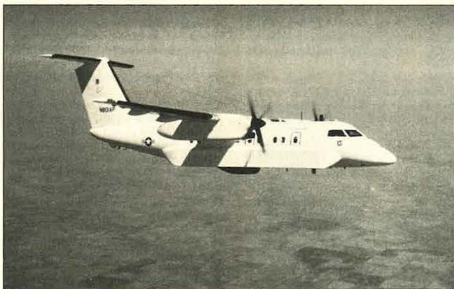
The 475th Weapons Evaluation Group, based at the Air Force Air Defense Weapons Center at Tyndall AFB, Fla., recently received the first of two E-9A airborne platform telemetry relay aircraft. The de Havilland Dash-8's sensor suite was developed by the Sierra Research Division of LTV.
