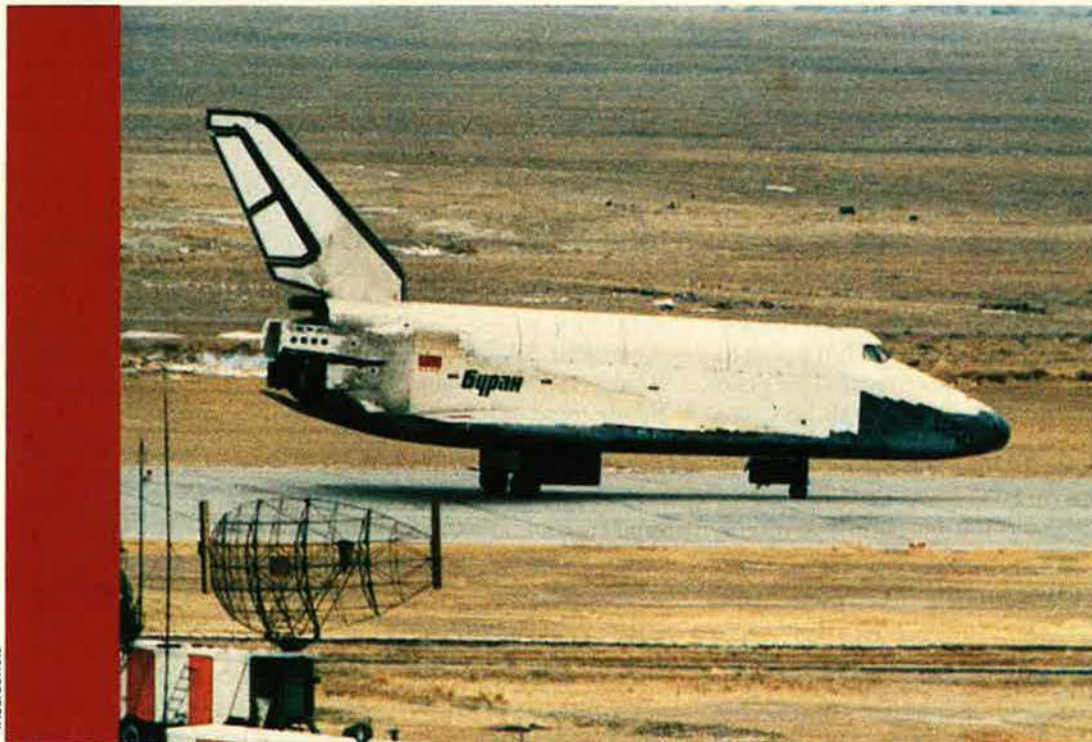
At the end of its two-orbit mission, Buran landed on a specially constructed runway at Tyuratam near the Aral Sea. The Soviet shuttle also used a drag chute to slow it down once on the runway. Buran's computer-controlled first flight stunned many Western observers.
