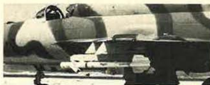
AA-2D (NATO 'Atoll') missile on MiG-21RF of Egyptian Air Force (Denis Hughes)
