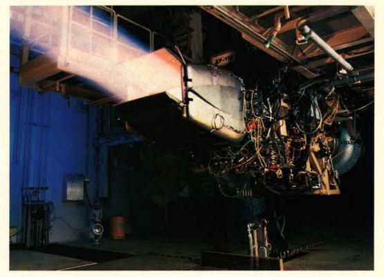
A version of the Pratt & Whitney YF119 powerplant, featuring a two-dimensional exhaust nozzle, undergoes sea-level testing at the company's West Palm Beach facility. Use of these kinds of nozzles on the aircraft is expected to give ATF great maneuverability and responsiveness in air combat.
