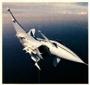
Flight test for the BAe Experimental Aircraft Program technology demonstrator went well last year, as the aircraft was flown up to Mach 1.6 + in 130 flight hours. The EAP aircraft is shown here during its handling trials.
