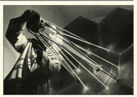
Conventional monolithic primary mirrors for very large reflecting astronomical telescopes now weigh so much that they have become impractical. Dr. Kenneth Lorell, a Lockheed physicist, works with the Advanced Structures/Controls Integrated Experiment in Palo Alto, Calif. The experiment will help Lockheed to develop lighter-weight, segmented, computer-controlled primary mirrors that are accurate to within a few billionths of a meter.
