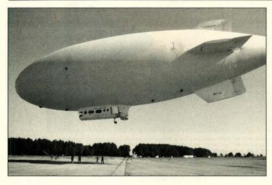
The world's first full-authority, fiber-optic control system was flown on this Airship Industries Skyship 600 at the company's Elizabeth City, N. C., plant. The airship will undergo intensive flight testing to evaluate the system. The Navy expects to incorporate a fly-by-light system into its Operational Development Model airship program. The program is being restructured under DARPA.
