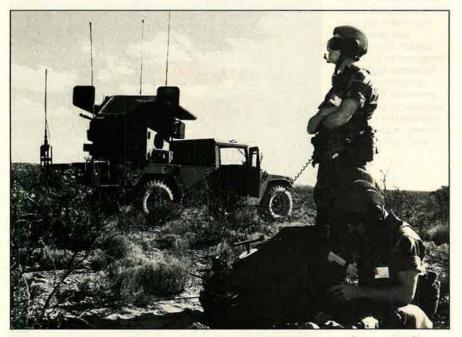
Hummers also serve as the chassis for the new Pedestal-Mounted Stinger (PMS) vehicles, delivered to the Army last November. The man-held, surface-to-air FIM-92 Stinger missiles can be fired either from the turret (under the vehicle's three antennas) or, as shown here, from the remote control unit, which can operate the fire unit from up to fifty meters away.
