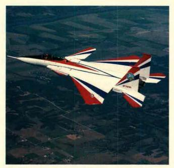
The McDonnell Douglas F-15 STOL Maneuvering Technology Demonstrator (SMTD) flew for the first time last fall. It will soon be fitted with vectoring nozzles and will begin the second part of its two-phase flight-test program this summer.
