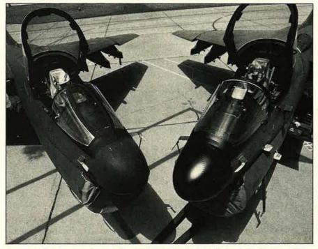
A new single-piece windscreen for the LTV A-7 jet (right) is being tested by the 162d Tactical Fighter Group, ANG, in Tucson, Ariz. The new windscreen, made of multilayered polycarbonate between two layers of acrylic, improves visibility by twenty percent, requires thirty percent fewer spare parts to maintain, and offers greatly improved birdstrike protection. AFSC's Aeronautical Systems Division is managing development and flight testing.
