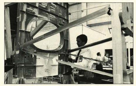
Assembly of the first Rockwell/Messerschmitt-Bölkow-Blohm X-31 Enhanced Fighter Maneuverability (EFM) demonstrator began last November 14 at Rockwell's North American Aviation plant in Palmdale, Calif. Shown here is the forward inlet bulkhead that was secured to the plane's assembly jig. Under the auspices of DARPA/Naval Air Systems Command and the Federal Republic of Germany, two X-31 aircraft will be built. The first is expected to fly later this year.
