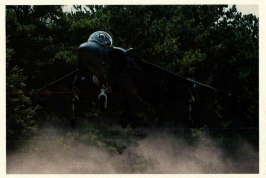
The Marine Corps AV-8B Harrier II was the first aircraft to embody fiber optics for data handling, not for flight control. Mc-Donnell Douglas is now considering the use of flight-control fiber optics in Its Navy F/A-18 and in a night-attack version of its AV-8B.
