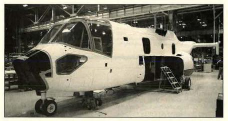
The canopy for the first Bell-Boeing V-22 Osprey flight-test article was recently installed at Boeing's Philadelphia, Pa., facility. The canopy frame is constructed of titanium and weighs 160 pounds, excluding the transparencies, which are resistant to birdstrikes. The flight-test article was later shipped to the Bell Helicopter plant in Fort Worth, Tex., where it will get its wings and engines. First flight is scheduled for the middle of this year.
