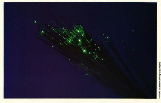
This photo shows how single-mode optical fibers can literally light up a communications or datahandling system. Lower attenuation of the signal and greater resistance to EMI and EMP are two advantages of singlemode fibers over earlier multimode varieties.
