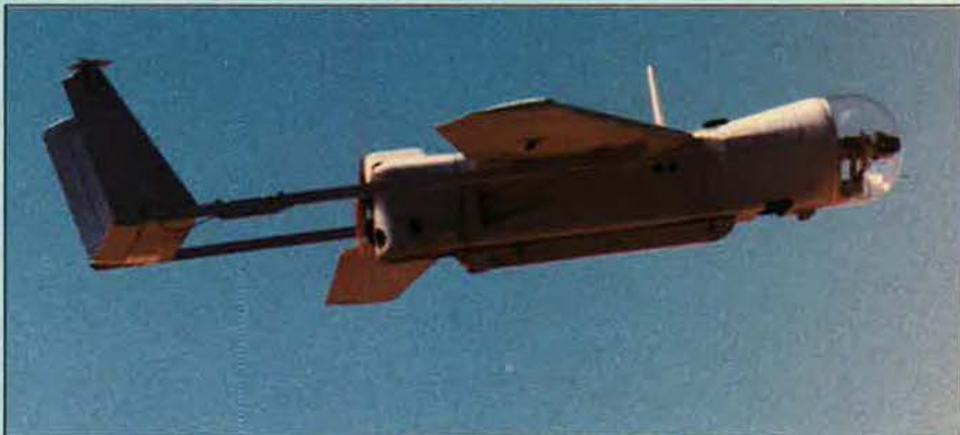
LSI/DS SkyEye R4E-40 RPV, used operationally by US Army in Central America
