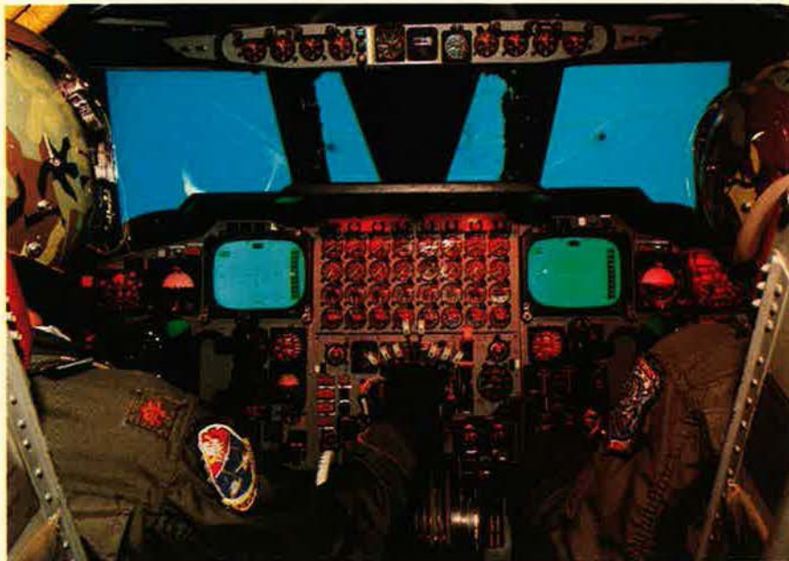
Air Force pilots practice aerial refueling while "flying" a B-52 simulator that shows a KC-135 tanker, as if for real, in one of their out-of-the-window scenes. Such computer-generated images are the stuff of modern simulators.
