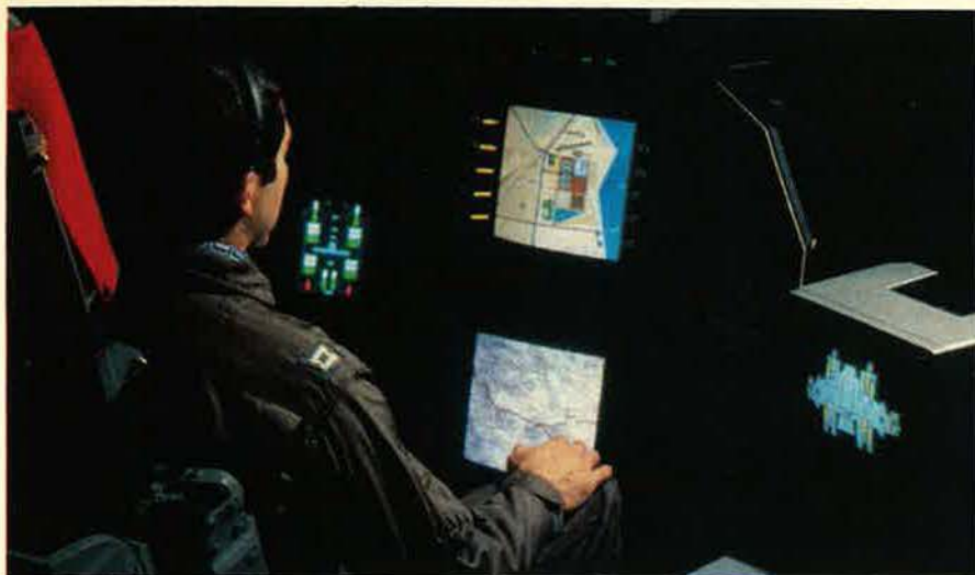
The Microprocessor Application of Graphics with Interactive Communications (MAGIC) simulator (here operated by Capt. Keith Beachy) is an example of the high technology that is making the pilot's job simpler, not more complex. It will enable command of certain aircraft by voice alone.
