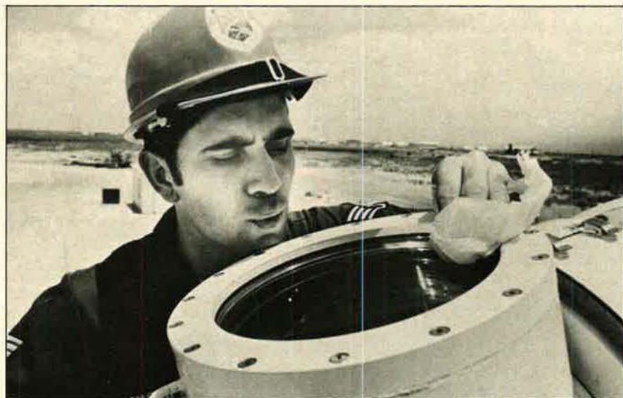
At Holloman AFB, N. M., a technician polishes a ten-inch-diameter telescope that is part of Electronic Systems Division's solar electro-optical network (SEON). The recent opening of an observatory at San Vito, Italy, completed the network.
