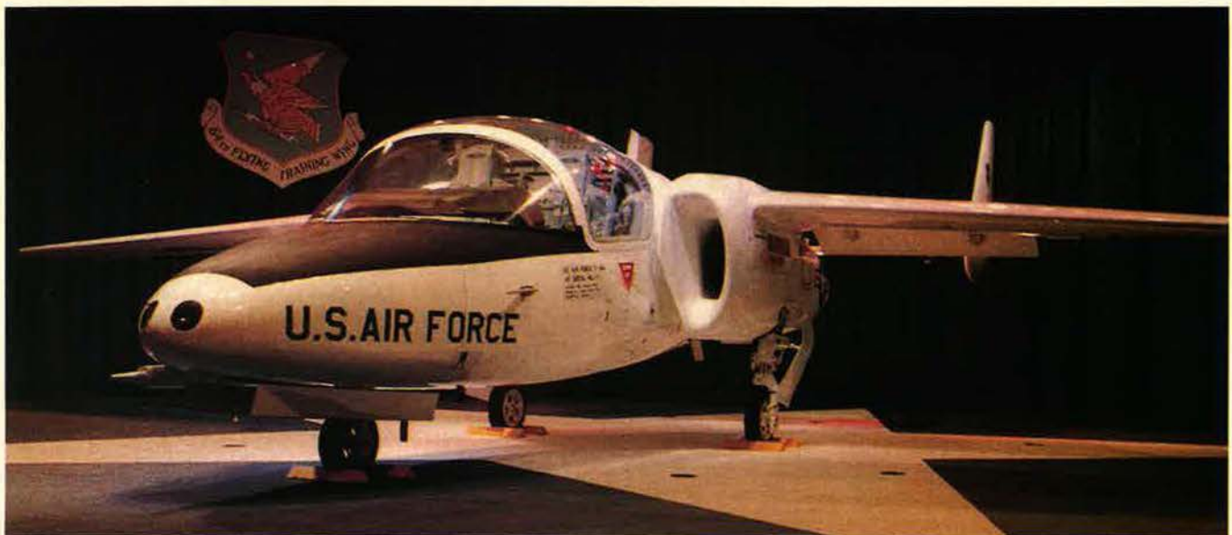
When it was roiled out in early 1985, the Fairchild T-46A was scheduled to be the Air Force's first new primary trainer in thirty years. The airplane features side-by-side seating in a pressurized cockpit and two engines.
