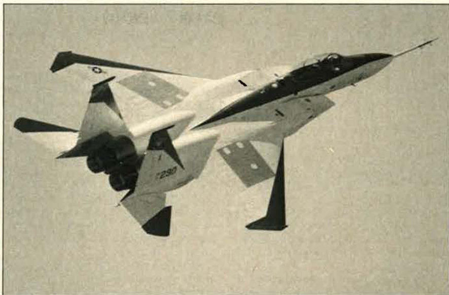
A McDonnell Douglas F-15 recently flew for the first time with wing panels made from a new aluminum-lithium alloy. The panels made of the new alloy are five percent stronger and nine percent lighter than the all-aluminum parts they replace.
