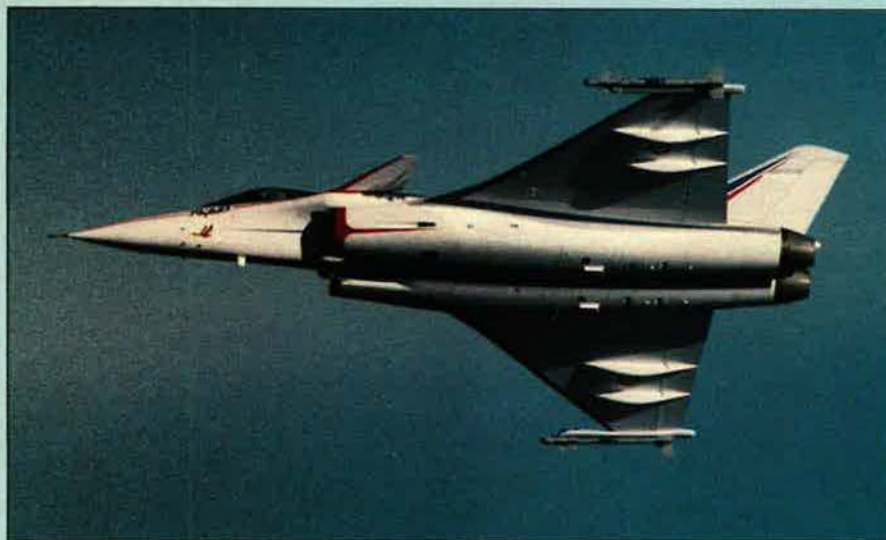
The Rafale A, like BAe's EAP, is intended primarily as a technology demonstrator for the planned production Rafale B
