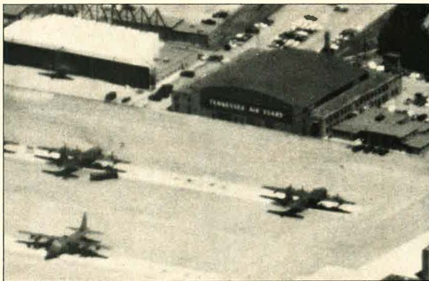
A KS-127 Long-Range Oblique Photography Camera took this photo of the Tennessee ANG ramp, shown in 12X enlargement. This photo was taken from an altitude of 35,500 feet and from a distance of twenty-two nautical miles.
