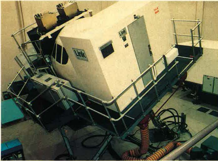
An Air Force B-52 simulator duplicates maneuvers anticipated for the bomber's crews on combat missions. B-52 "weapon system trainers" are being upgraded to correspond with modifications of B-52 avionics, in keeping with USAF's drive to make its simulators as modern as its aircraft.
