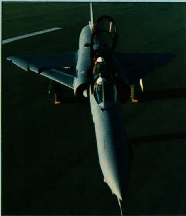
The Cheetah has many design features in common with the Israeli Kfir, but retains an Atar engine
