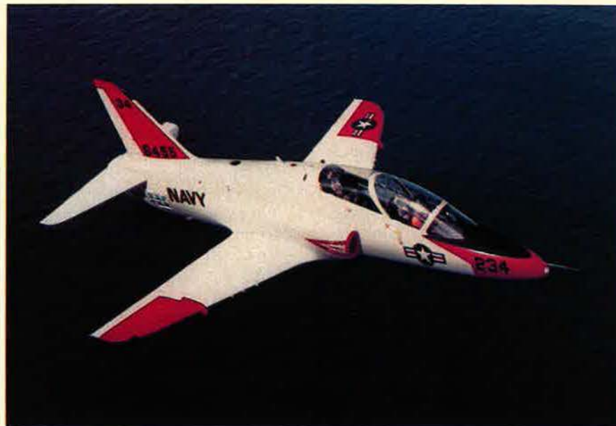
McDonnell Douglas and British Aerospace are teaming up to build the Navy’s new trainer, the T-45A Goshawk. Removing the T-45’s arresting hook and replacing its dual nosewheel, neither of which the Air Force needs, would save roughly 800 pounds of weight.
