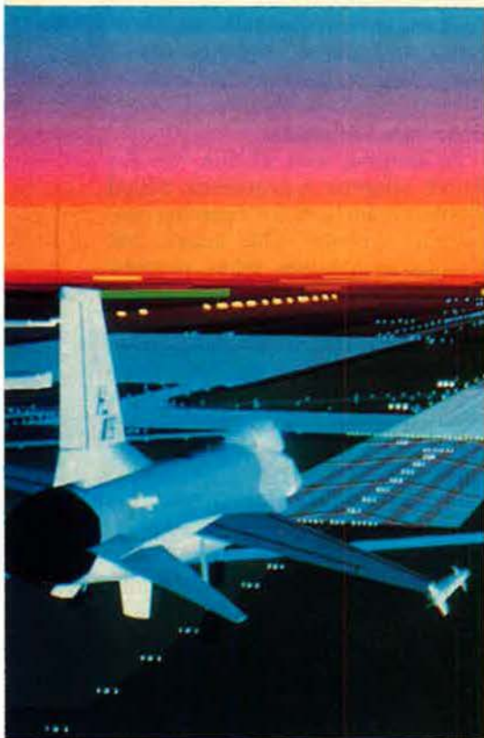
Computer-generated visual systems have vastly broadened the scope and utility of USAF's simulators. This Singer-Link digital image generation (DIG) system depicts a final approach.
