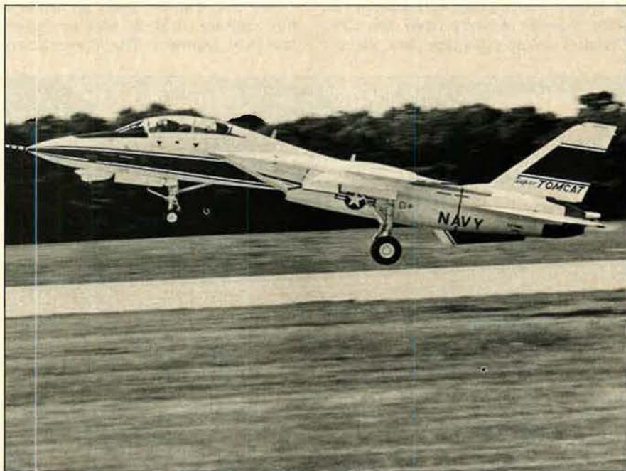
The Navy's newest Tomcat took to the air for the first time in late September as the first Grumman F-14A Plus aircraft lifted off from the company's Calverton, N. Y., test facility. It features two General Electric F110-GE-400 engines and improved avionics. Fleet deliveries of the new Tomcat will begin in late 1987.
