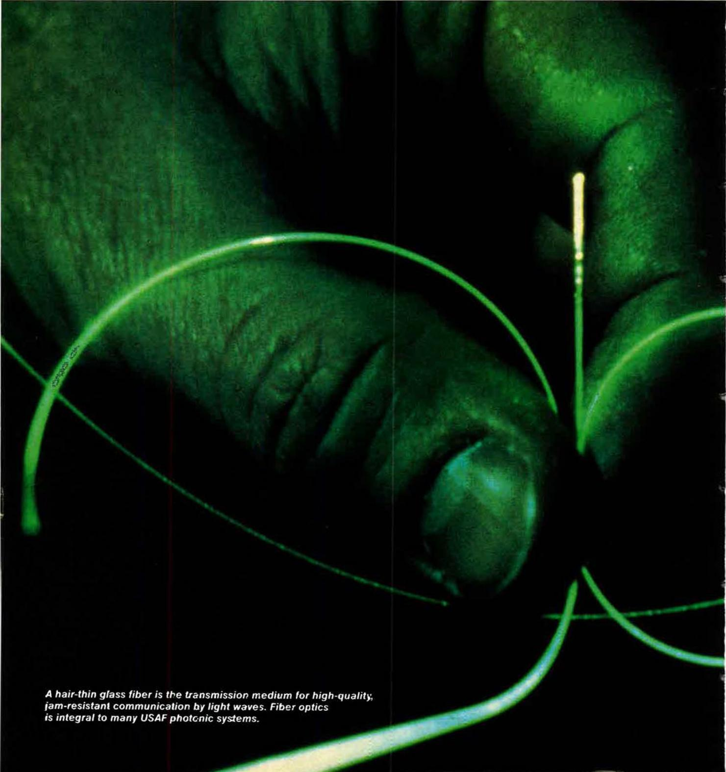
*A hair-thin glass fiber is the transmission medium for high-quality, jam-resistant communication by light waves. Fiber optics is integral to many USAF photonic systems.*
