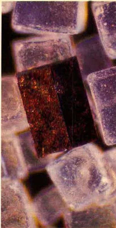
*Grains of salt surround a semiconductor laser. The device, developed by Bell Labs, can be tuned to emit a range of ultrapure light frequencies.*
