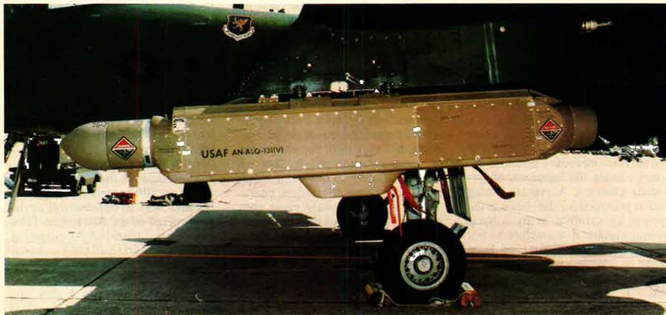
A-10 aircraft can carry the Westinghouse AN/ALQ-131 electronic countermeasures pod. The newest version of the pod, the Block II, has posted an excellent reliability and availability record during operational tests.
