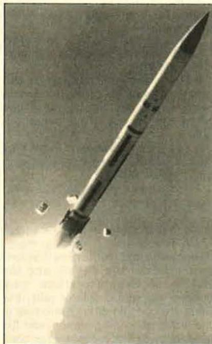
*On April 20, the Army's Flexible Lightweight Agile Guided (FLAG) Experiment Program hypersonic test vehicle, shown above at launch, destroyed an aluminum sphere suspended below a balloon at 15,000 feet. The FLAG program is part of the SDI effort.*
