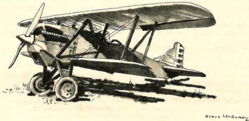
*Forerunner of the P-12 was the earlier PW-9, Boeing's first fighter design. It had a 21,000-foot ceiling, top speed of nearly 160 mph, and range of 390 miles.*
