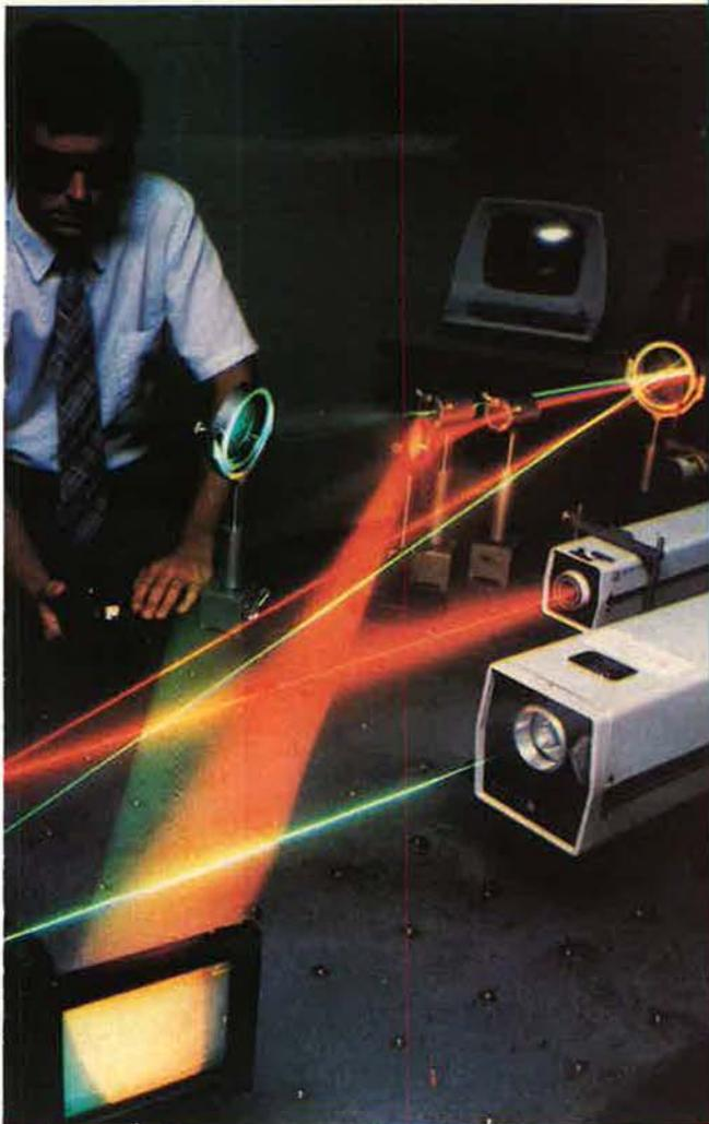
*Dr. Steve Butler of AFSC's Armament Division produces a target-seeking hologram. Future missiles may carry a small lightweight optical computer on board that can compare holographic imagery of preselected targets to objects on a battlefield. The autonomous missile will home in on and destroy only the specified target. The system is being tested now at Eglin AFB, Fla. (US Air Force photo)*
