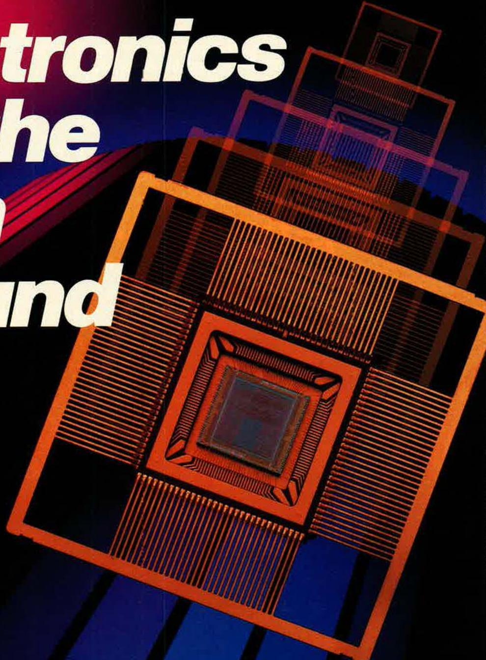
Densely layered VHSIC chips such as this Westinghouse "10K configurable gate array" device will enhance the reliability and performance of USAF's electronic systems.
