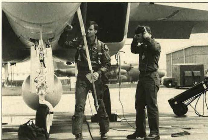
Maj. Kevin Chilton (left) and SSgt. Bernard Keller of the 3247th Test Squadron at Eglin AFB, Fla., preflight the first Joint Tactical Information Distribution System (JTIDS)-equipped F-15A prior to its initial flight in late March. JTIDS will provide quick and secure communications in a battlefield situation.
