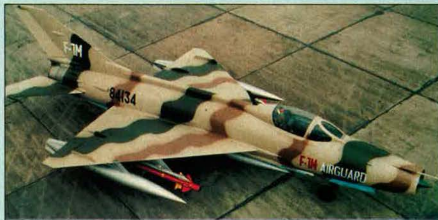
British avionics and the latest Chinese air-to-air missiles are features of the Xian F-7M Airguard export fighter
