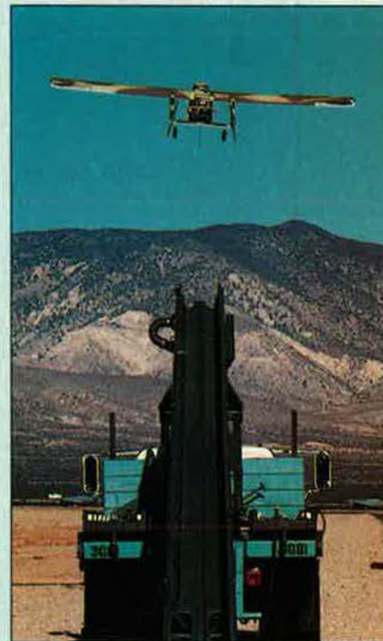
Mazlat/AAI Pioneer RPV can utilise catapult launcher in restricted areas or from shipboard
