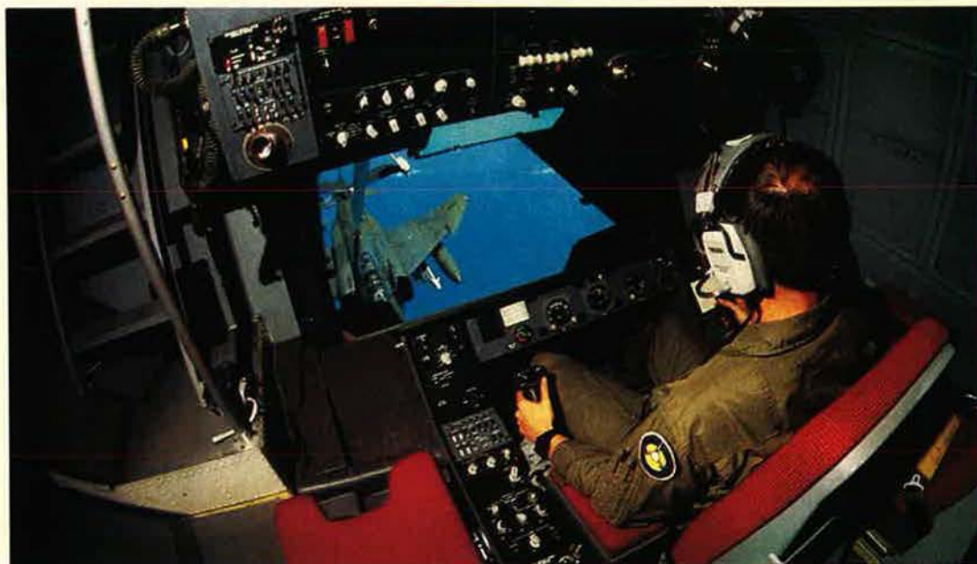
The boom operator's compartment on board a KC-10 Extender offers fly-by-wire controls, superb visibility, and environmental amenities not found on older KC-135s. The operator can also control a permanently mounted drogue system to refuel Navy and allied aircraft. The "boomer" doubles as loadmaster for the dual-role KC-10. (USAF photo by SSgt. Lee Schading)
