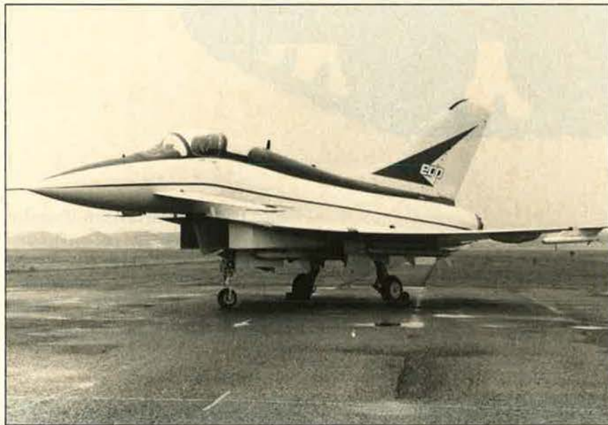
The Experimental Aircraft Program (EAP) technology demonstrator was rolled out on April 16. The vehicle incorporates a number of advanced technologies; the knowledge gained from this program should prove beneficial in the new European Fighter Aircraft.
