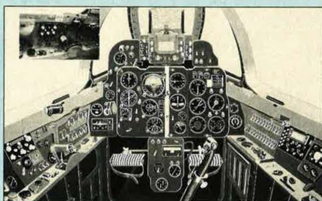
Modernised cockpit of the F-7M Airguard includes a HUDWAC (head-up display and weapon aiming computer)
