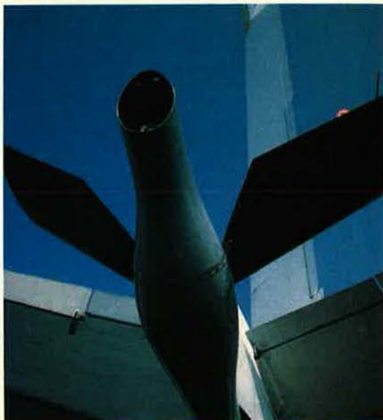
The business end of the KC-135 can pass 900 gallons of jet fuel a minute to a receiver aircraft. USAF's Aeronautical Systems Division is looking at improving the boom system with higher flow fuel pumps, a new nozzle, and a load-indication system. (USAF photo by "O. C." Carlisle)
