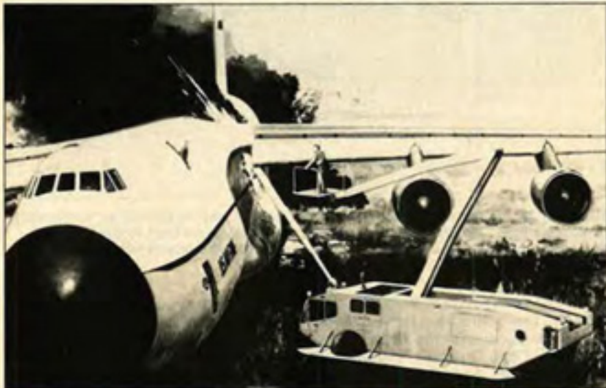
This is an artist's concept of the new crash/rescue vehicle being developed for the Air Force by Bell Aerospace Textron, Inc., and ASD's Flight Dynamics Laboratory at Wright-Patterson AFB, Ohio. The new truck will combine air cushion technology and conventional-wheel drive.
