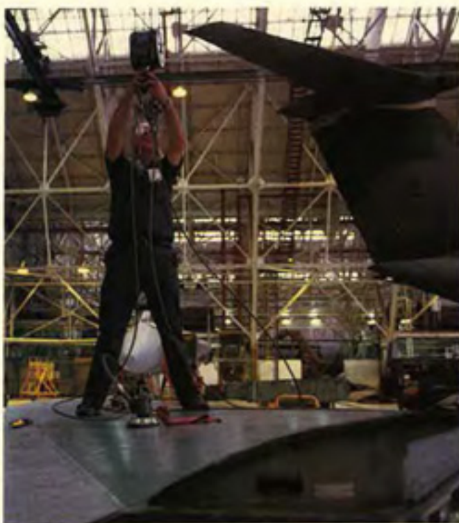
At the Warner Robins Air Logistics Center at Robins AFB, Ga., mechanic John Belflower attaches a sling to the wing of an F-15 for installation on the aircraft. AFLC operates five such centers for maintenance of all major operational systems.
