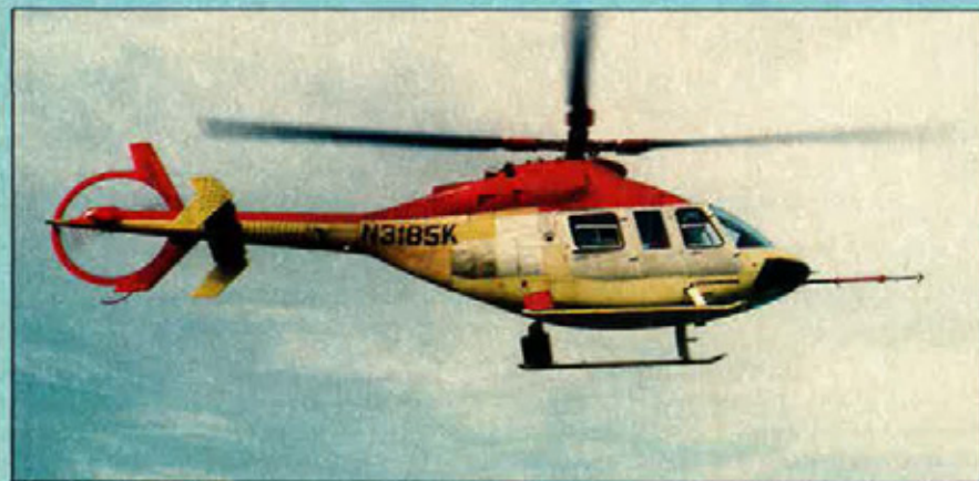
Pre-production Model 400 TwinRanger in flight test configuration
