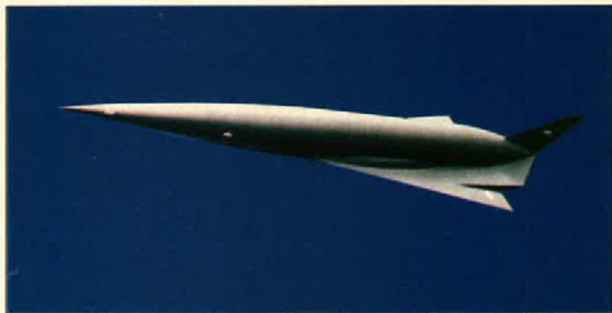
One of the concepts explored by Project Forecast II is the National Aerospace Plane (NASP), which would be the first conventional takeoff-to-orbit vehicle.
