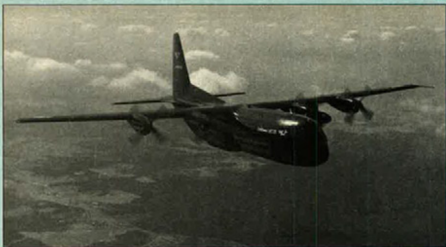
Lockheed-Georgia's all-black high technology testbed (HTTB) conversion of an L-100-20 Hercules
