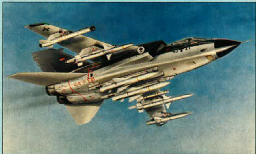
MBB artist's impression of ECR Tornado in German Navy insignia, with Kormoran anti-ship missiles under the fuselage, HARM missiles underwing (inboard), and outboard pylons occupied by a chaff/flare dispenser (port) and ECM pod (starboard)
