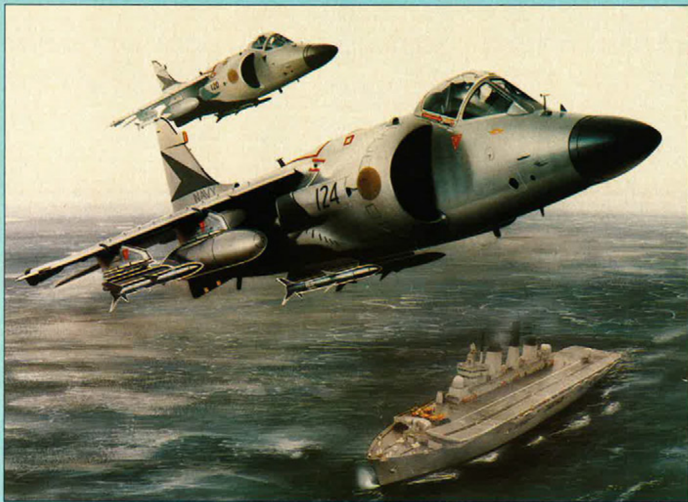
Artist's impression of the midlife updated BAe Sea Harrier FRS. Mk 2, armed with four AMRAAM missiles
