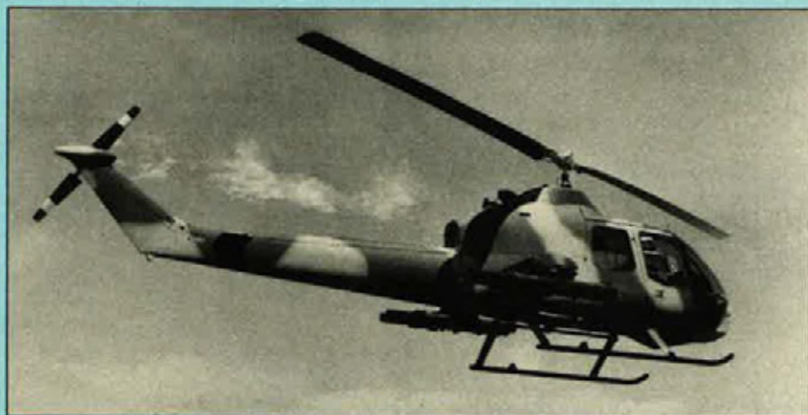
Armament of the Hiller RH-1100M Hornet includes four TOW anti-armour missiles, with nose-mounted sight and sensors
