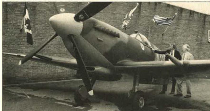
It looks like a restored Supermarine Spitfire Mk. IX, but it's not. Specialised Mouldings Ltd. has produced a limited number of glass-reinforced plastic model Spits for outside display. The planes are accurate down to the last detail.
