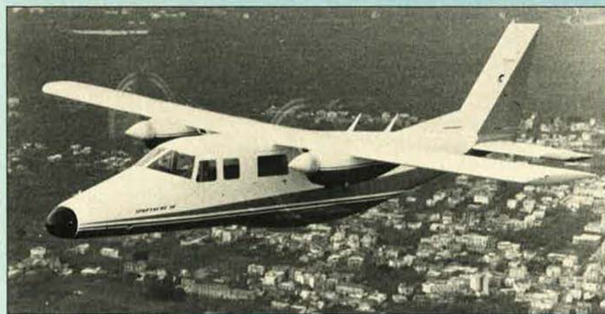
Partenavia Viator, a 'stretched' version of the Spartacus with retractable landing gear
