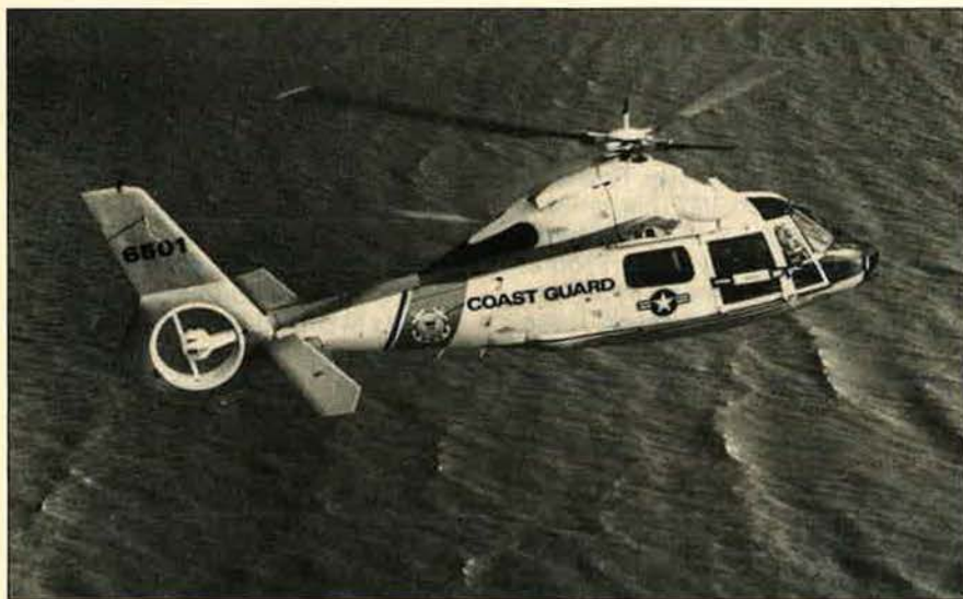
The Aérospatiale HH-65A Dolphin is the newest addition to the Coast Guard's aerial search and rescue fleet. The helicopter makes extensive use of composite materials, features advanced avionics, and has a top speed of 125 knots.
