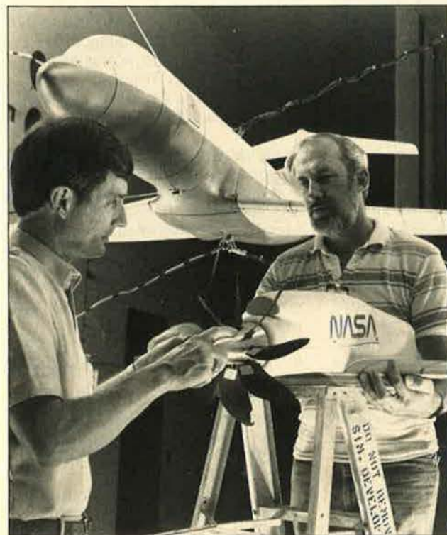
Lockheed-Georgia engineer Jerry Jenness (left) and Caltech model technician Scott McAfee prepare to adjust the configuration of the one-ninth-scale model of the Propfan Technology Assessment test-bed aircraft in the Transonic Dynamics Tunnel at NASA's Langley Research Center in Virginia. The full-scale version of the propfan and the Gulfstream II aircraft will begin testing later this year.
