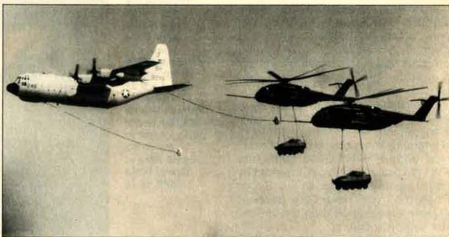
For the first time, US Marine Corps CH-53 Super Stallion helicopters have been refueled in flight while carrying Light Armored Vehicles (LAVs). The 23,000-pound LAVs are used to support amphibious and other combat operations. With in-flight refueling, the Super Stallions can provide fast LAV support from more than 100 miles behind the battle line.
