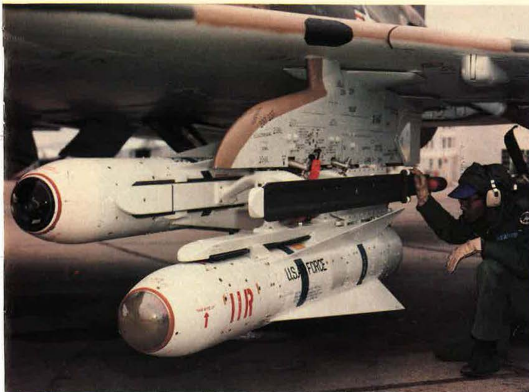
Imaging Infrared (IR) Maverick missiles are checked out prior to a test flight. The IR Mavericks performed with resounding success in tests late last year at Nellis AFB, Nev., and are now being deployed with USAF's A-10s at RAF Bentwaters, UK. A big improvement on their TV-guided predecessors, the IR Mavericks will greatly enhance the standoff capability and enrich the tactics of ground-attack aircraft.
