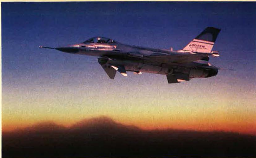
Test-bed aircraft in the Advanced Fighter Technology Integration (AFTI) F-16 program is put through its paces. Among many achievements, this program has proven out an advanced, digital, fly-by-wire flight control system that makes for major improvements in aircraft maneuverability and that is applicable to existing USAF fighters. (Photo by Erik Simonsen)
