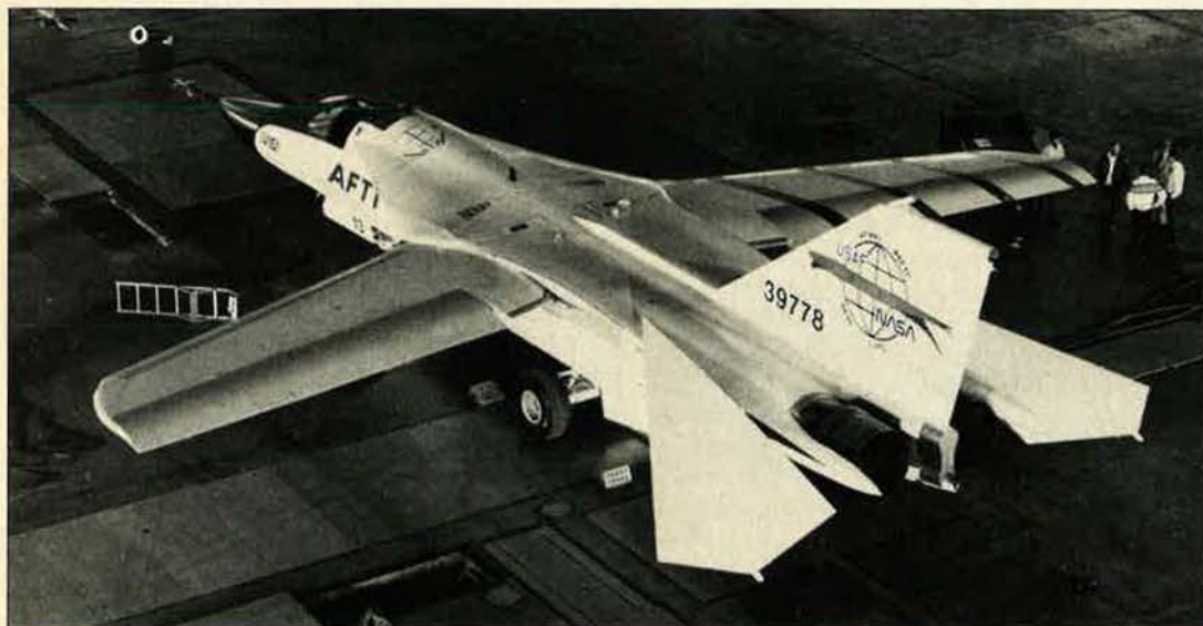
An F-111 fitted with a revolutionary new variable-camber wing is shown just before the start of an extensive, two-stage test program at Edwards AFB, Calif. The wing relies on internal hydraulic actuators and a flexible composite skin to accommodate changing flight conditions.
