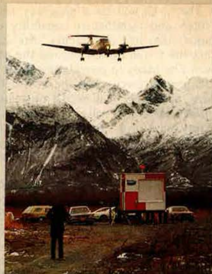
An FAA Beech King Air makes an MLS landing approach during commissioning of the MLS at Valdez, Alaska.
