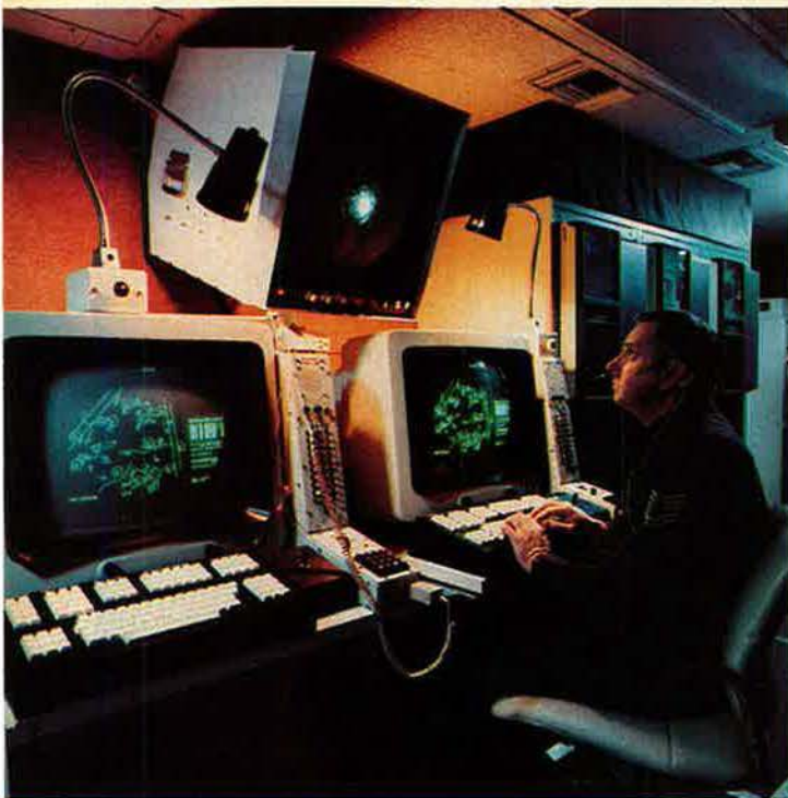
A USAF air controller works with GTE's System Trainer & Exercise Module (STEM), which duplicates actual air traffic conditions, including a radar display of up to 200 aircraft, pilot communications, and weather and terrain information. Using real aircraft to duplicate STEM's simulated workouts for controllers would entail prohibitive flying hours and costs. STEM training has a real-life feel.
