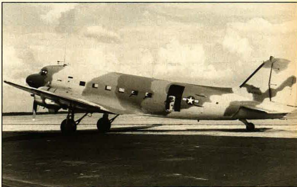
In Vietnam, the venerable Gooney Bird took on a new role and a new designation. The AC-47 Spooky mounted three side-firing 7.62-mm Gatling guns, each with a capacity of 18,000 rounds per minute, for counterinsurgency missions.
