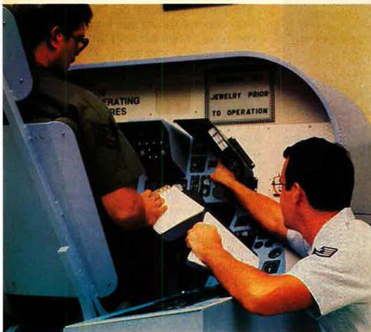
Part-task trainers, more economical than full-system simulators, are integral to both flying and ground training at Luke. This F-16 Engine Operating Procedures Trainer is used to teach crew chiefs to start, run, and check out the Fighting Falcon powerplant, with emphasis on switchology and interpretation of instrument readings.
