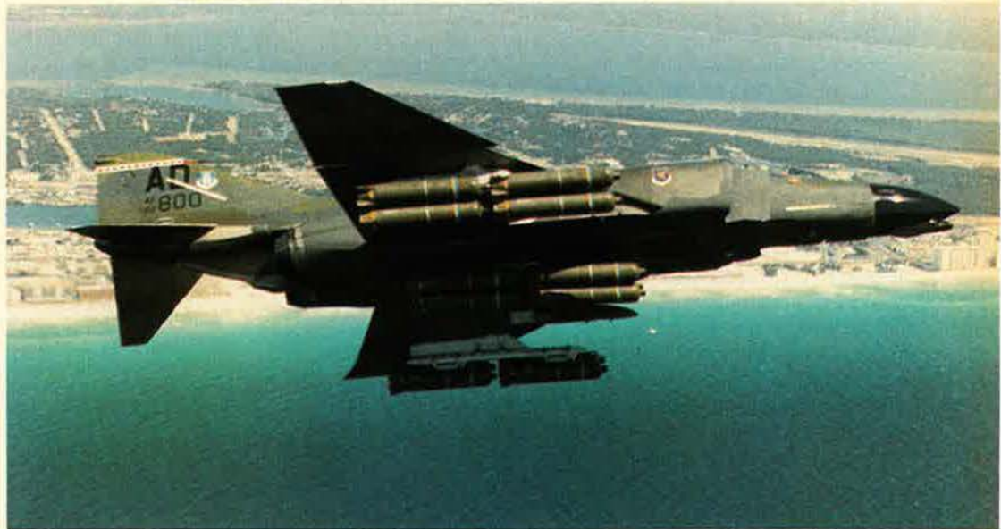
An F-4 Phantom II from Eglin AFB's Armament Division in flight tests with Gator munitions dispensers over Florida's Gulf coast. Gator is the first air-delivered scatterable mine system in the USAF inventory and can be released from a variety of aircraft.
