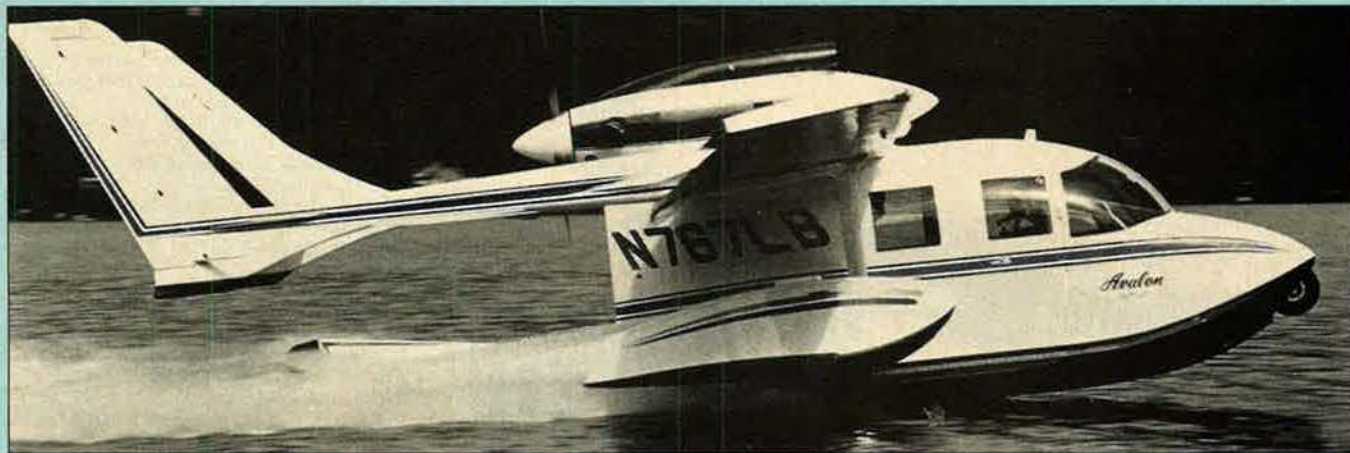
Airmaster Avalon 680 prototype (Pratt & Whitney Canada PT6A-34 turboprop engine)
