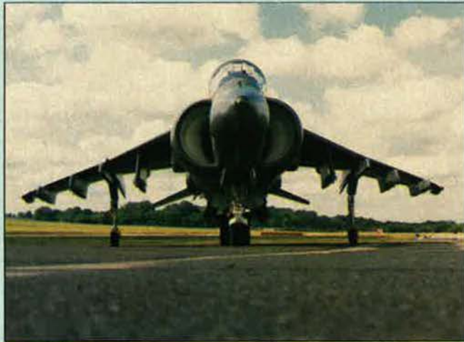
Three or four stores stations under each wing reflect the doubled payload/range of the Harrier II compared with earlier versions
