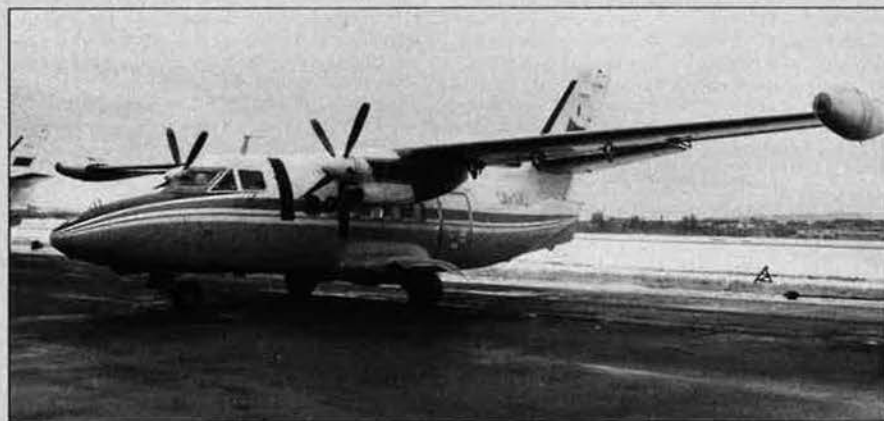
New wingtip fuel tanks distinguish the L-410UVP-E version of the Let Turbolet light transport
