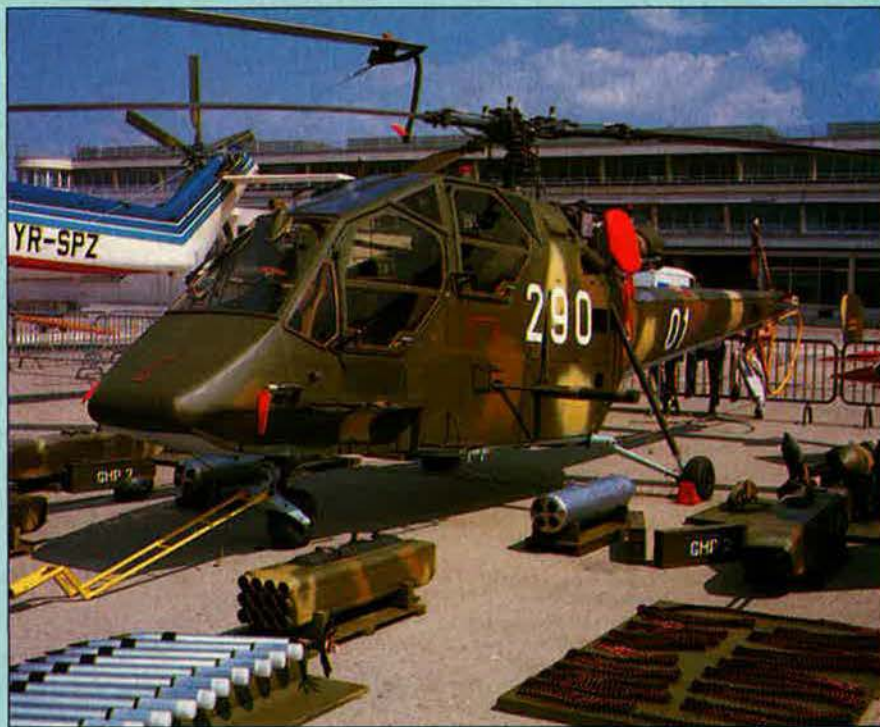
Prototype ICA IAR-317 Airfox helicopter gunship with typical weapon loads (Brian M. Service)
