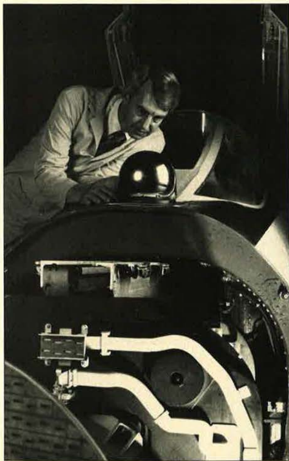
It's not a crystal ball, but an Infrared Search and Track (IRST) sensor that Hughes Radar Systems Group is proposing to "transplant" from deactivated Air Force F-101, F-102, and F-106 interceptors into Air National Guard F-4s. Giving the Air Guard this IR capability can be accomplished for one-tenth the cost of a new infrared system, Hughes says. (See item, p. 38.)
