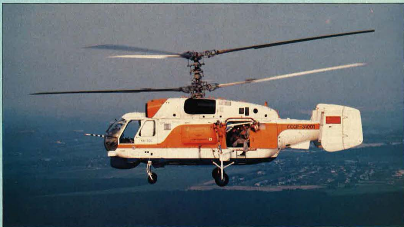
Absence of flight crew from the cockpit of this Kamov Ka-32S demonstrates their confidence in the aircraft's automatic control system
