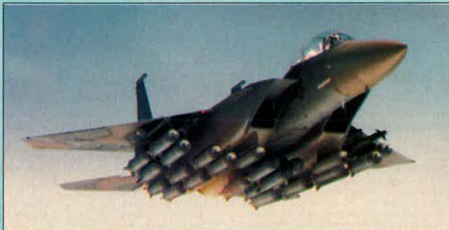
The McDonnell Douglas F-15E Eagle has a max weapon load of 10,659 kg (23,500 lb)
