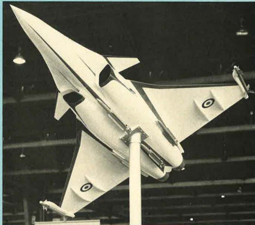
Model of Dassault-Breguet Rafale prototype at 1985 Paris Air Show. This view shows the revised engine air intakes (Brian M. Service)
