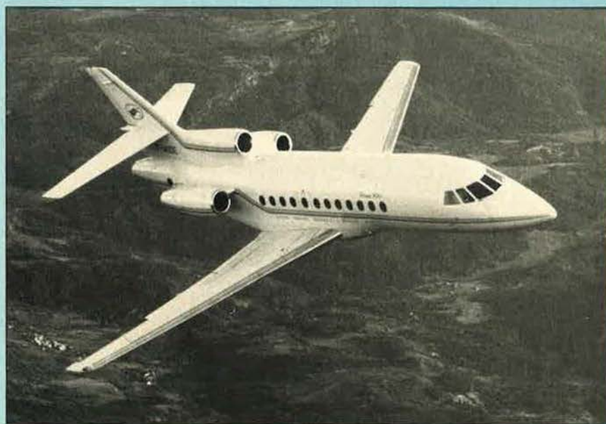
With the same three-turbofan configuration as the Falcon 50, the larger Mystère-Falcon 90 provides VIP accommodation for up to 19 passengers
