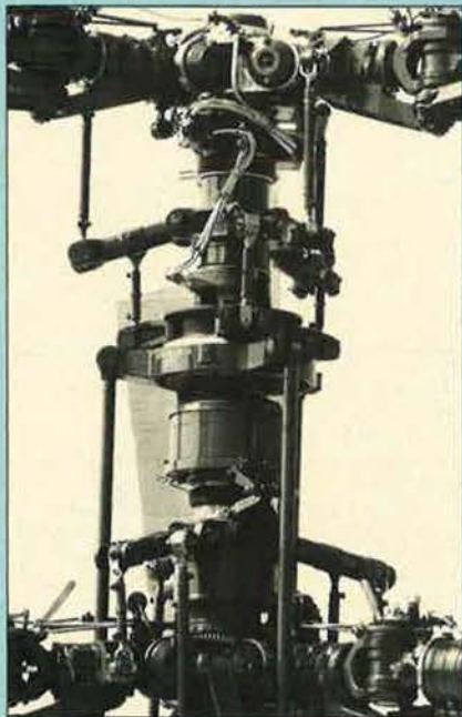
Close-up of Ka-32 rotor head (Air Portraits)
