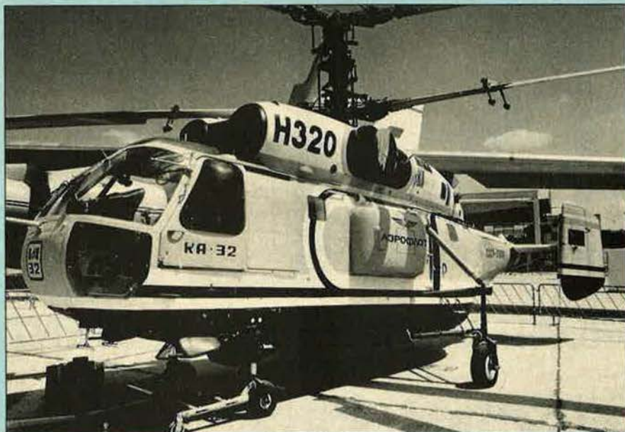
Kamov Ka-32 shown at this year's Paris Air Show was a basic transport/flying crane version of the important Ka-27 ('Helix-A') naval ASW helicopter (Brian M. Service)
