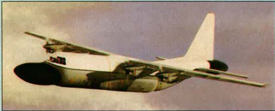
Radomes at nose and tail identify the projected AEW version of the Lockheed C-130 Hercules
