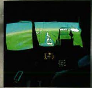
CGIVS. Computer-generated image visual system for the Tornado training simulator.
