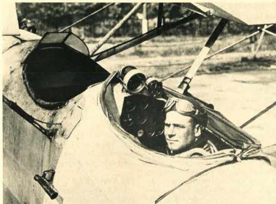
Doolittle had a special hood constructed (shown here in the down position) for the Consolidated NY-2 to ensure that the first blind flight would be made on instruments alone. Even though Doolittle made the flight with Lt. Ben Kelsey in the front seat as a safety pilot, Lieutenant Kelsey held his arms over his head to prove to ground observers that only Doolittle was at the controls.
