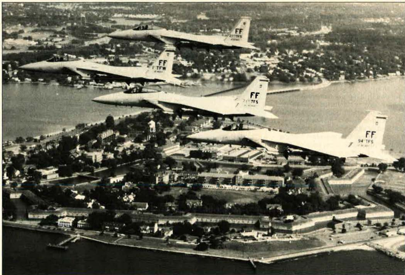
A flight of four F-15 Eagles armed with air-to-air missiles maintains close formation over historic Fort Monroe, Va., near their Langley AFB home. The Eagle recently established a fully mission capable (FMC) rate of 80.2 percent and became the safest fighter ever built, with a loss rate of only four aircraft per 100,000 flight hours.
