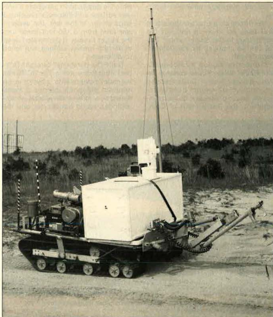
"Robbie Robot," its manipulator arm at the ready, rolls along its own tracks to the site of an unexploded warhead. This remotely controlled vehicle, about the size of a golf cart, safely retrieves unexploded munitions for analysis.
