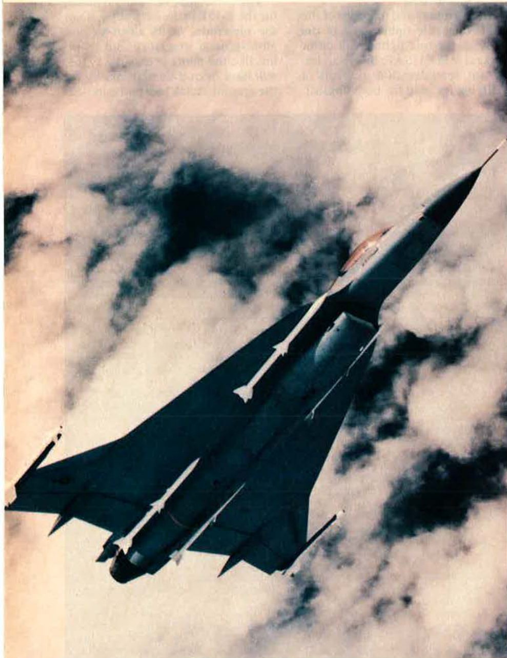
TAC has decided that its future swing-role F-16F fighter will look like this F-16XL prototype with cranked-arrow wings and a slightly longer fuselage than that of existing F-16s. TAC badly needs the launch-and-leave, multiple-engagement AMRAAM radar-guided missiles shown under the F-16XL's fuselage, along with heat-seeking Sidewinders at its wingtips.
