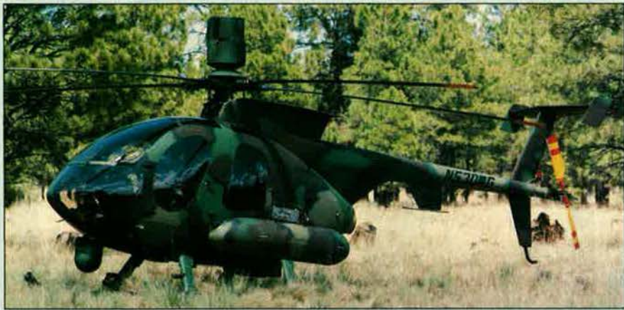
Mast mounted sight and undernose night vision system enable the Hughes Model 530MG Defender to be used for nap-of-the-earth and low-level night missions over rough terrain
