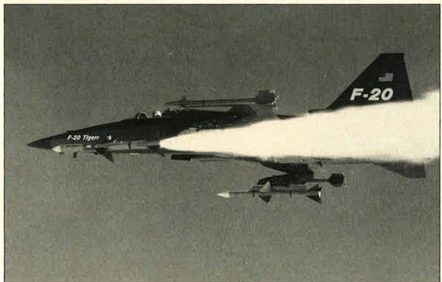
A radar-guided AIM-7F Sparrow air-to-air missile is fired from a Northrop F-20 Tigershark against an MQM-74C drone target thirteen miles away. The Sparrow, launched by USAF test pilot Maj. Doug Pearson, scored a direct hit over the ranges of the US Naval Weapons Center, China Lake, Calif. The Tigershark, which has flown more than 1,100 sorties in its flight-test program out of Edwards AFB, Calif., is carrying another Sparrow and two wingtip-mounted AIM-9 heatseekers.
