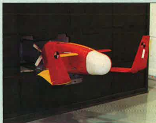
Pave Tiger emerging from launch container, with wings still partially folded
