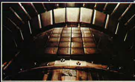
Plasma chamber protective tiles
