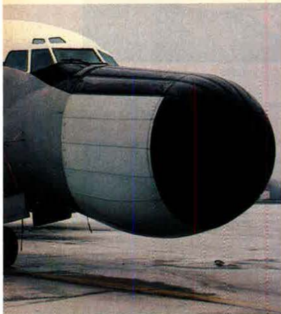
One simulator in the Crew Station Design Facility is used to train aircrews for the new EC-18B Advanced Range Instrumentation Aircraft (ARIA), which houses special mission equipment in its distinctive bulbous nose.
