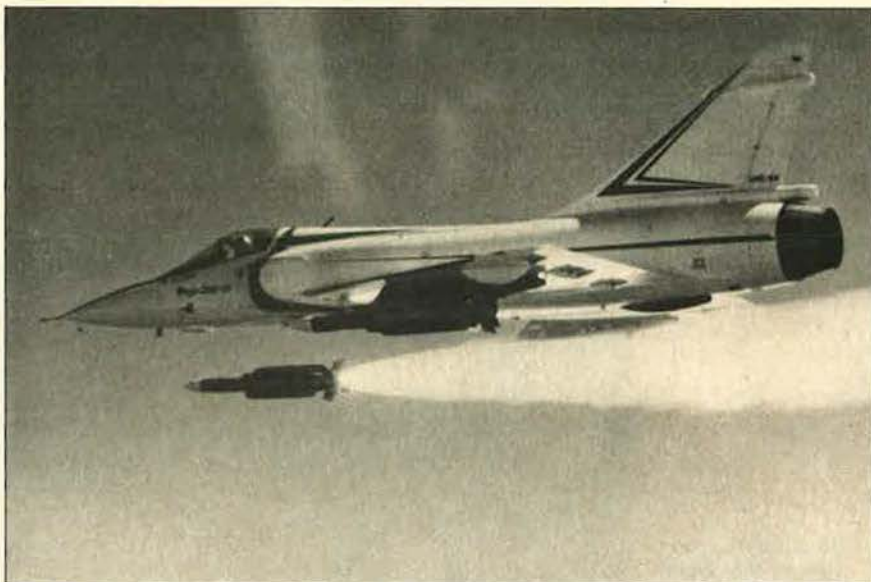
A French Mirage 2000 releases a new MATRA Super 530D long-range air-to-air missile, capable of snap-up or snap-down interceptions of targets at altitudes from the deck to 80,000 feet. It replaces the Super 530F.
