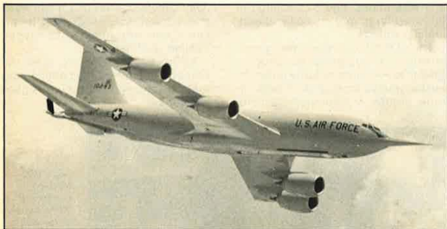
The Operational Test and Evaluation Center began testing a reengined Stratotanker—designated the KC-135R—at McConnell AFB, Kan., this past April. The aircraft's elongated nose contains a test instrumentation package. (USAF photo)
