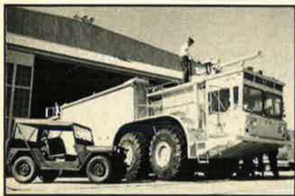
The flagship of the Air Force fire protection fleet, the P-15, packs two 430-hp diesel engines and weighs more than sixty-five tons.
