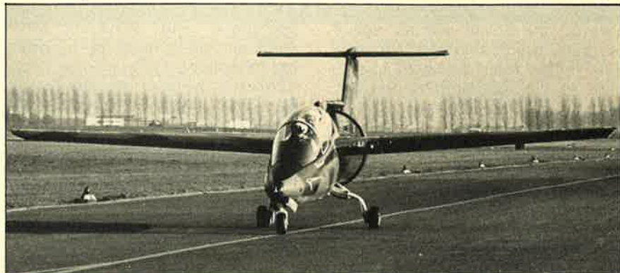
Shown airborne and on the runway is the Fantrainer, a two-seat training aircraft developed by Rhein-Flugzeugbau, a subsidiary of VFW-Fokker. Chief flight characteristic of the new plane is its novel integrated fan propulsion system provided by two rotary engines that produce a total of 300 hp. Designated the AB-2, the aircraft allows flight training at minimum cost.
