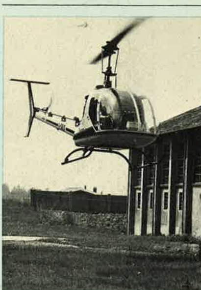
Silvercraft SH-200 two-seat light helicopter (Lycoming LHIO-360 engine)
