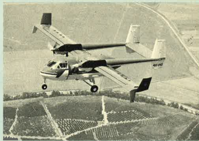
LEFT ABOVE: IAI 201 military version of the Arava, with fuselage-side gun packs and pylons for rocket launchers (Brian M. Service) RIGHT ABOVE: Prototype IAI 202 Arava, with auxiliary winglets and PT6A-36 engines
