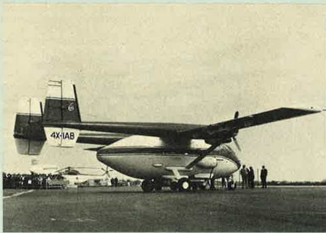
LEFT ABOVE: IAI 201 military version of the Arava, with fuselage-side gun packs and pylons for rocket launchers (Brian M. Service) RIGHT ABOVE: Prototype IAI 202 Arava, with auxiliary winglets and PT6A-36 engines
