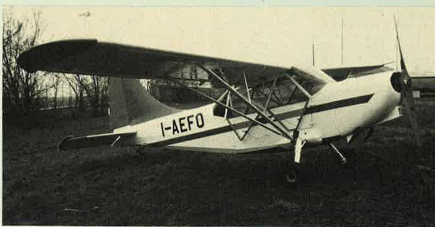
Stinson L-5 glider tug, re-engined by SSVV with a 175 kW (235 hp) Lycoming O-540
